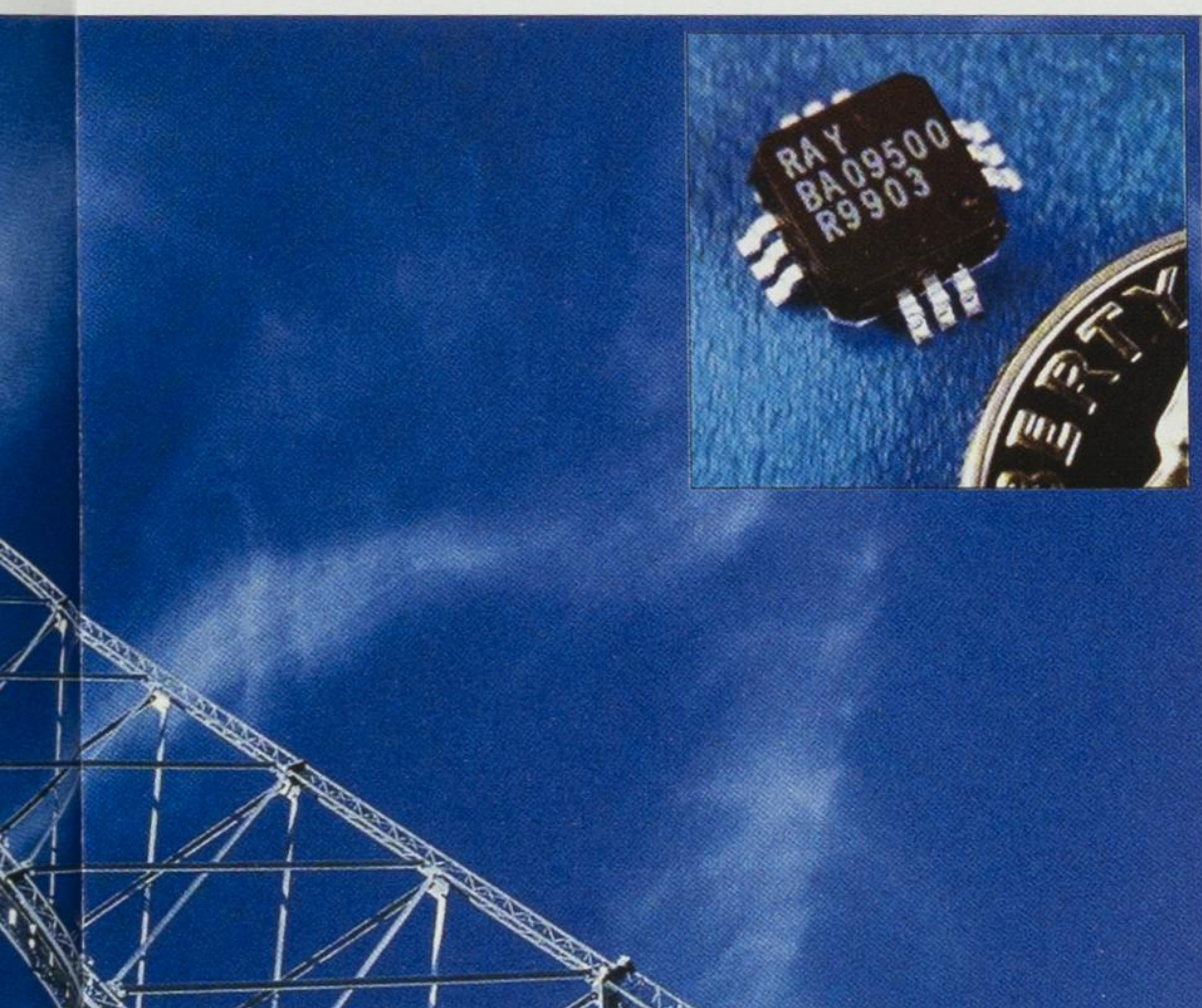
Raytheon GaAs power amplifier (inset) is a PHEMT-based MMIC used in cell base stations, and fabricated in Andover, MA.
