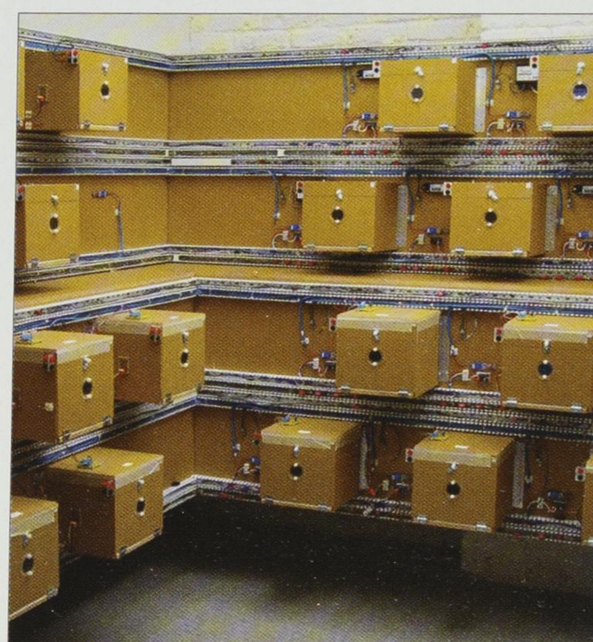
Fig. 1. Laboratory set-up at the Lighting Research Center used to measure the junction temperature and spectral characteristics of standard red and white LEDs.
