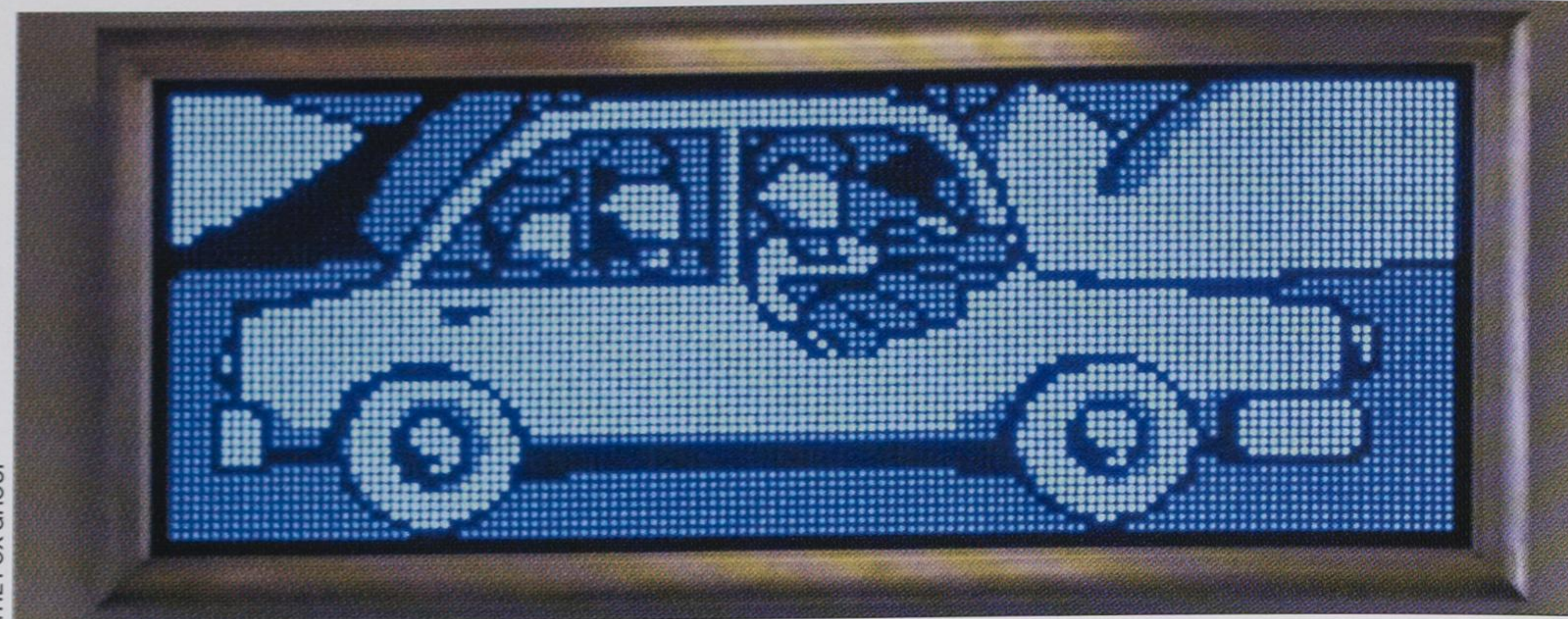
Fig. 4. Monochromatic 32 × 194 pixel sign, with dimensions of 0.45 × 1.2 m, using Fox Group's blue LEDs. The devices were not subjected to binning for color or forward voltage. Halftones were achieved by employing lower drive currents.
