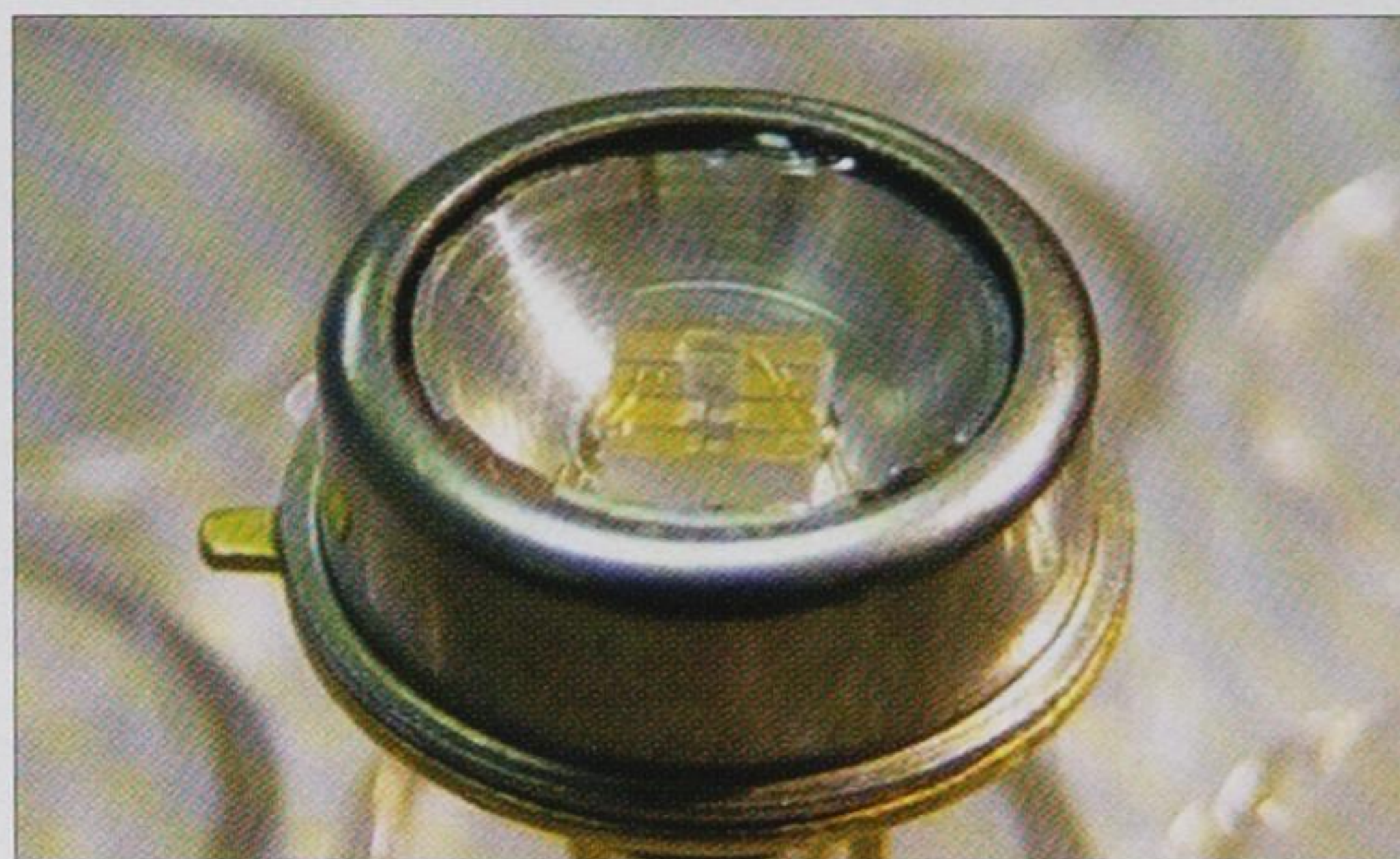
Fig. 1. Sensor Electronic Technology's UVTOP-340 LED is the first commercially available UV LED with peak emission at 340 nm, and is designed for biological and chemical sensor applications.
