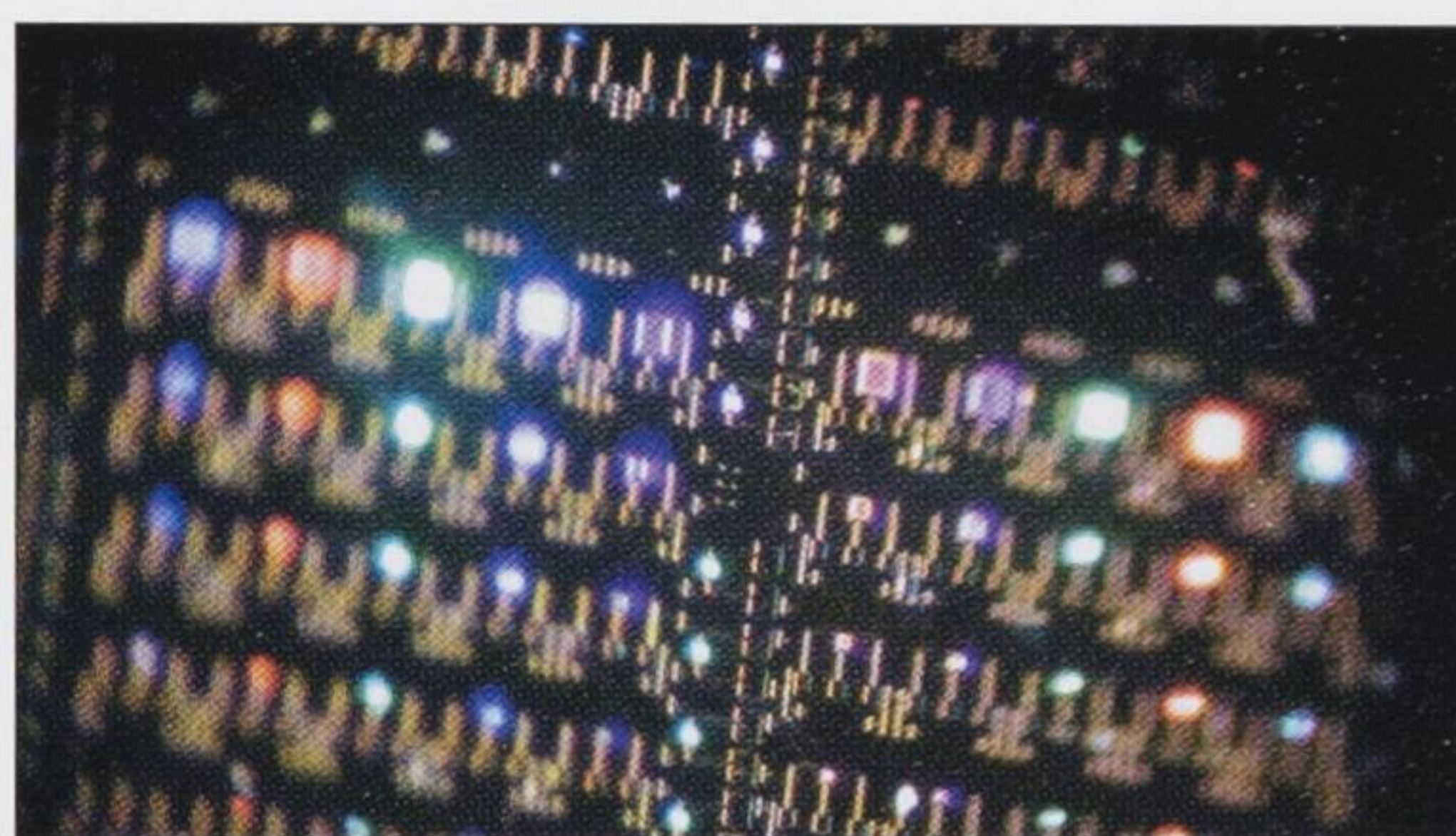
Fig. 3. An optical micrograph of an array of GeOI photodetectors. The active areas appear colored when held at an angle to the illuminating light because the interdigitated fingers of the devices are of a similar size to visible wavelengths. The detectors at the top of the photograph are 100 \mu\text{m} wide, while those at the bottom measure just 10 \mu\text{m} .
