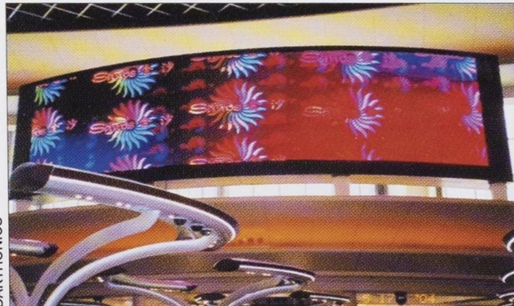
This 22 ft high by 82 ft long casino display in China features 1.7 million LEDs p6
