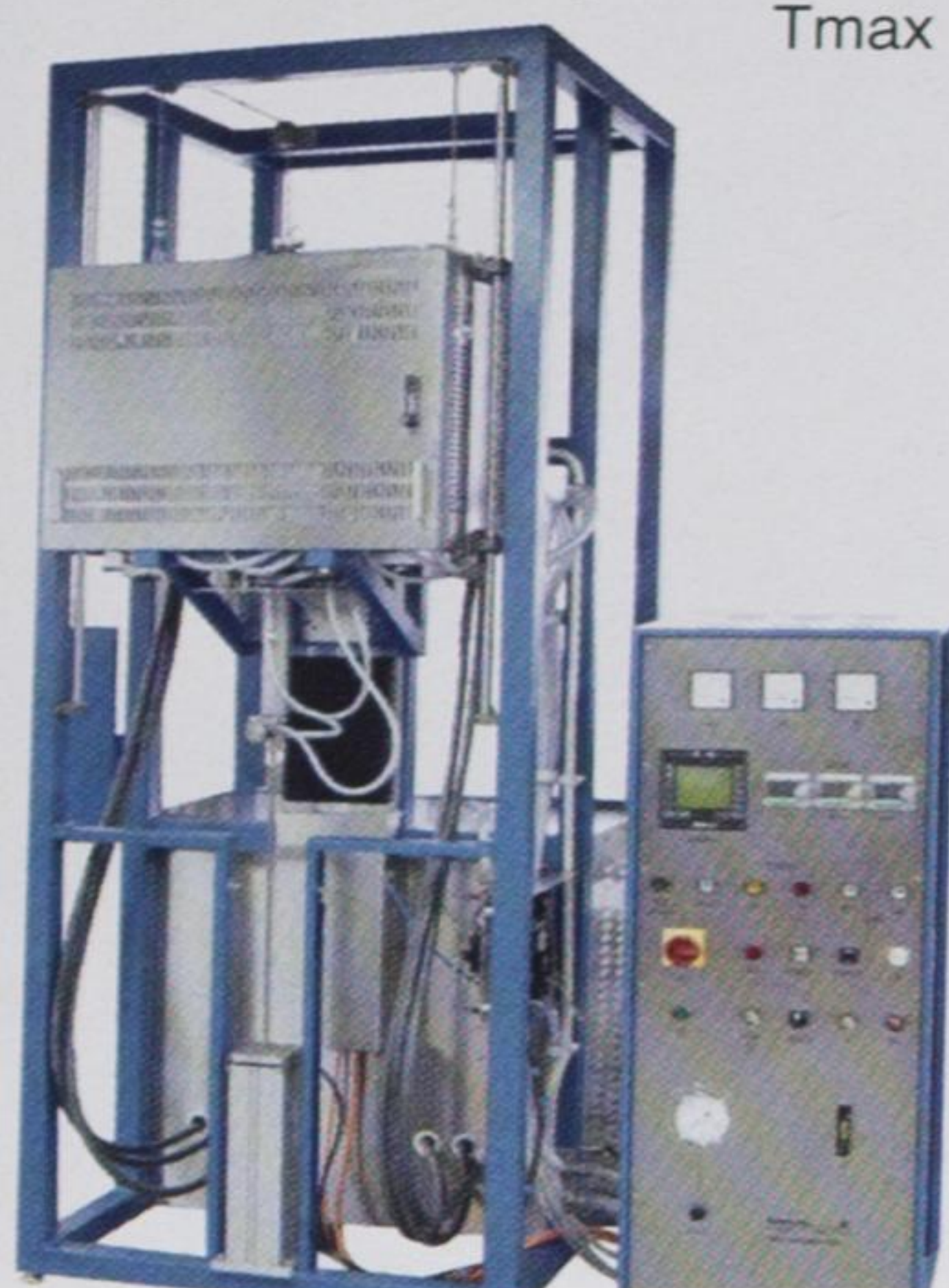
Bridgeman 3 zone vertical tubular furnace with graphite heater for directional / and single crystal solidification of metals under protective gas atmosphere. With quenching baffle. High precision translation. Program controller: SE 502. Max. furnace temperature: 1.800 °C. Max. heating power: appr. 20 kW. Linear unit: 0,1 mm/h to 1.000 mm/h. Fast cooling: appr. 100 mm/s.
