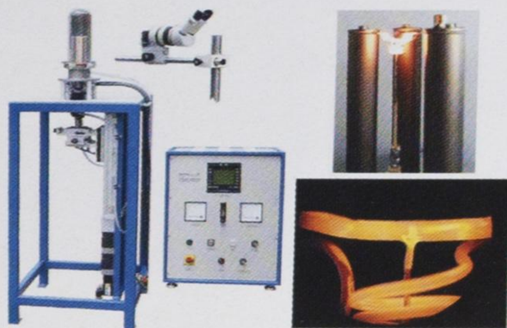
Micro-Crystal growth system for pulling of single crystalline fibers from the melt under inert gas or air. Fiber dimensions: \varnothing = 0,2-2,0 mm, l_{max} = 250 mm. Up to 5000 mg of starting material is melted in a platinum crucible (for high-melting compounds also Ir-, W-, Mo- crucibles) and a fiber crystal is pulled down through a capillary nozzle with a secondary heater around the nozzle. Power supply: primary heater 80 W (max. 500 W), secondary heater 30 W (max. 200 W).
