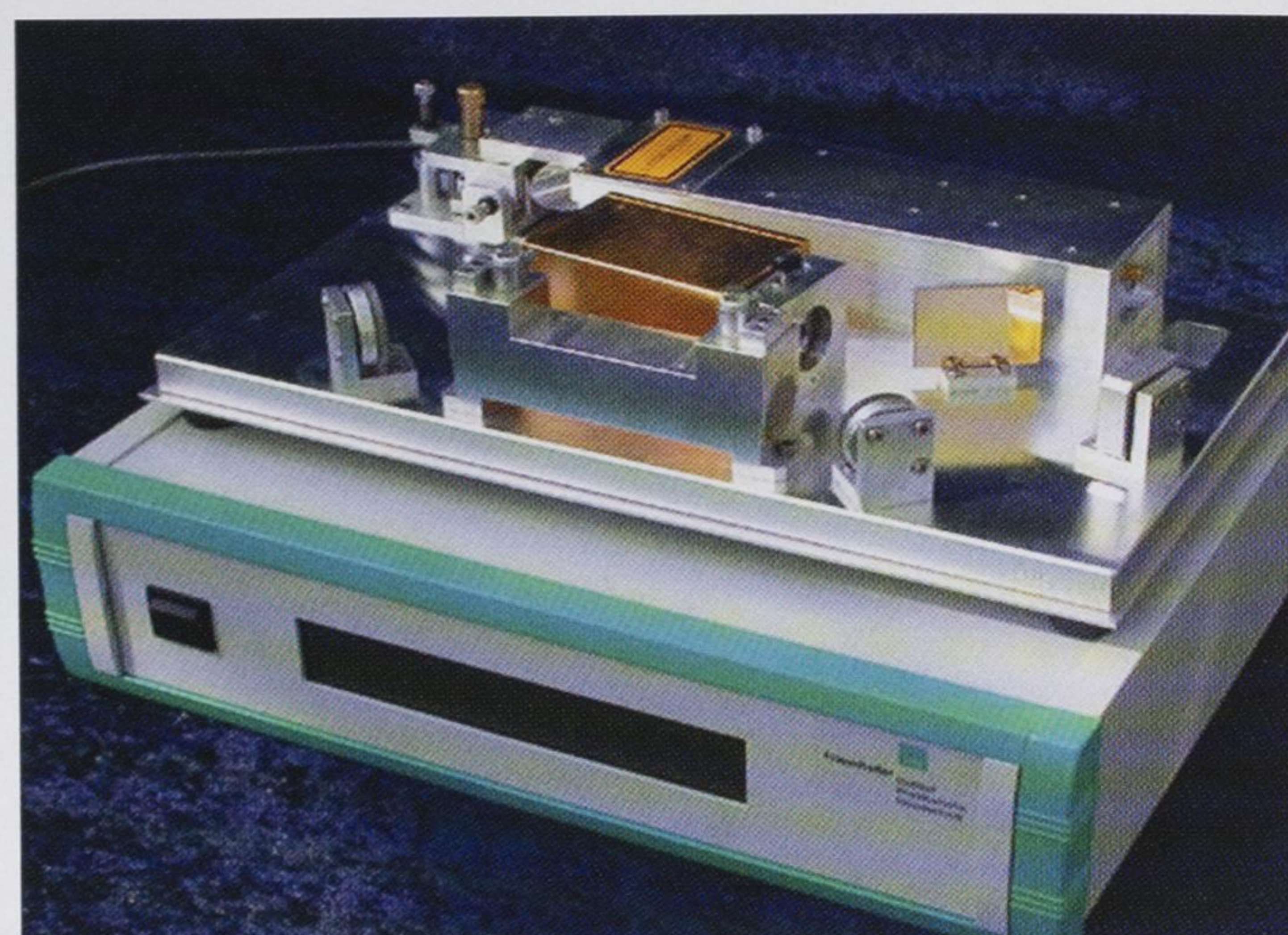
Fig. 2. Fraunhofer Institut Physikalische Messtechnik's QCL system detects various gases including \text{NH}_3 , \text{CO}_2 and \text{NO} .
