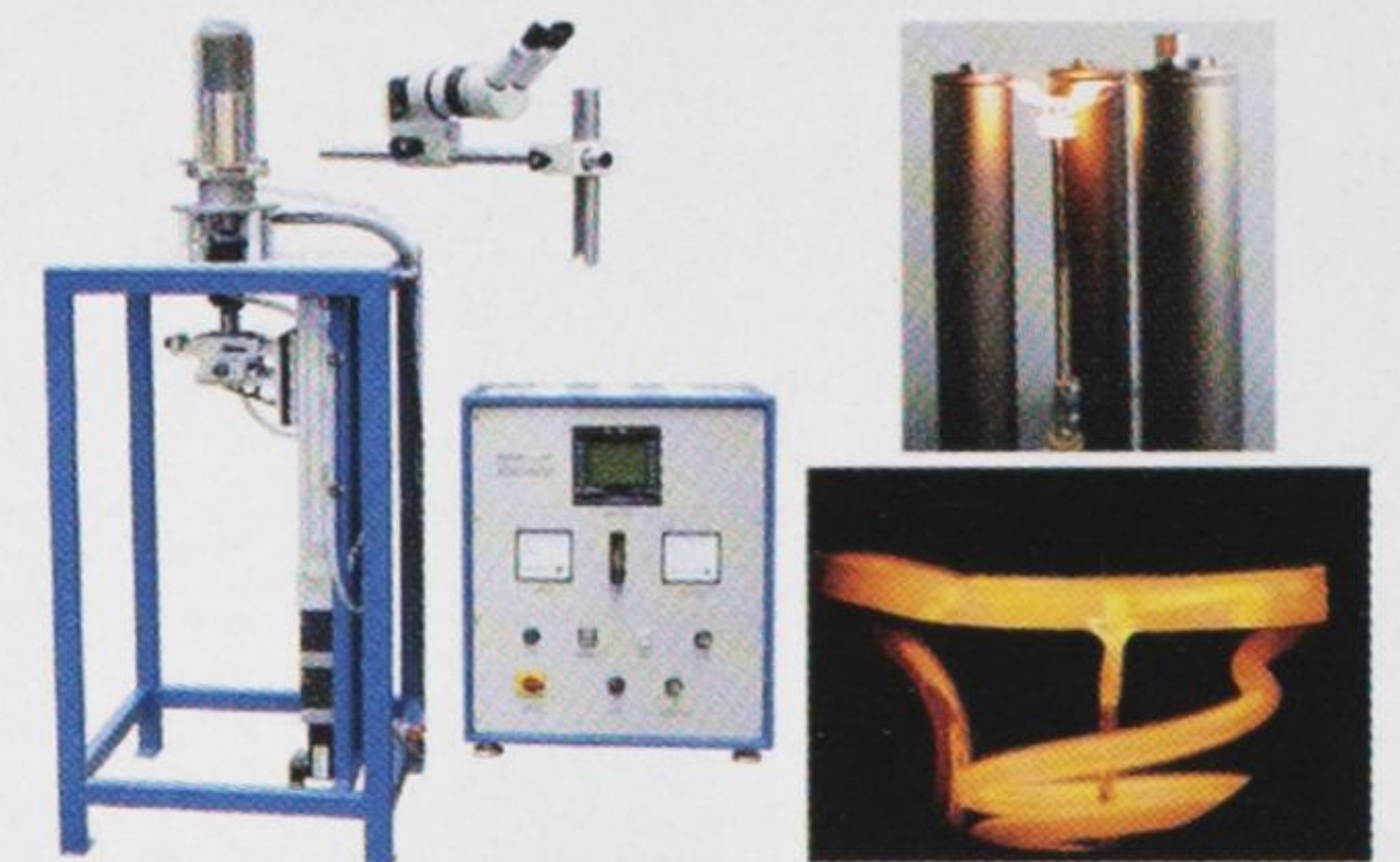
Micro-Crystal growth system for pulling of single crystalline fibers from the melt under inert gas or air. Fiber dimensions: Ø = 0,2-2,0 mm, l max = 250 mm. Up to 5000 mg of starting material is melted in a platinum crucible (for high-melting compounds also Ir-, W-, Mo- crucibles) and a fiber crystal is pulled down through a capillary nozzle with a secondary heater around the nozzle. Power supply: primary heater 80 W (max. 500 W), secondary heater 30 W (max. 200 W).
