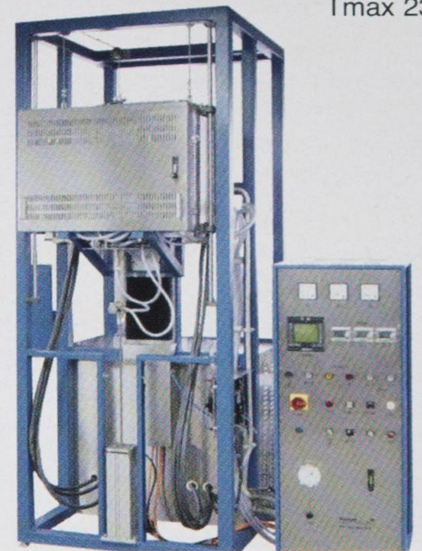
Bridgman 3 zone vertical tubular furnace with graphite heater for directional / and single crystal solidification of metals under protective gas atmosphere. With quenching baffle. High precision translation. Program controller: SE 502. Max. furnace temperature: 1.800 °C. Max. heating power: appr. 20 kW. Linear unit: 0,1 mm/h to 1.000 mm/h. Fast cooling: appr. 100 mm/s.
