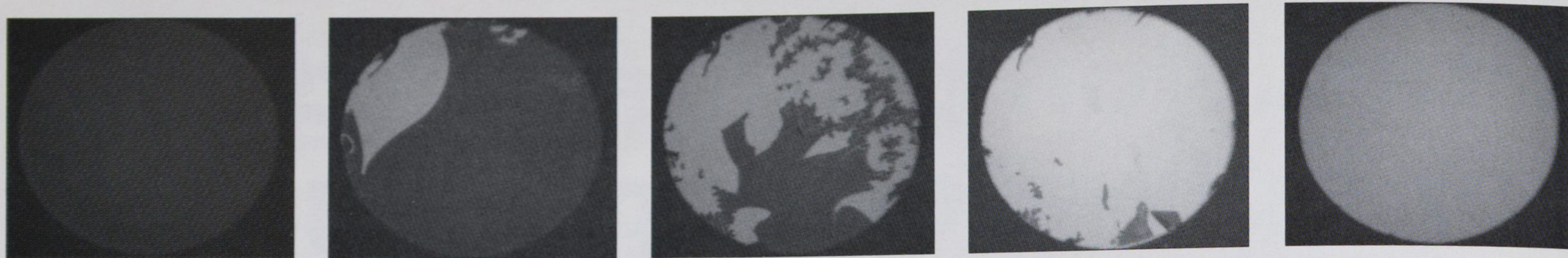
Fig. 4. The ECV profiler can be used to analyze distributed-Bragg-reflector structures with an etch flatness of about 5 nm. Sequential images recorded by the in situ camera monitor the effective oxide film removal while etching through an AlGaAs/GaAs interface.
