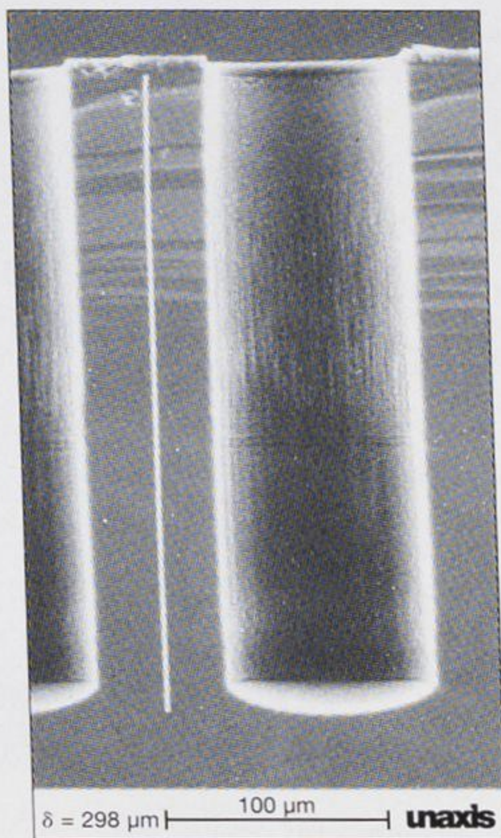
300 µm deep silicon via etched with DSE™
