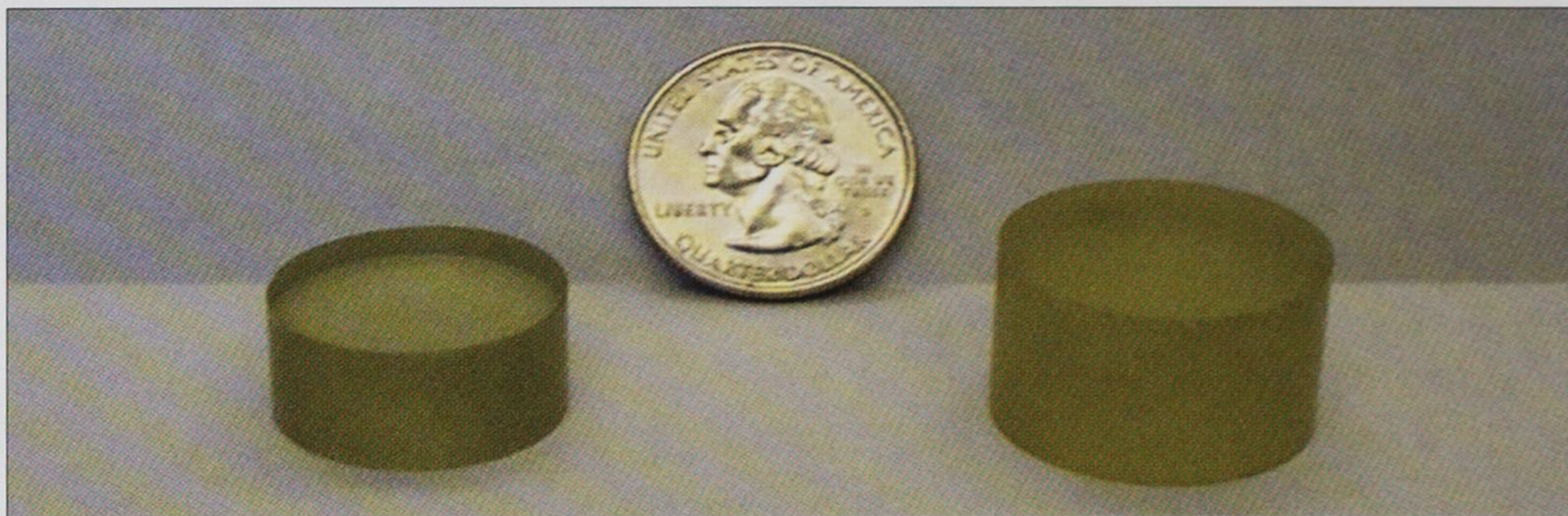
Fig. 1. Cermet has produced these ZnO substrates with a range of dopants to induce self-fluorescence. Eventually, this could lead to the fabrication of high-efficiency, phosphorless white LEDs. With a defect density of only 1 \times 10^4 \text{ cm}^{-2} , the lattice-matched InGaN that has been grown on this ZnO should result in high-performance nitride devices.
