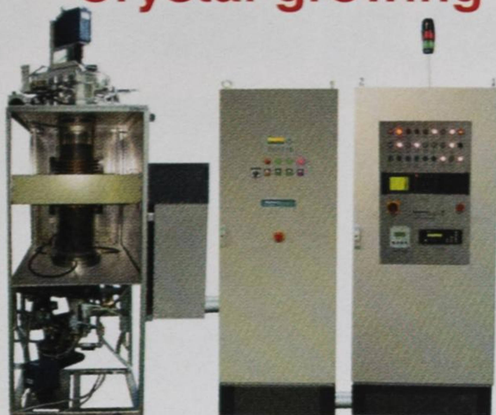
Production system for sublimation growth of 2 / 3 inch 4H- and 6H SiC single crystals for optoelectronics, power- and high temperature electronics. Allows the precise control of process conditions (temperature field, gas pressure, gas composition). Tmax 2300 °C.
