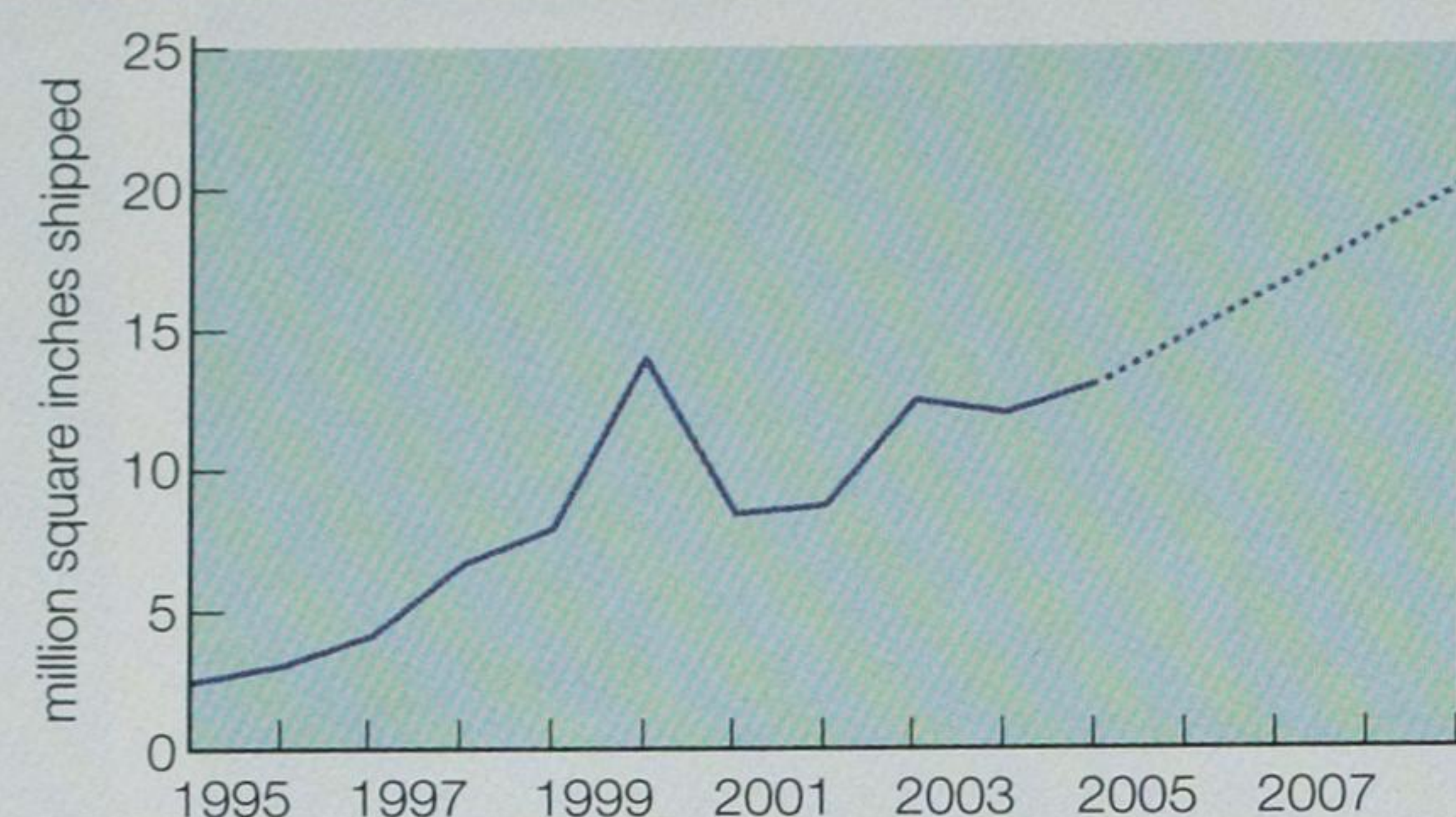
GaAs markets 1995–2009: substrate shipments (right) have mirrored fluctuations in the device market.
