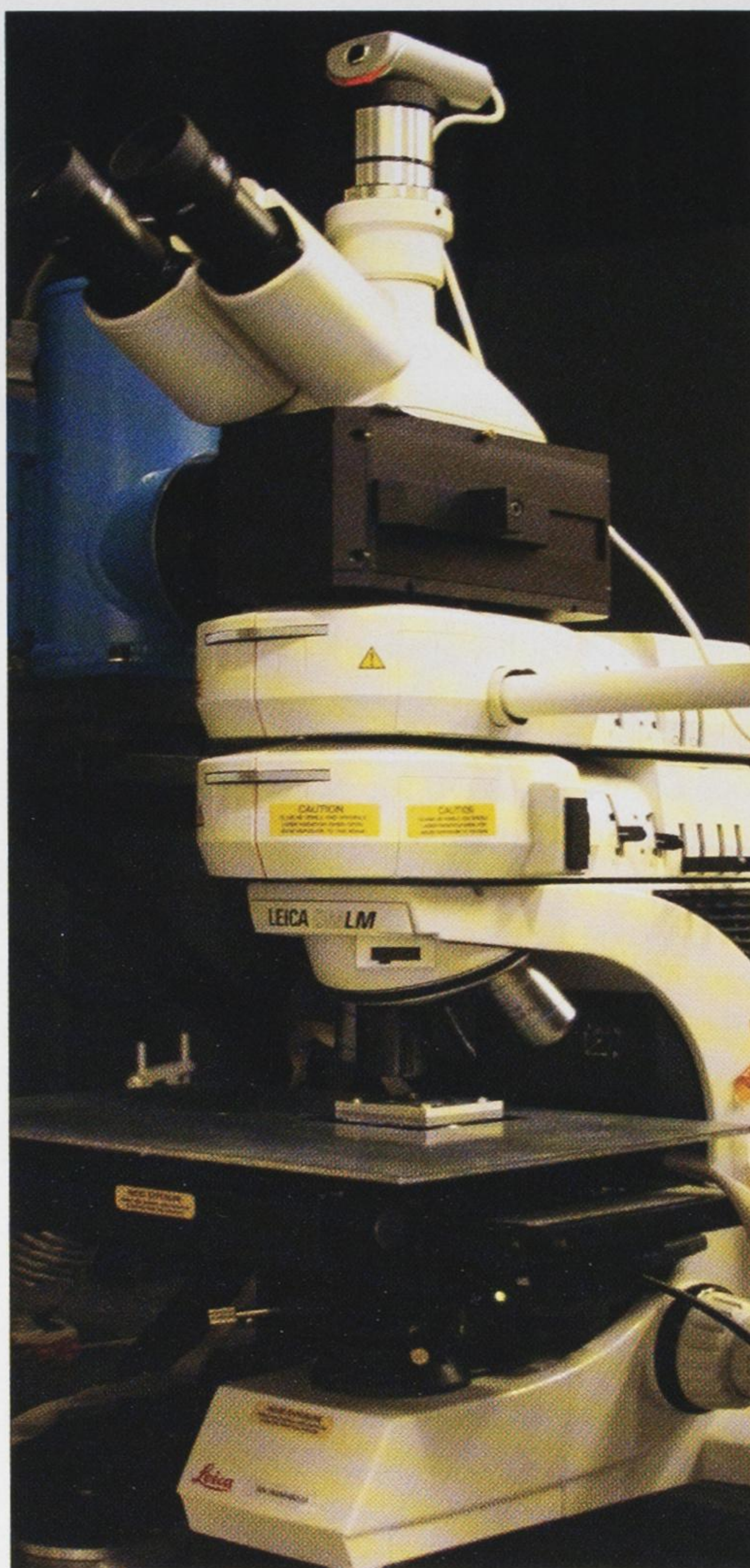
Fig. 1. The integrated Raman spectroscopy and infrared thermography system (left) combines the best of both techniques to allow investigation of micrometer-scale local heating in AlGaIn/GaN HFETs (above).
