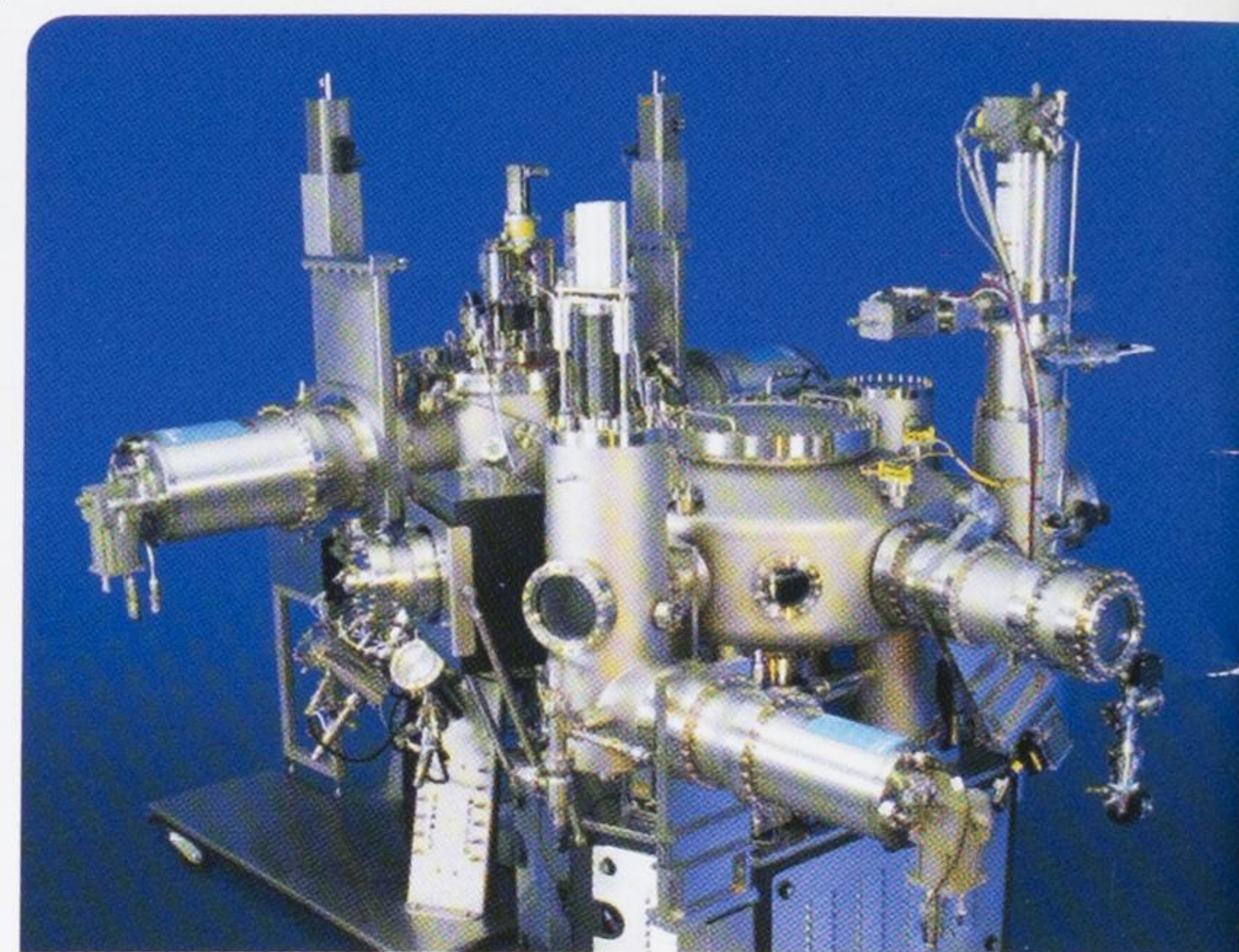
Photo of Veeco Silicon-Style Cluster Tool.
