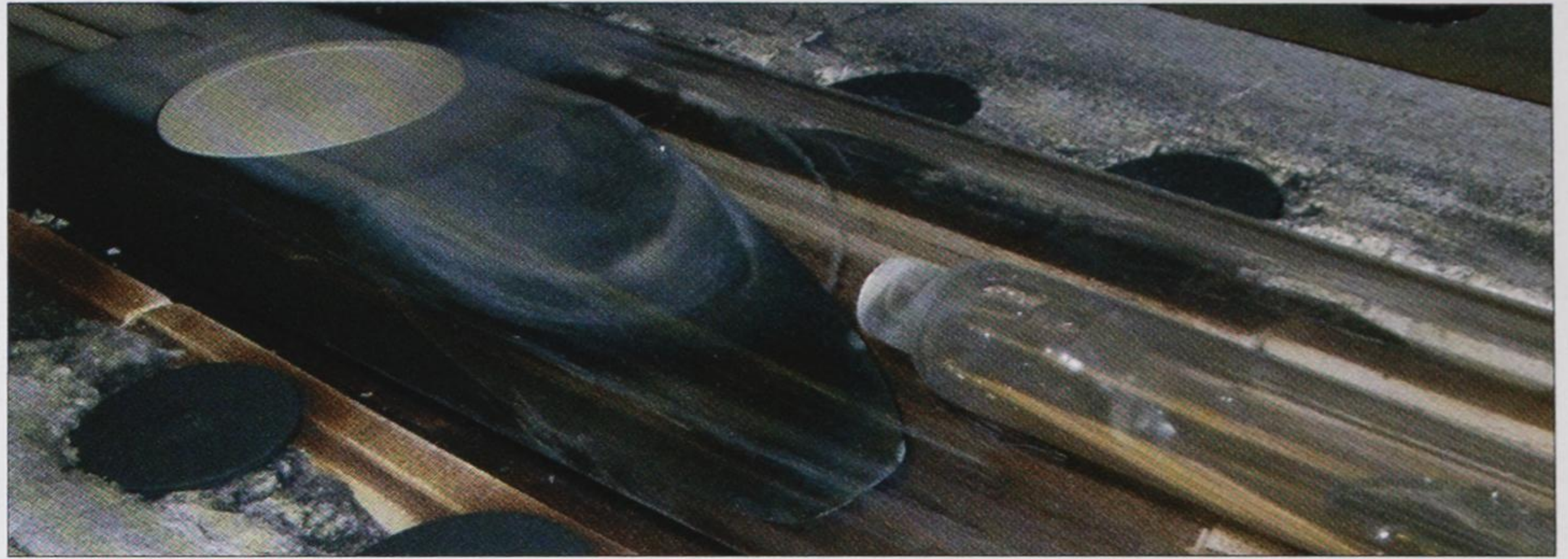
Combining the strengths of HVPE and MOVPE allows high-quality GaN films to be grown on sapphire substrates in a single process. This horizontal gas-flow reactor features a raised platform for the substrate, and carrier and process gases that are introduced from the right-hand side. Independent heating of the substrate holder and reactor walls provides suitable conditions for both types of growth process.
