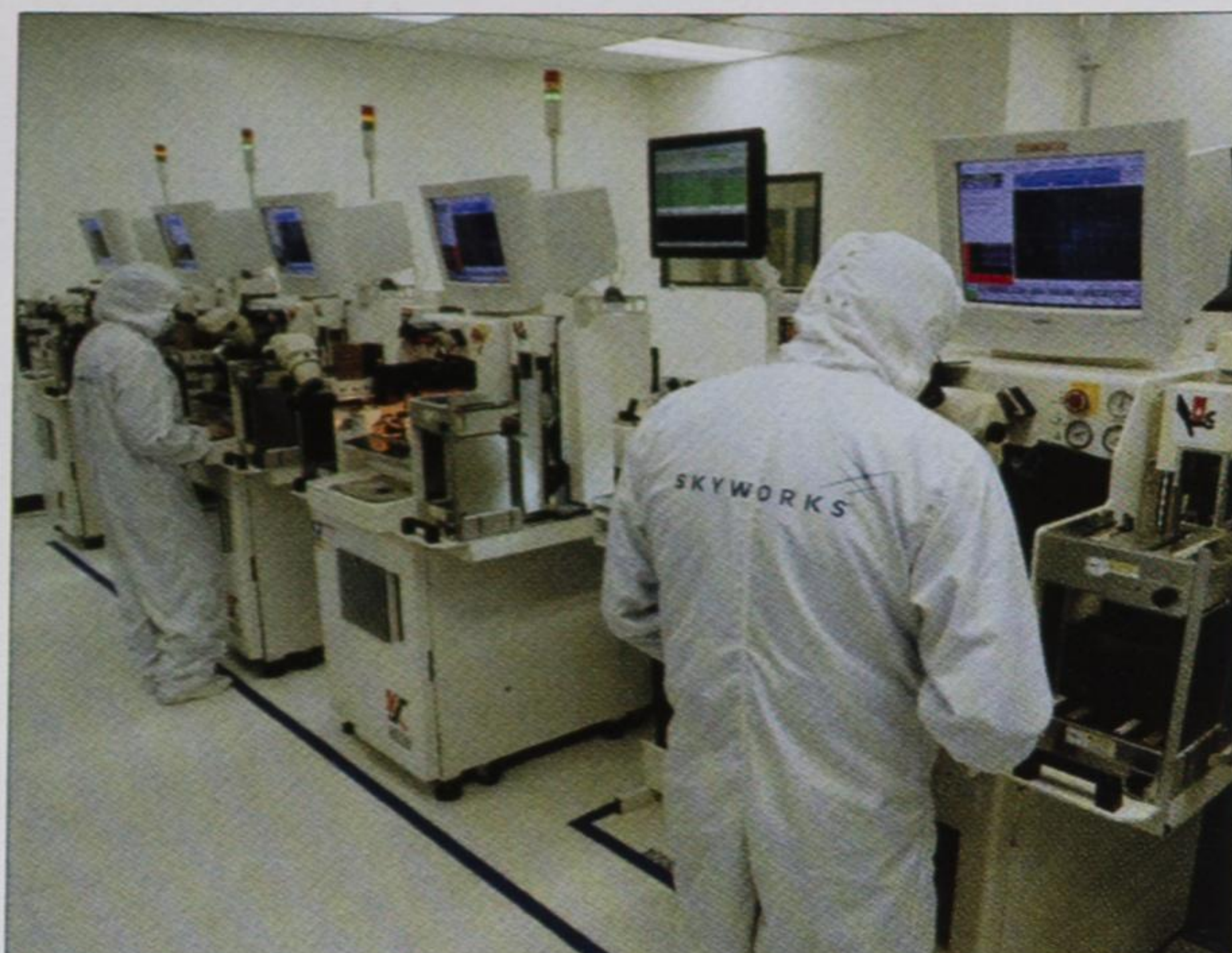
Wirebonders in the cleanroom area of Skyworks' back-end facility in Mexicali, Mexico. The company operates two GaAs fabs, one in Newbury Park, CA, where HBTs and BiFETs are produced, and another in Woburn, MA, for PHEMT and MESFET manufacture.
