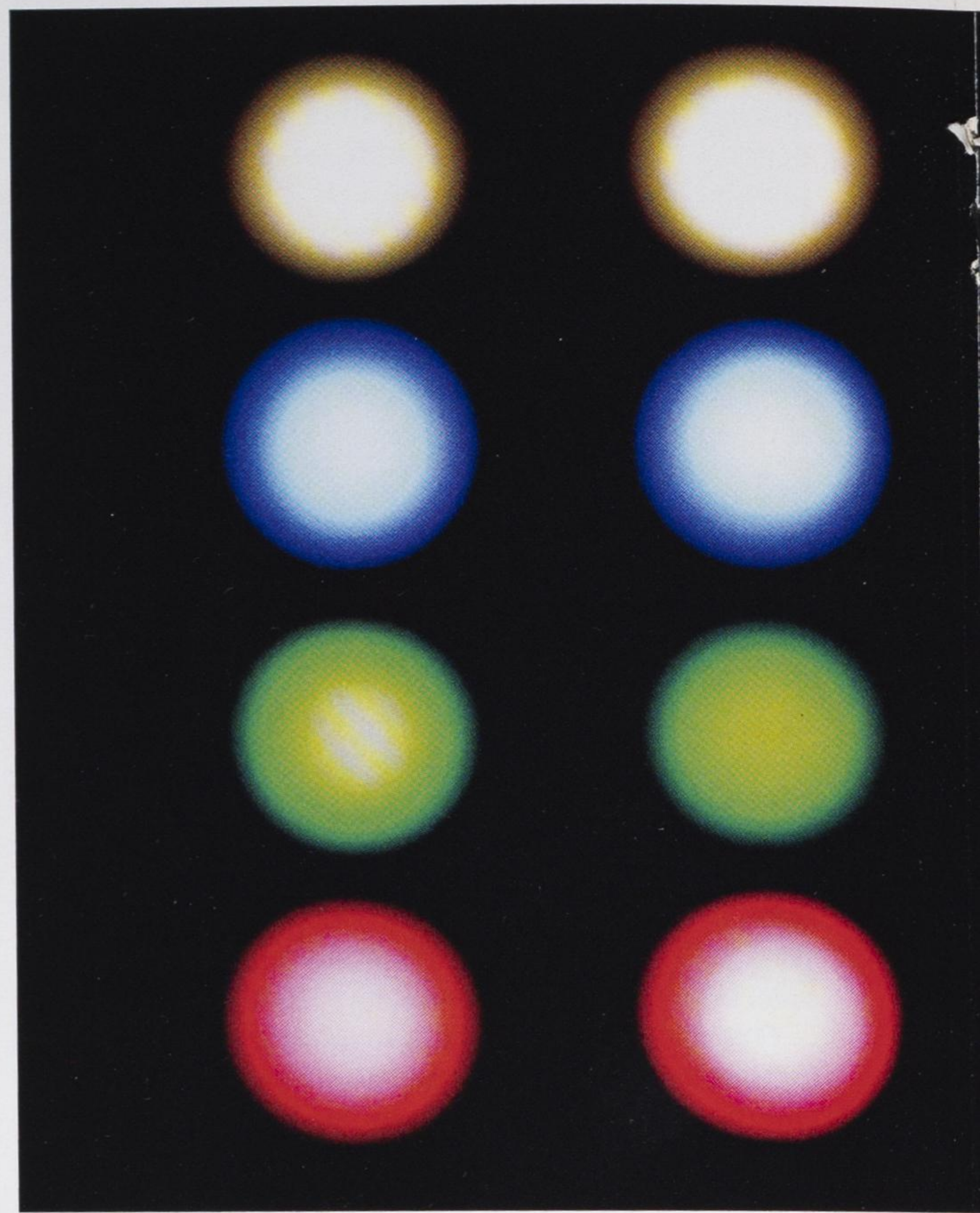
MOXtronics has recently produced the first-ever ZnO-based LEDs emitting in the development of ZnO-based materials, such as the alloys CdO, CdSe and CdS, could
