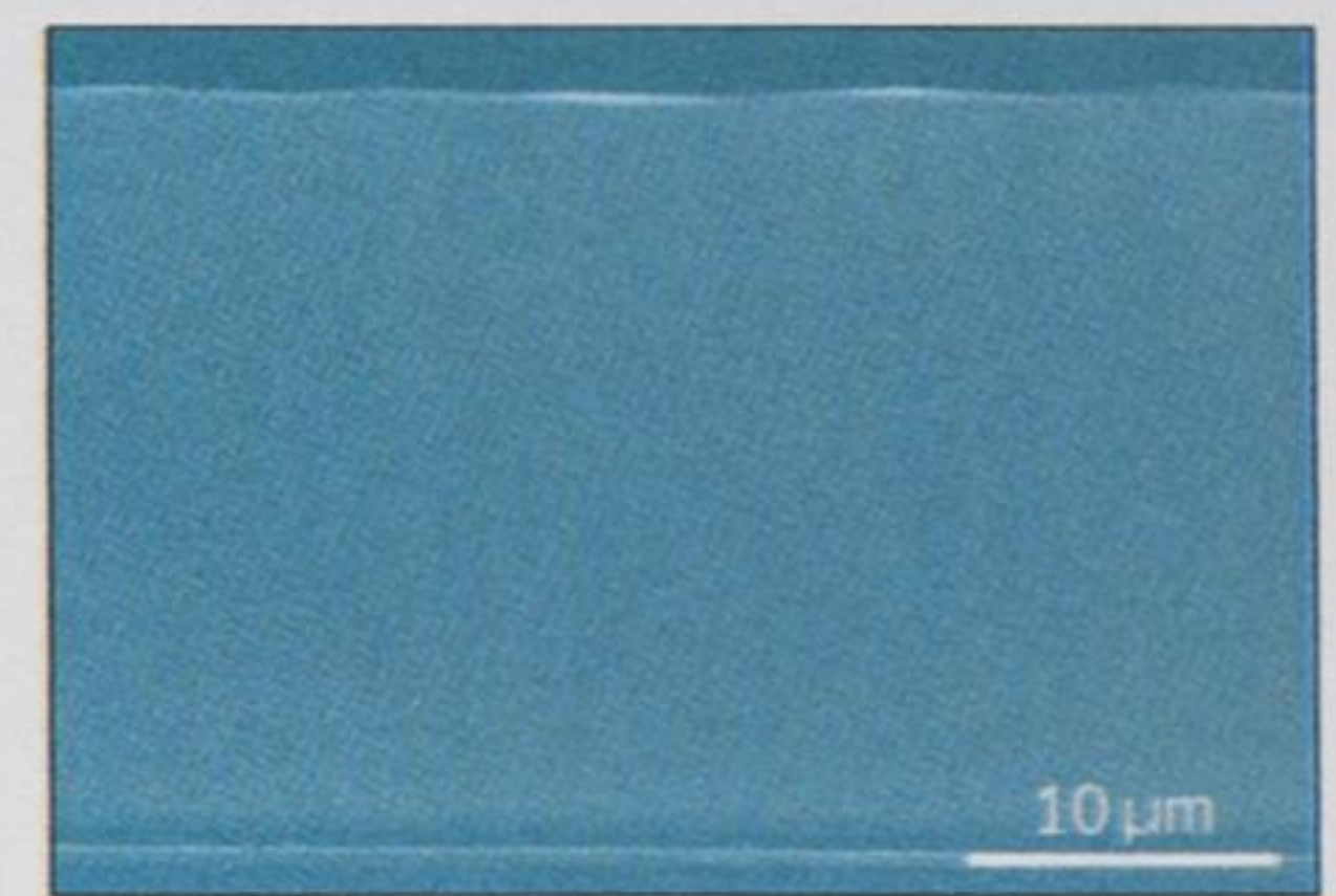
The cleaved edge of an AlN-on-SiC epitaxial wafer with a 26 \mu\text{m} -thick AlN layer, showing that it is possible to grow crack-free AlN using TDI's stress-control HVPE process.
