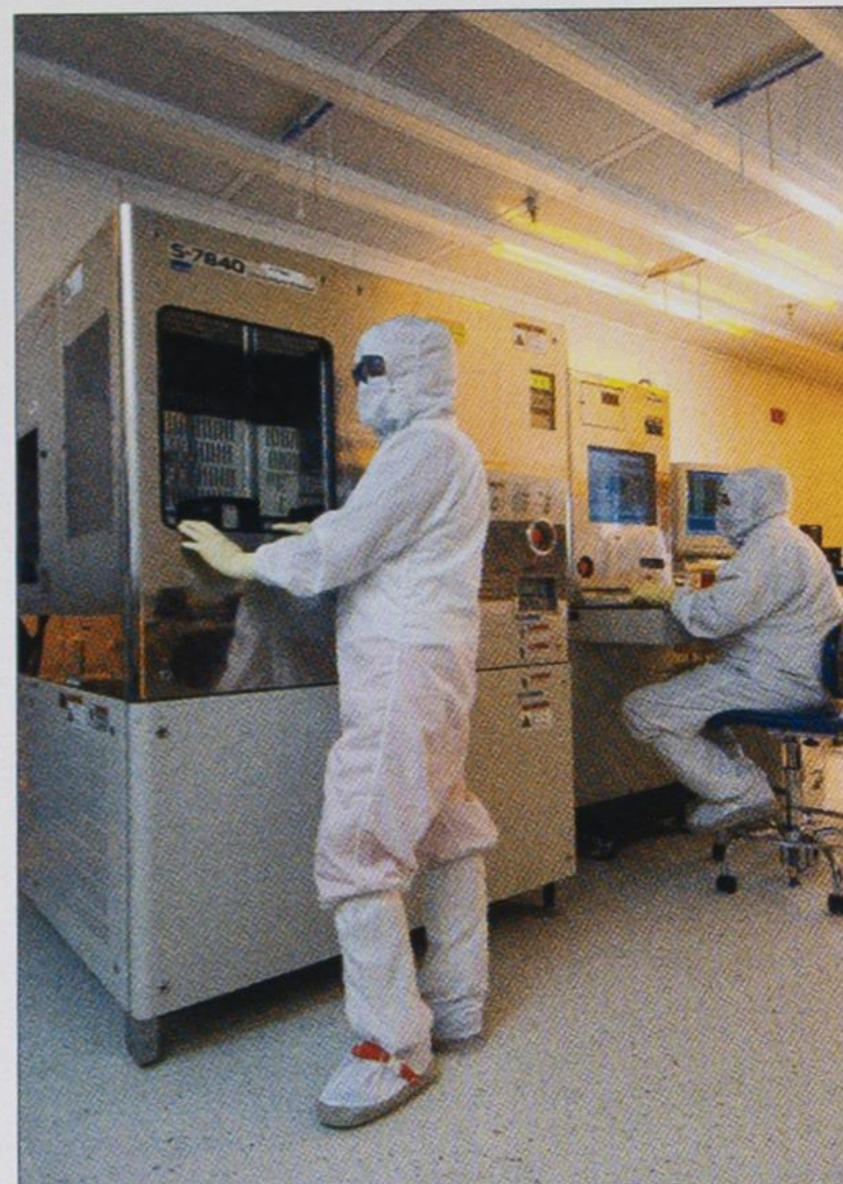
Despite the advanced material being processed there, Cree's new SiC power and RF device facility is much like any GaAs or silicon fab. It features a bay of I-line lithography steppers (left), an inspection station with scanning electron microscopes (center) and an electron beam metal-evaporation system (right).
