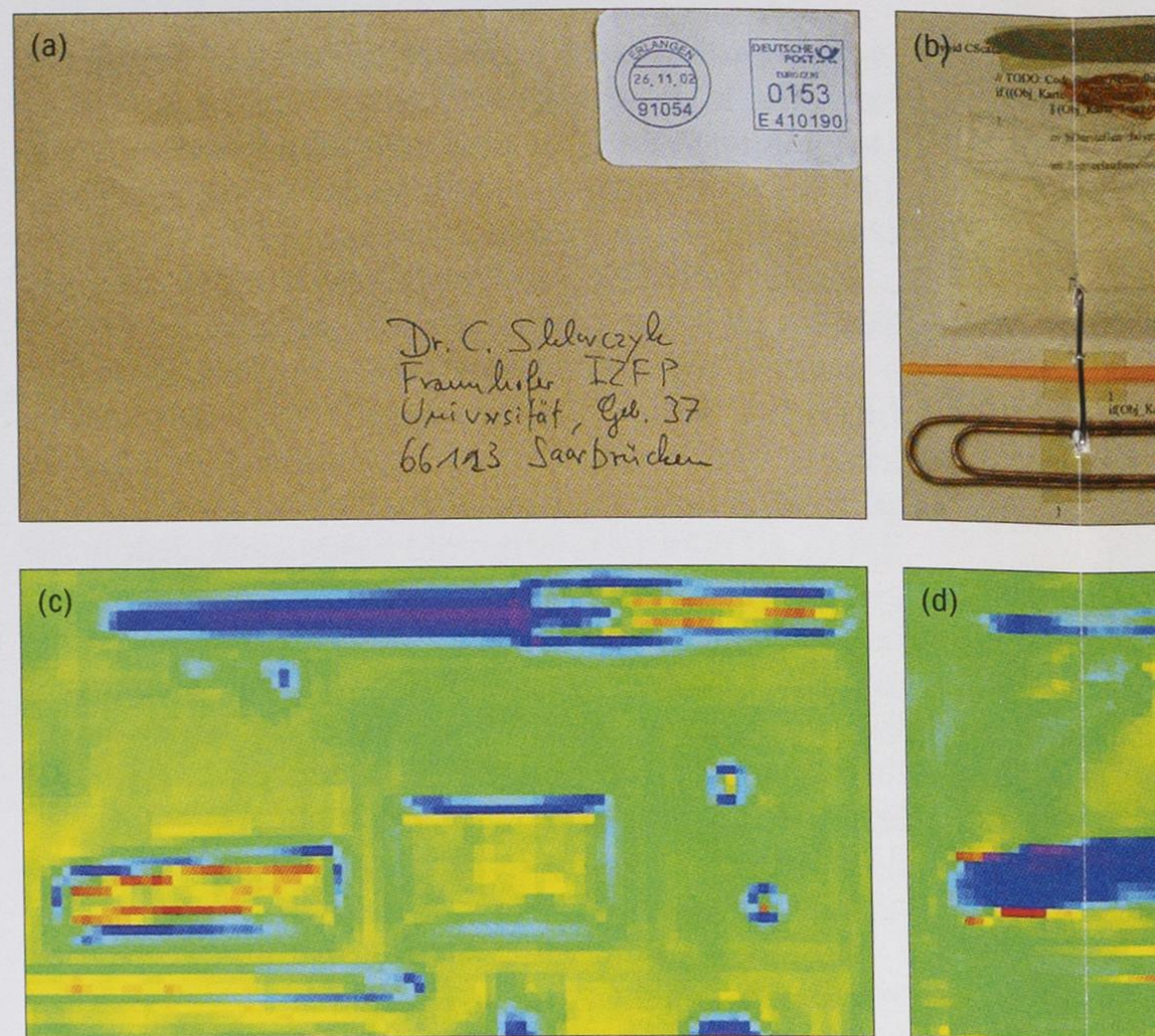
Fig. 1. Substances that are now banned on flights can be exposed by active millimeter-wave imaging. (a) hides a nail file, sugar, artificial sweeteners, cocktail needle, copper wire and paper clip. (b) shows a paperclip. (c) and (d) are amplitude (c) and phase (d) images produced at Fraunhofer IZPF, a partner of Fraunhofer IAF.
