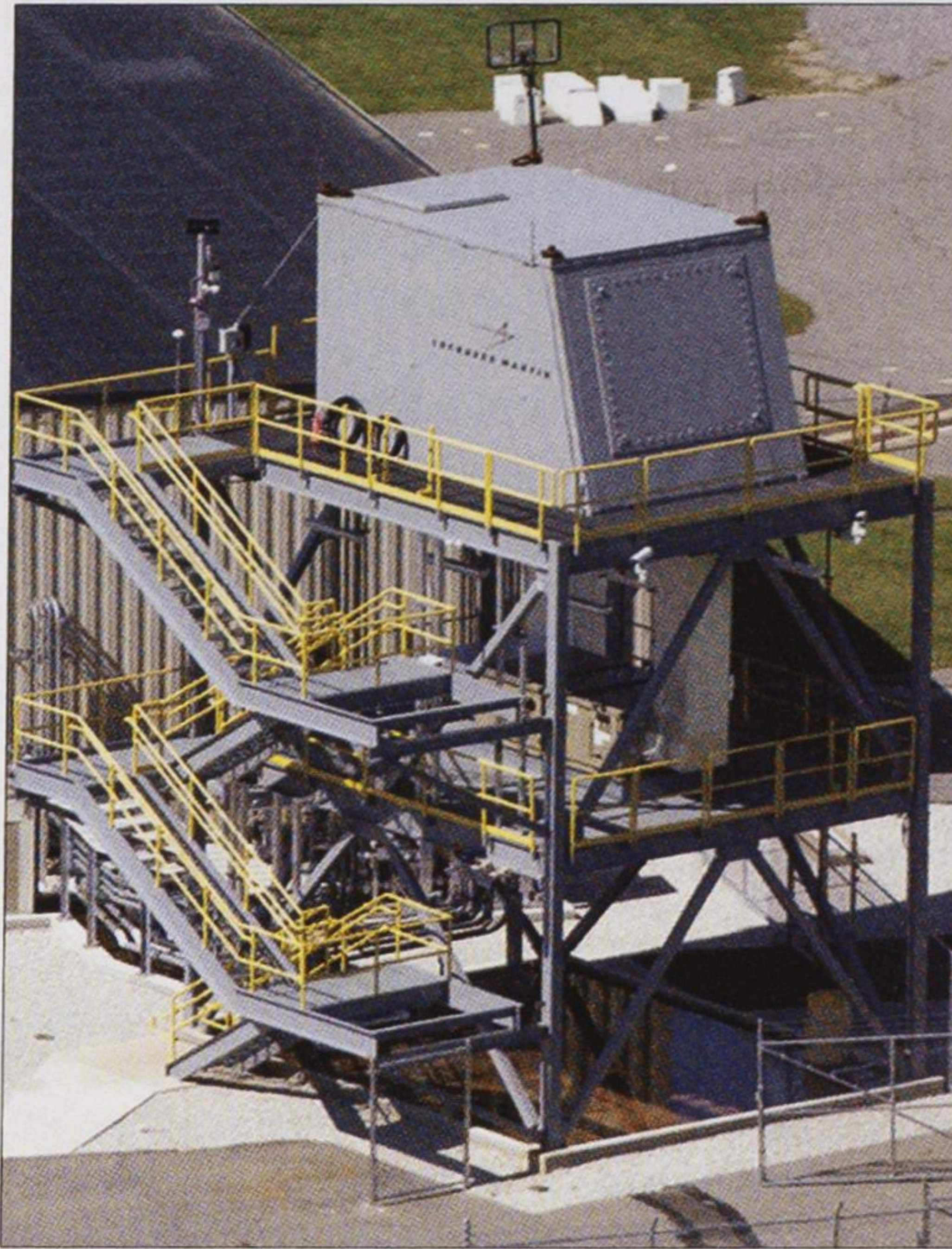
Powered up: Developed for the US military, Lockheed-Martin's scalable solid-state S-band radar is the first SiC-based system to perform live aircraft tracking.
