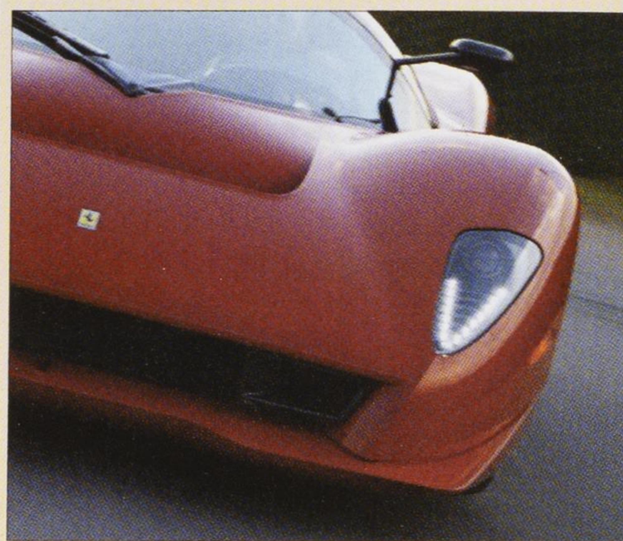
Automotive design specialist Pininfarina used 15 lighting clusters, each fitted with eight Power TopLEDs supplied by Osram Opto Semiconductors, to create daytime running lights in the headlamps of this Ferrari P4/5. Each LED is equipped with a ThinGaN chip, providing an efficiency of 40 lm/W.
