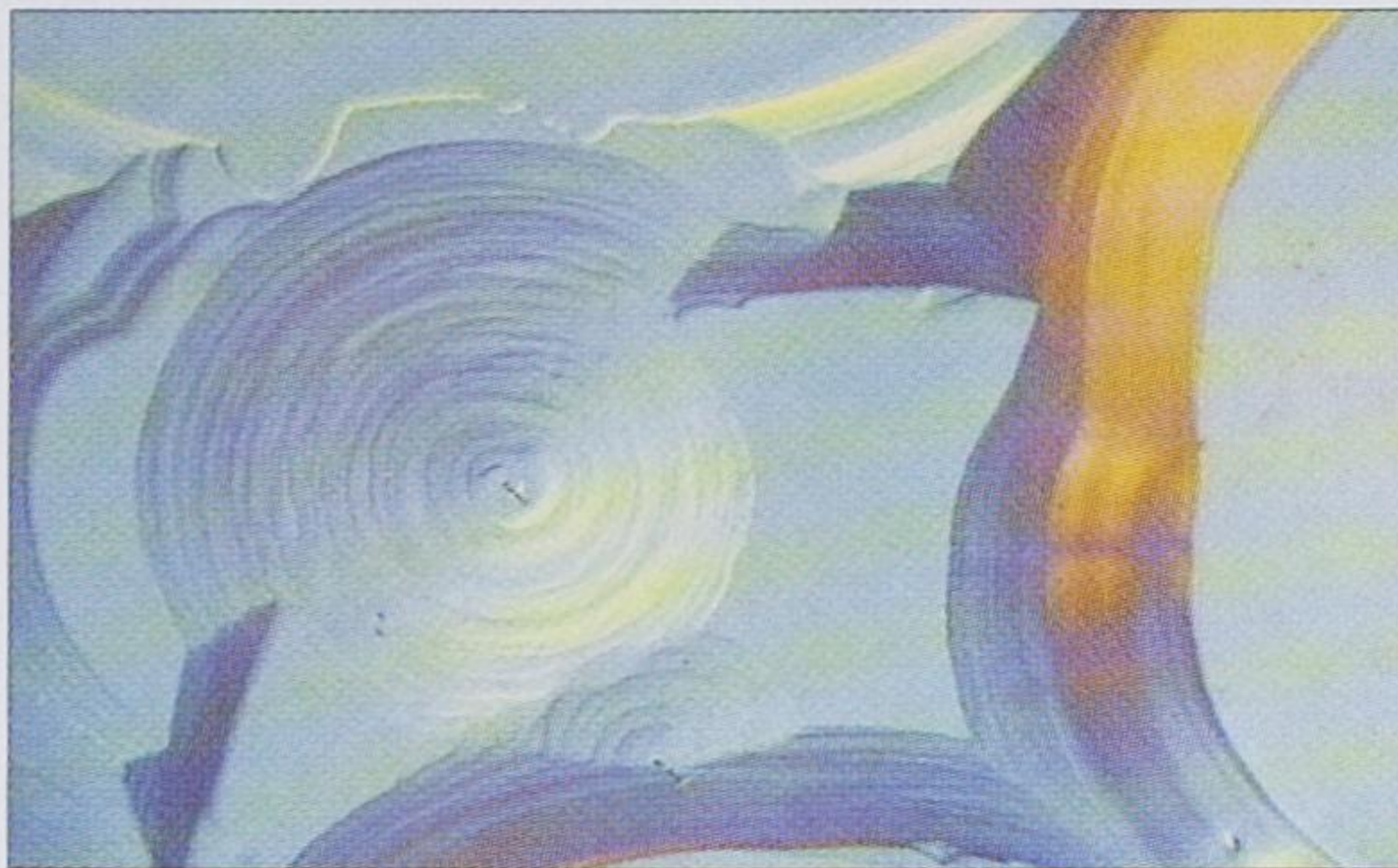
Caracal's prize-winning on-axis epitaxial 4H-SiC. The lines demarcate coalescing SiC islands.
