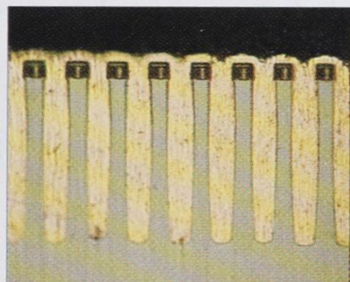
Copper-filled through-silicon vias , seen here, is a growing application area.
