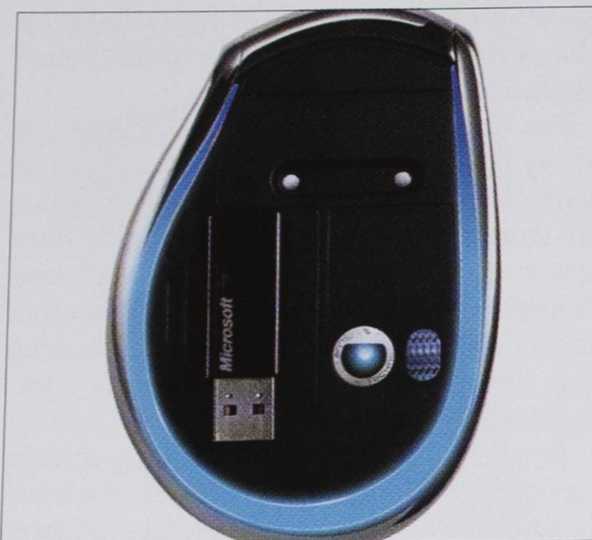
Microsoft's Blue Track mouse uses blue LED light, which is disrupted less easily than coherent red lasers on its way back to the mouse's photosensor.
