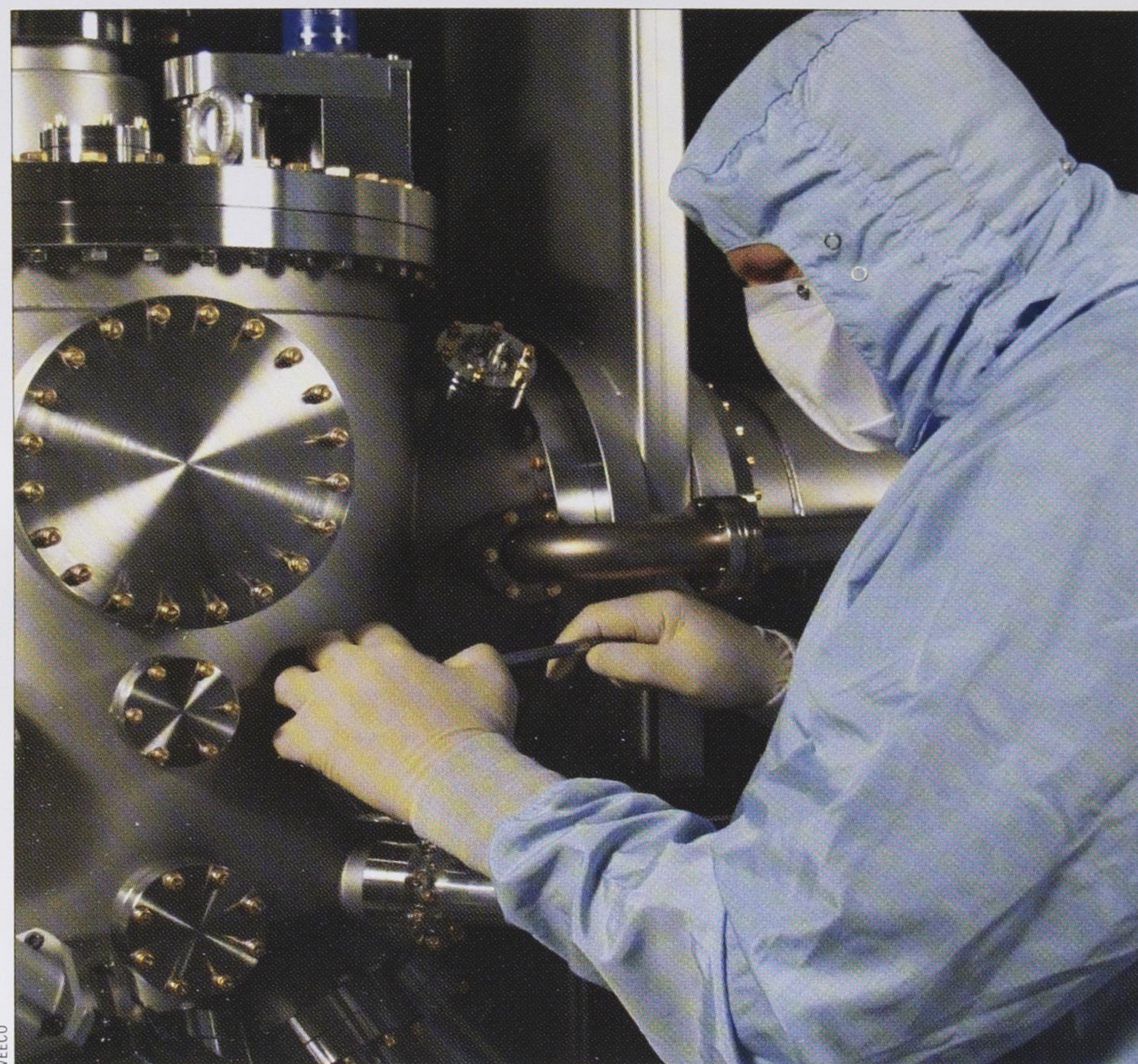
The Veeco GEN10 is a flexible system that can feature up to three separate growth modules. This enables simultaneous MBE development by researchers working on different materials.
