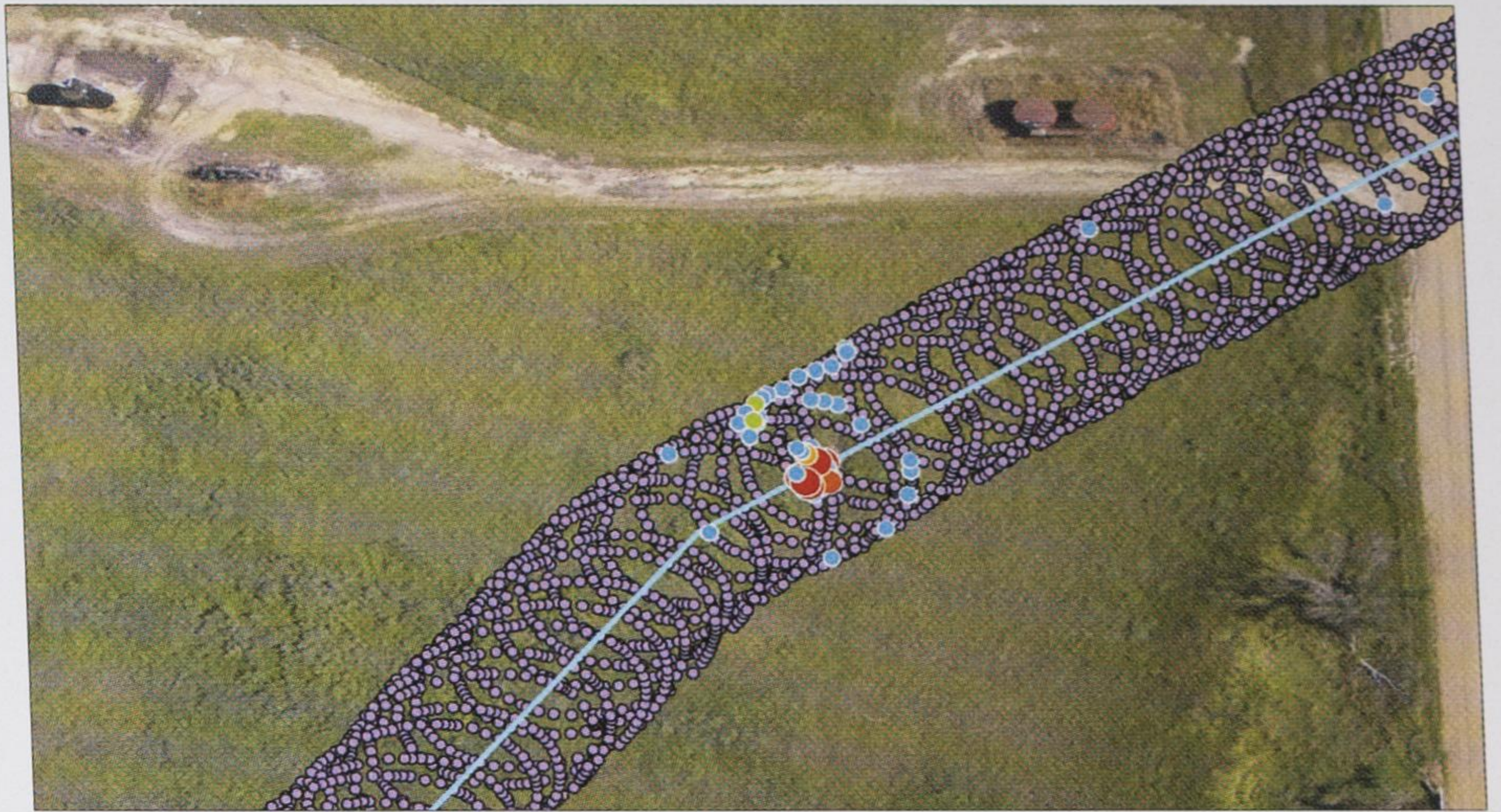
Gas leaks from an underground pipe have been detected by differential absorption, using an instrument mounted in the low-flying aircraft ITT Angel Service. This approach is far quicker than the traditional methods involving hand-held instruments and it can cover 1000 miles per day.
