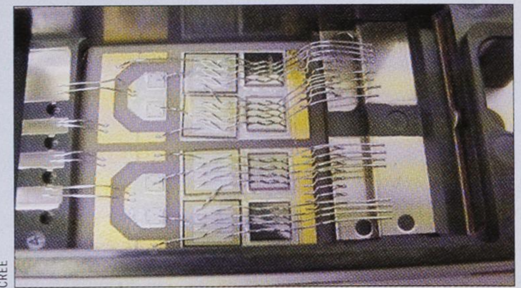
Power modules feature several semiconductor die that are housed in an encapsulated package (top left). Cree's dual power module for the Air Force Research Lab (bottom left) can either employ five 20 A MOSFET die per switch (top right) or two 50 A MOSFET die per switch (bottom right) to deliver 100 A.
