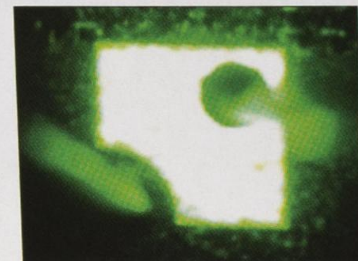
MOCVD growth on 6 inch silicon-on-insulator substrates produces thick crack-free GaN films that are processed into green and deep-green LEDs. Surface texturing has improved light output.
