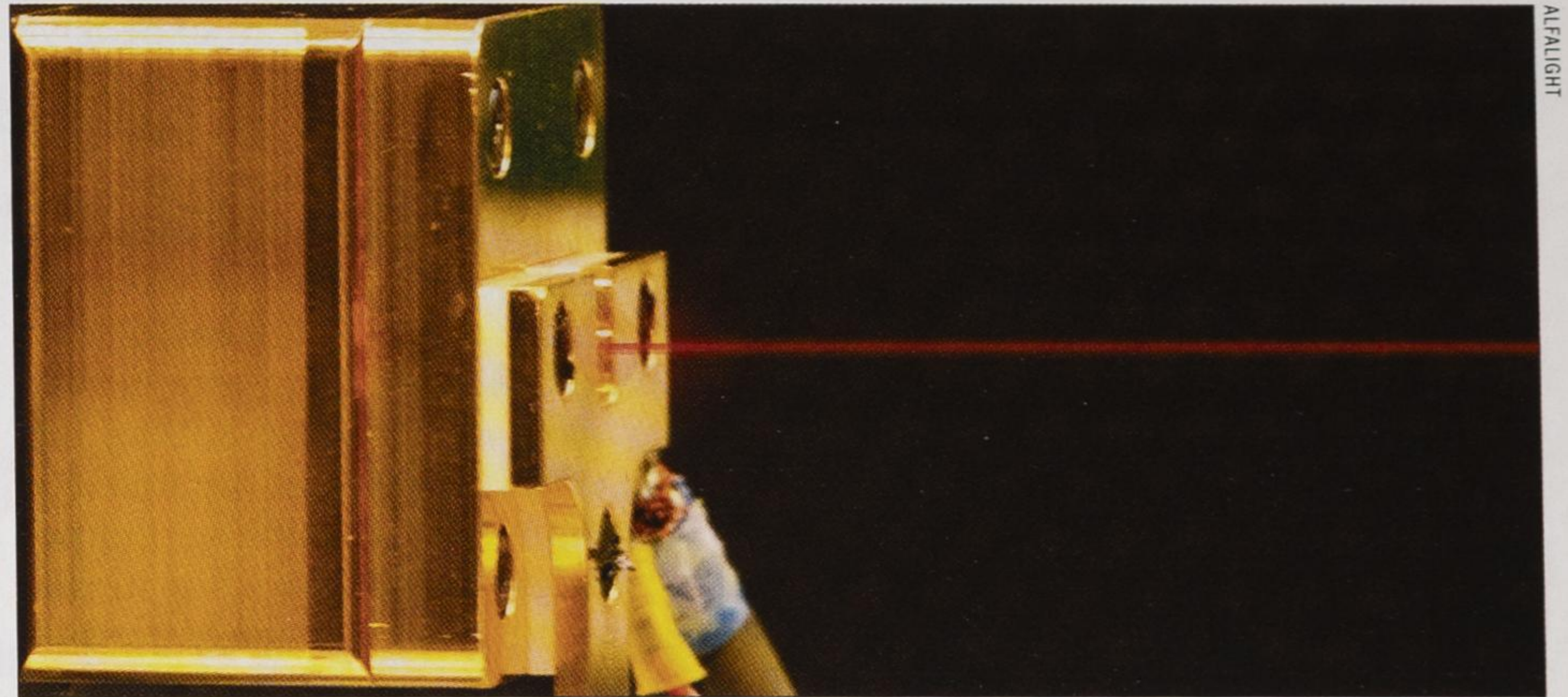
Alfalight's surface-emitting distributed feedback laser produces a collimated longitudinal beam that can be used for cutting, welding and the pumping of fiber and solid-state lasers.
