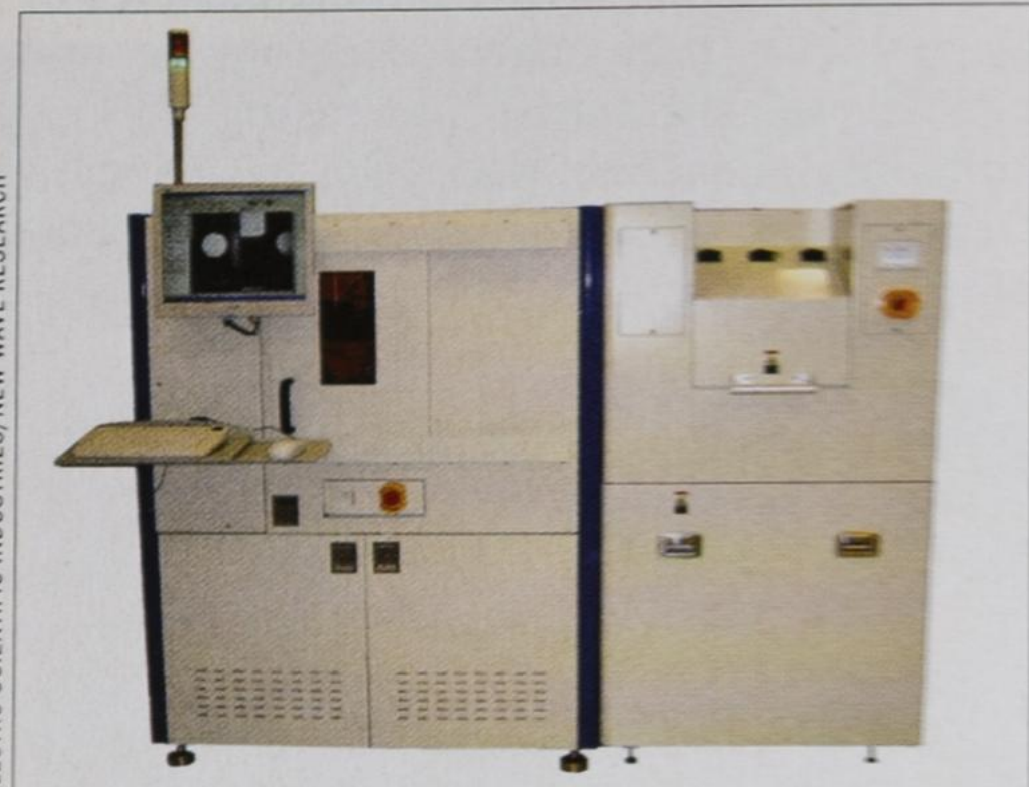
The AccuScribe 2155 laser scribe from Electro Scientific Industries features automated loading and unloading of wafers from and to cassettes.
