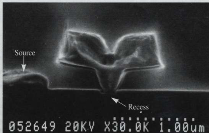
Figure 1. Cross-Sectional SEM of a wide head T-gate MESFET fabricated by split E-Beam lithography. The footprint and top width of the T-gate are 0.13 \mu\text{m} and 1.35 \mu\text{m} , respectively. SEM courtesy of Jin Hee Lee, ETRI (Taejeon, Korea)
