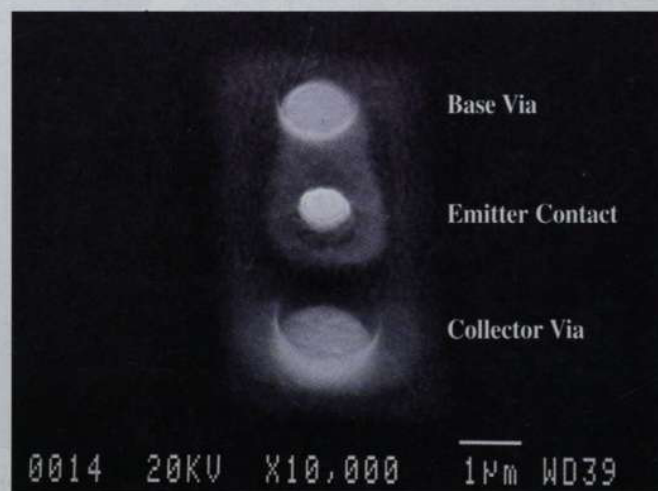
Figure 3. SEM of a fully self aligned AllnAs/GaInAs, InP-based HBT with 0.3 \mu\text{m}^2 emitter. SEM courtesy of Madjid Hafizi, Hughes Research Laboratories (Malibu, CA).
