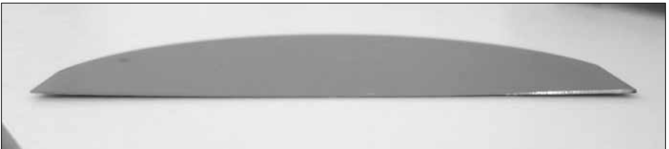
Figure 2. A typical cross-section of a 100 mm diameter high-temperature grown 3C-SiC epi-layer grown using a traditional high-temperature process. The thermal stresses cause bowing of the wafer.
