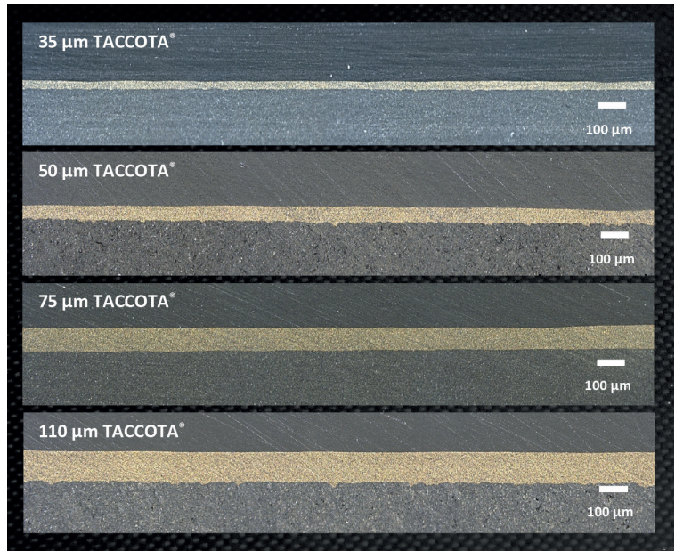
➤ Figure 1. The TaC process technology developed at Fraunhofer IISB allows adjustment of desired coating properties, such as thickness, shown here in the range 35 µm to 110 µm.
