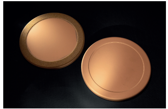
➤ Figure 3. SiC wafer carrier before (right) and after (left) several standard SiC epilayer processing runs.
