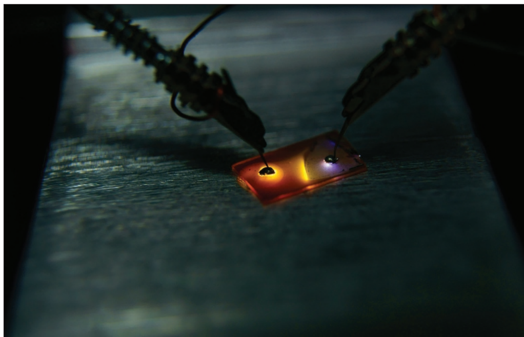
Yellow-orange InGaN test device. The probe to the left is on a high indium content n -type InGaN layer. The probe to the right is on the underlying p -type GaN template. The blue purple emission from the p -GaN probe is because of the slightly n -type surface oxide, one of several possible sources of n -type minority carriers.
