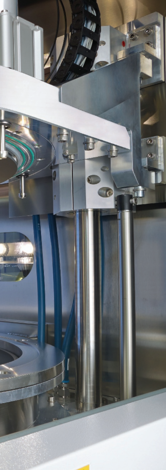
LEFT: The reactor chamber of Aixtron's Planetary system AIX G5+ that can be used for the growth of GaN on 200 mm silicon substrates.
