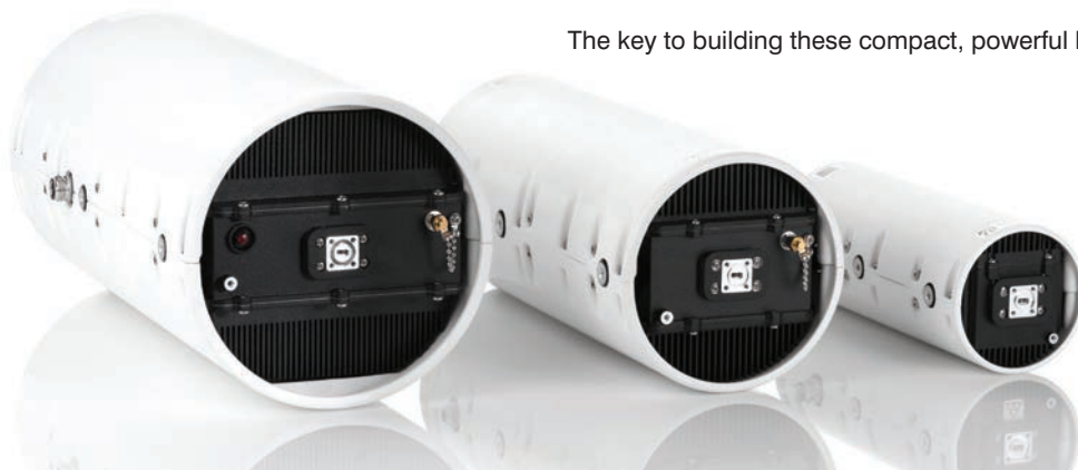
Figure 4. Mission Microwave's satellite communication block upconverter portfolio. From left to right, 200 W, 100 W, and 25 W K_a -band block upconverters that can efficiently provide linear output powers in industry-leading compact packages. At K_u -band, similarly-sized upconverters can provide 200 W, 100 W, and 55 W of output power.
