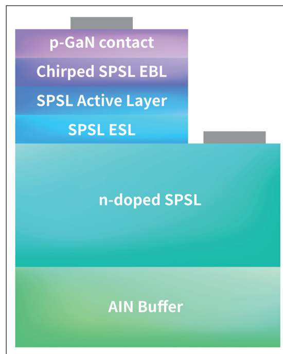
➤ Figure 5. Heterostructure for Silanna LEDs, utilising the short-period superlattice through almost the entirety of the device stack.
