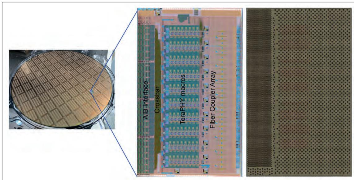
This enables fine-pitch 2.5D-type packaging without having to use a silicon interposer. Instead of that we can use an organic substrate, which provides greater flexibility in terms of area and yield.
