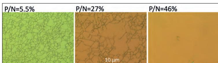
Cranking up the flow of tertiary-butylphosphine increases the ratio of phosphor-to-nitrogen and reduces the density of cracks in the AIPN layer.
