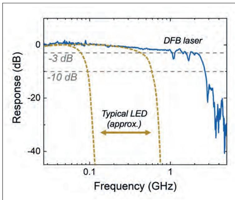
Figure 7. High-speed modulation bandwidth of the sky-blue DFB laser compared with the approximate bandwidth of typical LEDs (ranging from high-power LEDs to faster microLEDs).
