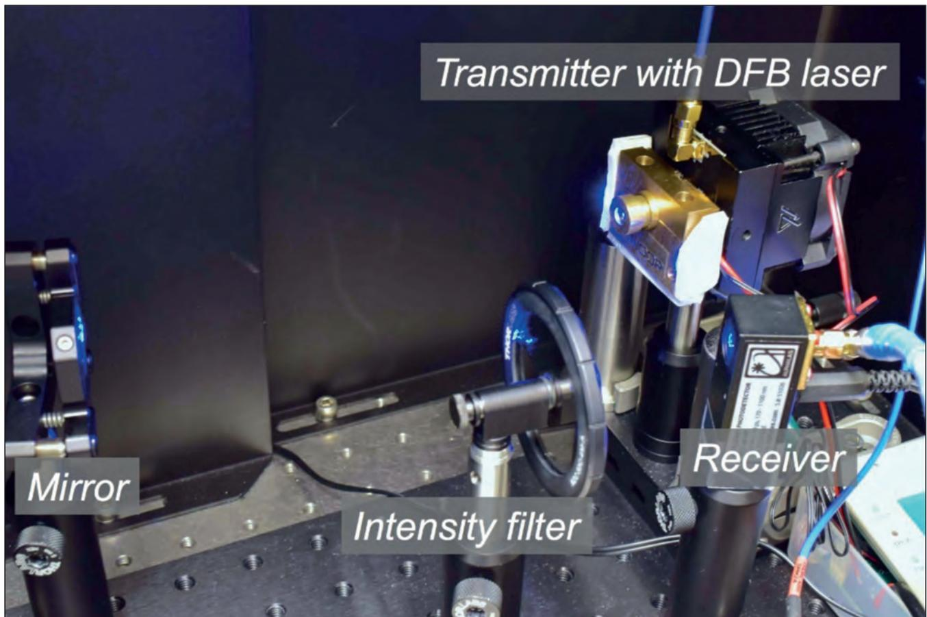
Figure 6. KAUST's testbed for proof of concept. The goal is beyond 10 Gbit/s using a GaN DFB laser.
