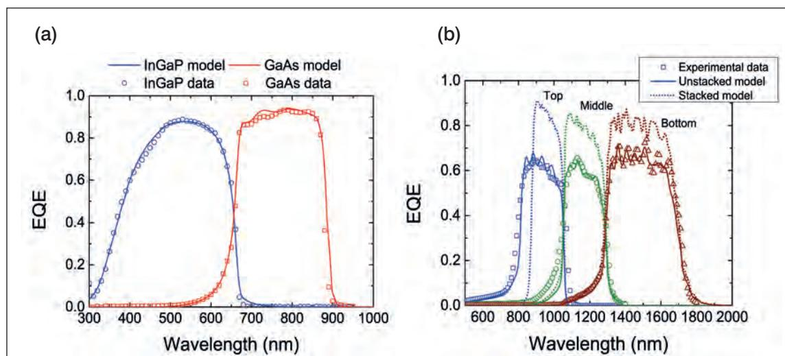
Figure 4. (a) Measured and simulated external quantum efficiency (EQE) for the GaAs double-junction cell. (b) Measured and simulated EQE spectra for the InP triple-junction cell. The implied EQE after stacking is shown by the dotted lines.
