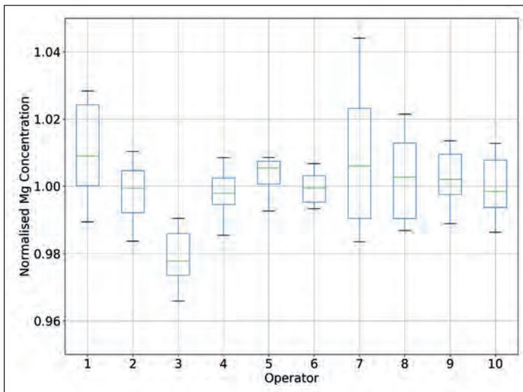
Figure 5. Representative results of a nested Gage reproducibility and reliability study on the determination of the magnesium concentration in the *p*-type GaN layer of a full normally-off GaN HEMT structure.
