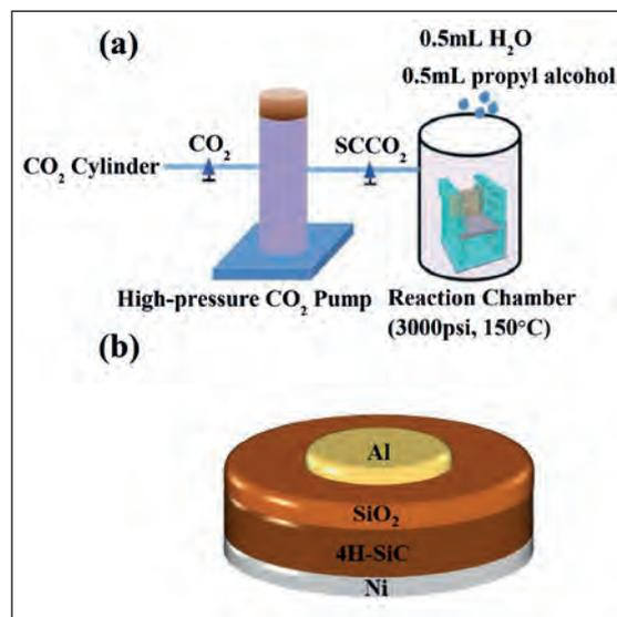
Treatment with supercritical CO<sub>2</sub> (a) is applied to MOS structures (b).
