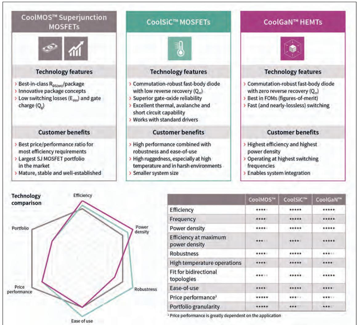
conducting, which dissipates the energy build-up that limits the switching frequency of silicon devices. It is the switching characteristics of SiC that are behind its capability to deliver higher efficiency.
