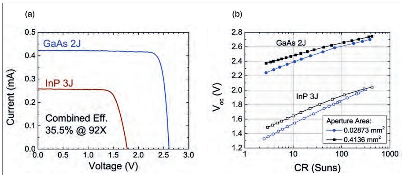
Figure 5. (a) Light current-voltage (I-V) curves for the stacked GaAs- and InP-based multi-junctions, which give a combined efficiency of 35.5 percent under simulated AM0 illumination. (b) Measured open-circuit voltage ( $V_{oc}$ ) for microcells with different perimeter-to-area ratios, highlighting the losses at low concentration due to perimeter recombination.
