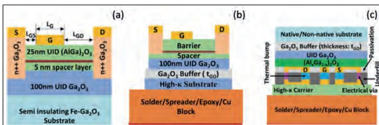
The thermal management of a Ga<sub>2</sub>O<sub>3</sub> MODFET (a) can improve by inserting a high thermal conductivity substrate (b). Even better results are possible with a double-sided cooling design (c).
