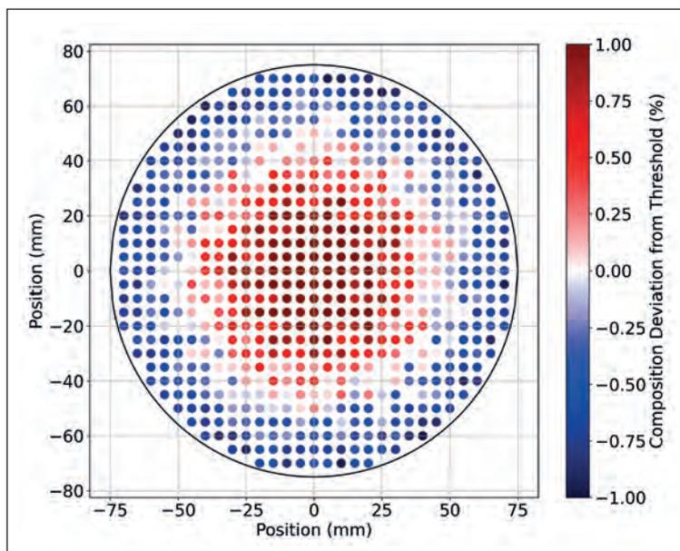
Figure 3. The Sântis 300 platform is capable of producing a wafer map of the aluminium composition of a buried AlGaIn layer in a GaN HEMT structure (simulated data).
