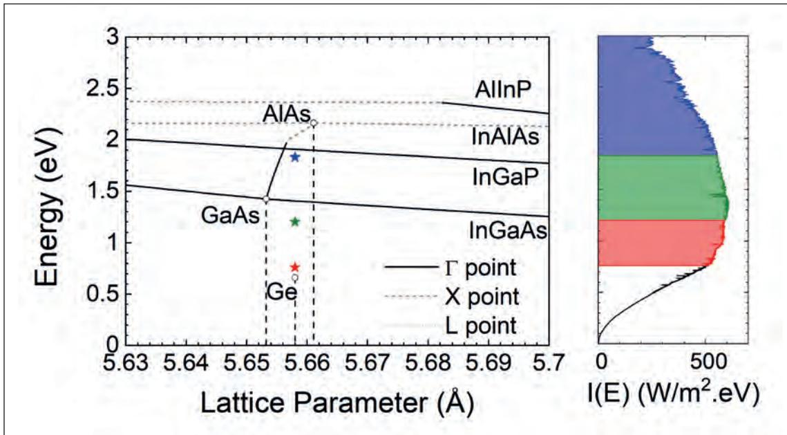
Figure 1. The ideal bandgaps for conversion of AMO illumination from the detailed balance limit in a triple-junction solar cell, compared with available bandgaps of III-As and III-P alloys on germanium.
