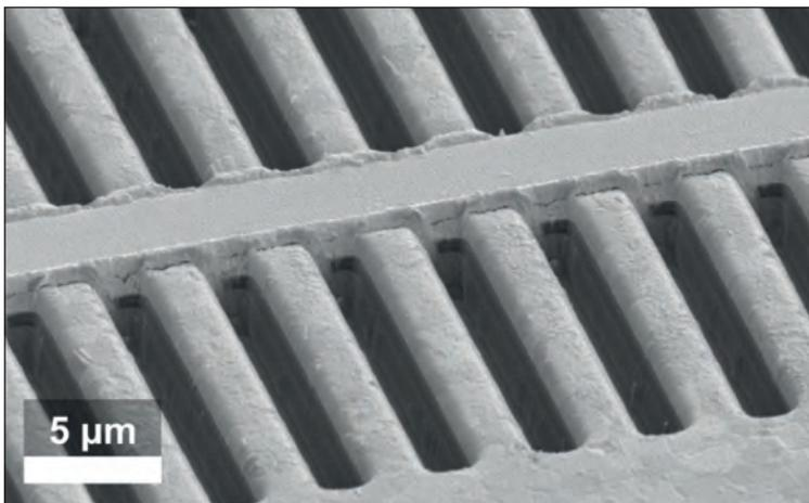
Figure 2. A DFB grating fabricated on the surface of a laser diode from KAUST. Using a surface grating allows a single-mode output without the need for the difficult overgrowth process in GaN lasers.
