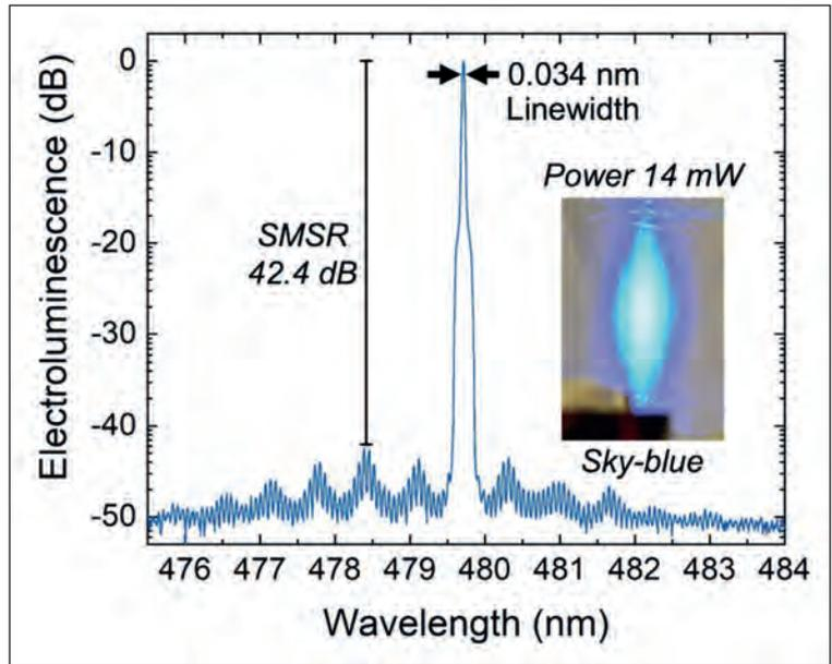
Figure 5. Sky-blue DFB laser emission shows a resolution-limited single-mode at around 480 nm. The inset shows a real-colour image of the laser far-field pattern. The side-mode suppression ratio (SMSR), linewidth, and optical power help to assess the quality of the DFB laser.
