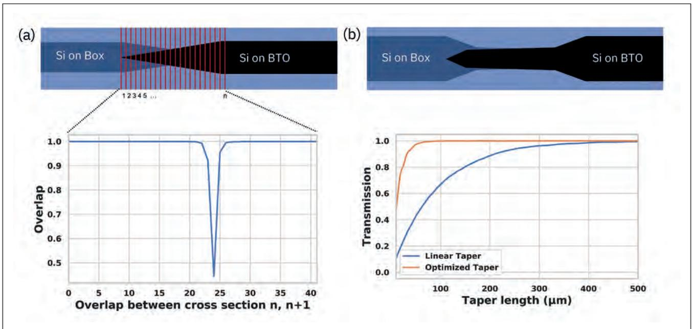
Figure 9.(a) Simulations of optical modes in 42 cross sections (red lines) along the taper. Mode overlap between consecutive sections were computed. (b) Simulated transmission for light coupling from silicon to a BTO/silicon layer as a function of taper length. A transmission value of 1 means that the mode is transferred without any loss. Using the optimised taper shape, a transmission exceeding 99.5 percent is realized for 90 μm-long tapers.
