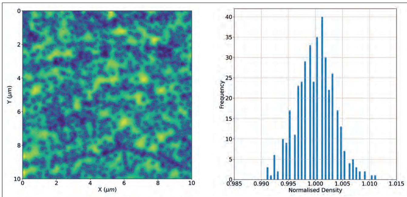
Figure 1. (a). A cathodoluminescence image with threading dislocations identified by the highlighted Attolight image reconstruction solution. (b) Histogram of normalised threading dislocation densities, recorded over several hundred iterations of the image reconstruction algorithm.
