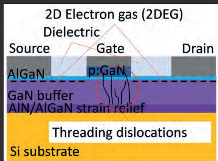
This is the general design of the junction-gated, normally-off HEMT, typically used for power-conversion applications. Threading dislocations are present in the entire sample. This sketch just indicates their presence and direction, especially under the gate, where they have potentially the largest impact.
