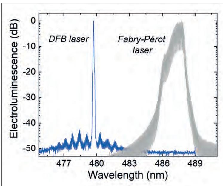
Figure 1. The multiple cavity modes of a Fabry-Pérot laser can be reduced to a single mode by adding a DFB grating. The figure shows a GaN-based sky-blue colour laser.
