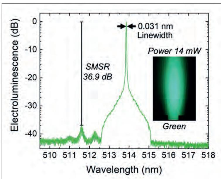
Figure 4. Green DFB laser emission shows a resolution-limited single-mode at around 514 nm. The inset reveals a real-colour image of the laser far-field pattern. The side-mode suppression ratio (SMSR), linewidth, and optical power help to evaluate the quality of the DFB laser.
