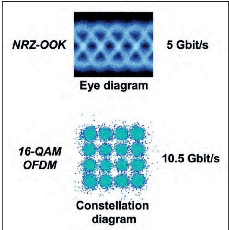
Figure 8. Digital communications can be represented visually depending on their modulation format. The figure shows the eye and constellation diagrams produced by the DFB laser.
