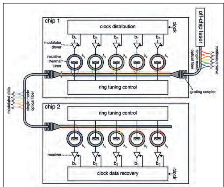
Figure 6. A complete WDM link system that integrates electronics with photonics components (Source: Ayar Labs).
