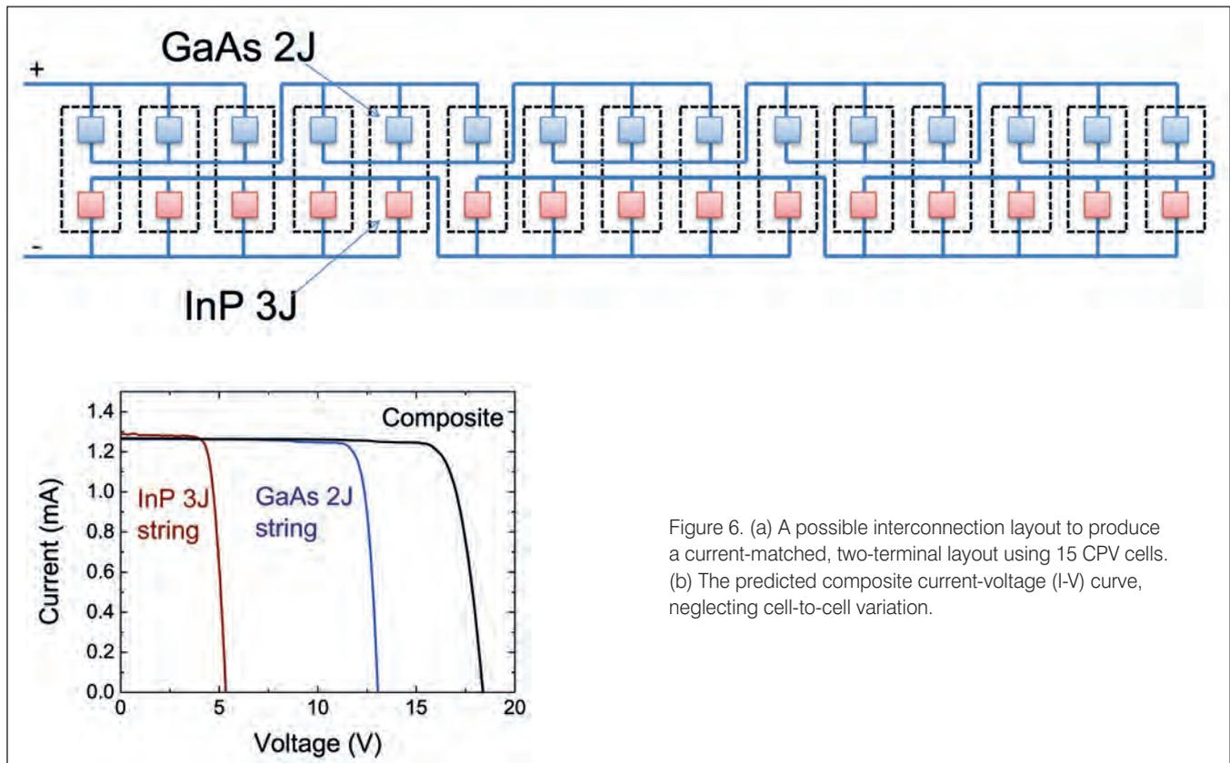
Figure 6. (a) A possible interconnection layout to produce a current-matched, two-terminal layout using 15 CPV cells. (b) The predicted composite current-voltage (I-V) curve, neglecting cell-to-cell variation.
