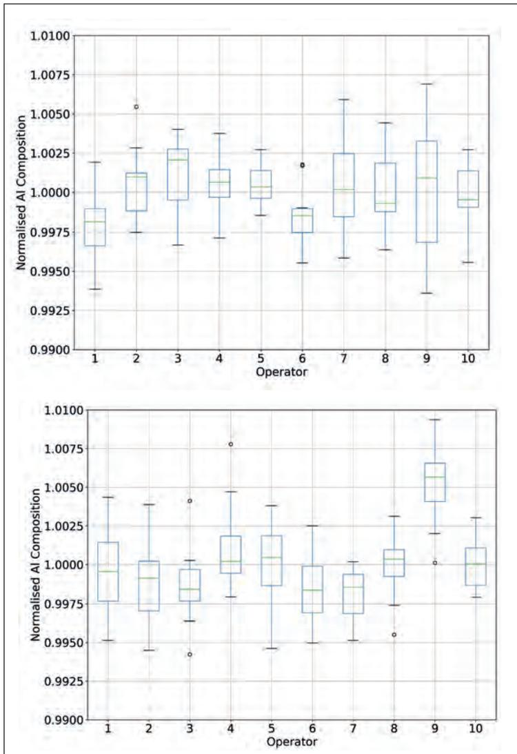
Figure 4. Representative results of a nested Gage reproducibility and reliability study on the determination of aluminium composition in the AlGaIn layer of: (a) a full normally-off GaN HEMT structure (buried layer); and (b), the equivalent HEMT structure with the  $p$ -type GaN cap removed (surface layer).
