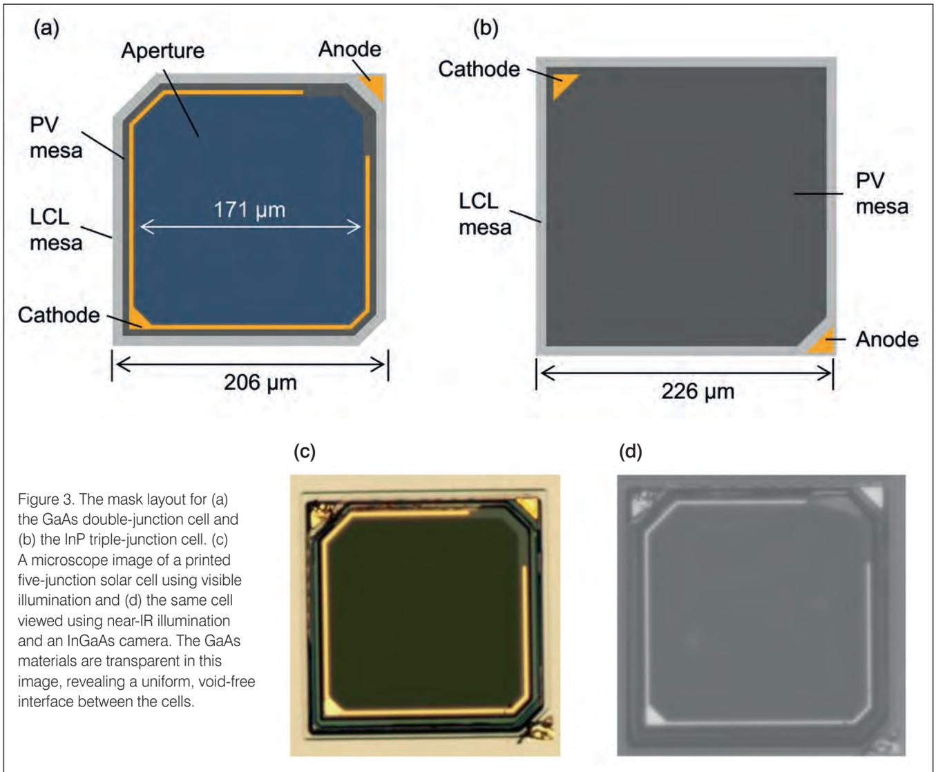
Figure 3. The mask layout for (a) the GaAs double-junction cell and (b) the InP triple-junction cell. (c) A microscope image of a printed five-junction solar cell using visible illumination and (d) the same cell viewed using near-IR illumination and an InGaAs camera. The GaAs materials are transparent in this image, revealing a uniform, void-free interface between the cells.
