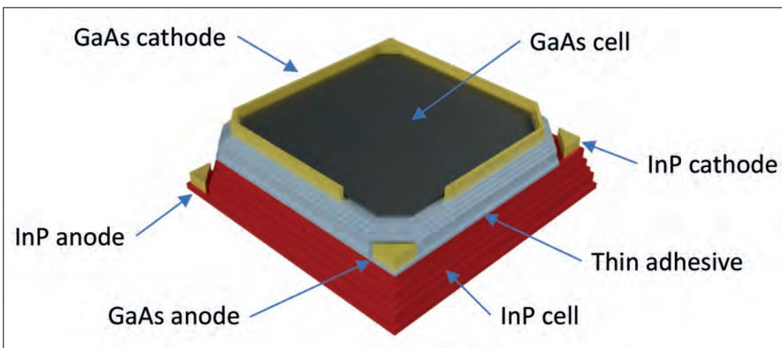
Figure 2. A stacked micro-CPV cell, formed from separate GaAs and InP-based multi-junction solar cells, can form a four-terminal device.
