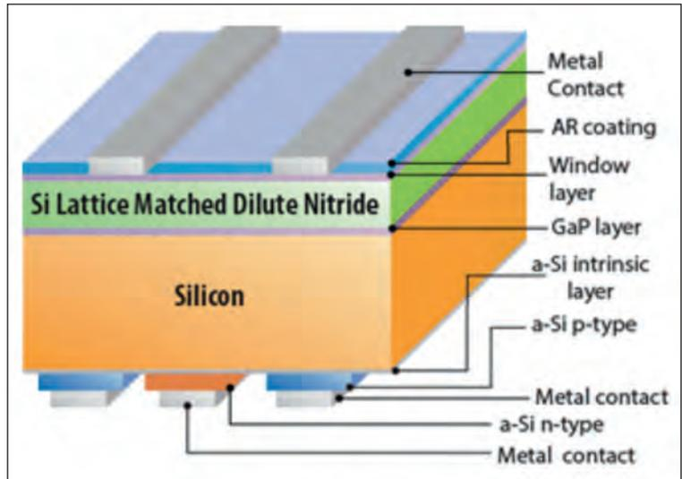
energy from the silicon cell. She also pointed out that to get the best output from the tandem, the bandgap of the top cell needs to be higher when working with imperfect material.
