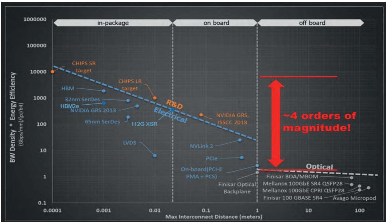
range electrical connections – they are incapable of spanning the signalling lengths required for off-board, rack-scale communication.
