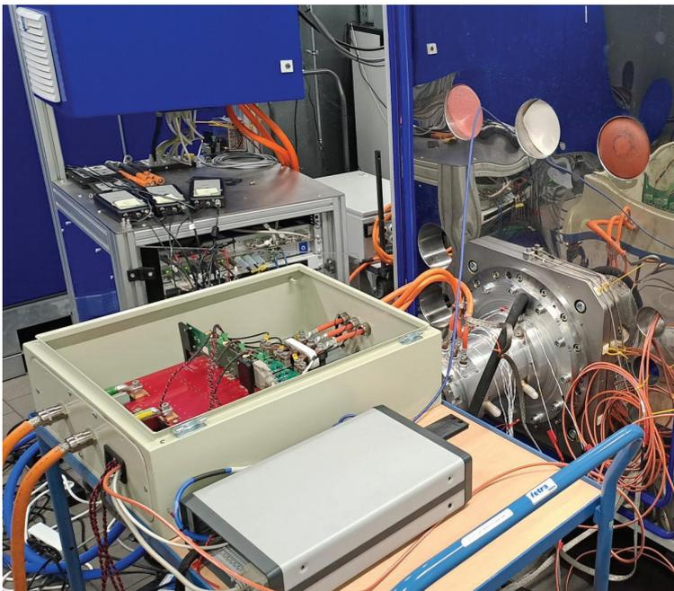
➤ AVL Dyno test setup with a VisIC D3GAN power inverter.
