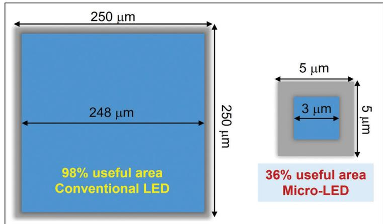
➤ Figure 1. Illustration (not to scale) of the effect of sidewall damage (assuming 1  $\mu\text{m}$  depth) with microLED device size scaling – the damage does not scale and hence the percentage of luminous area reduces significantly with size.
