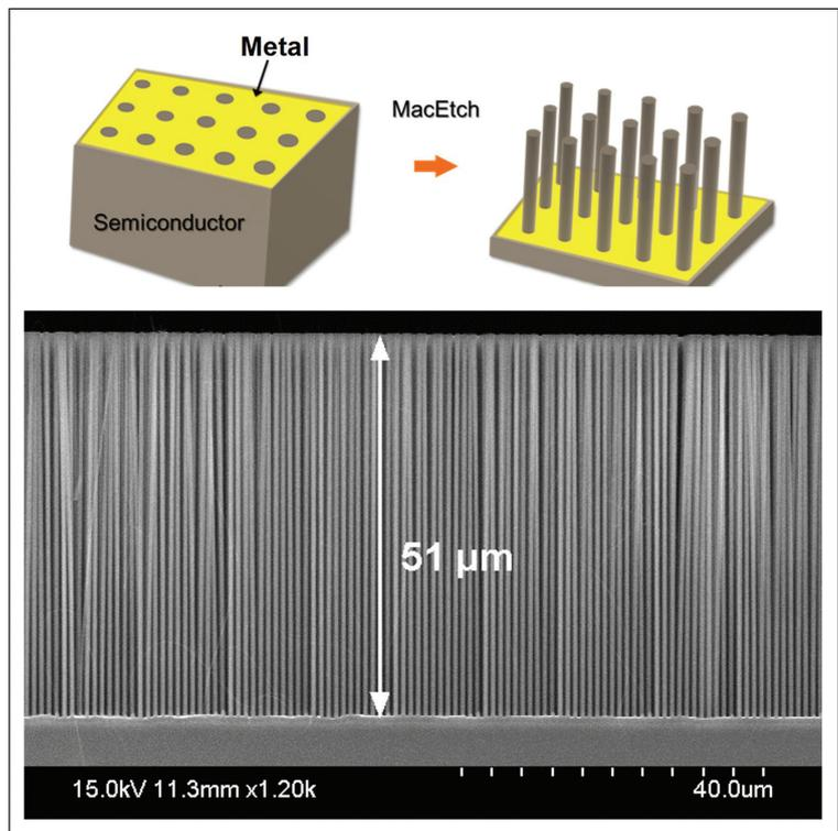
➤ Figure 2. MacEtch process illustration and a scanning electron microscopy image of an array of silicon nanowires (diameter = 550 nm, depth = 51  $\mu\text{m}$ ) produced by gold-MacEtch. For more details, see X. Li., *Curr. Opin. Solid State Mater. Sci.* **16** 71 (2012) and K. Balasundaram *et al.* *Nanotech.* **23** 305304 (2012).
