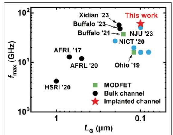
➤ Figure 7.  $\beta$ -Ga<sub>2</sub>O<sub>3</sub> MOSFETs that feature a diamond foundation and are produced using transfer printing are setting new benchmarks for  $f_T$  and  $f_{MAX}$  for MOSFETs made with this ultra-wide bandgap oxide.
