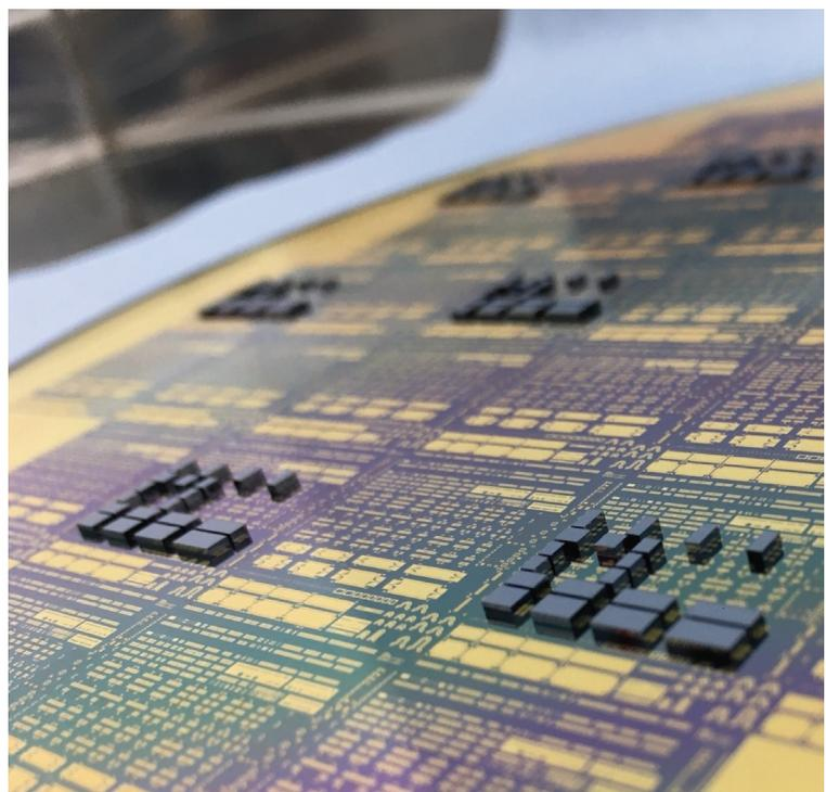
► Figure 3. (left) Transistor ready for pick and place assembly (right). Future package heatsink emulation using a copper finger, allowing higher electrical performance.
