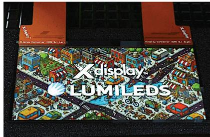
The new microLED display has an architecture based on a cluster drive system combined with microLEDs that measure  $13 \times 20 \mu\text{m}^2$ . The result is a peak brightness of  $2360 \text{ cd m}^{-2}$ . Notably, the mass transfer process employed in the development of these prototypes achieves 99.9998 percent microLED sub-pixel yield and a 99.992 percent microIC transfer yield, according to the partners. The processes used to manufacture the prototype are mass-production ready.
