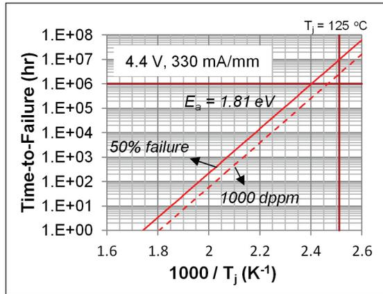
➤ Figure 7. Reliability test result of 70 nm pHEMT.
