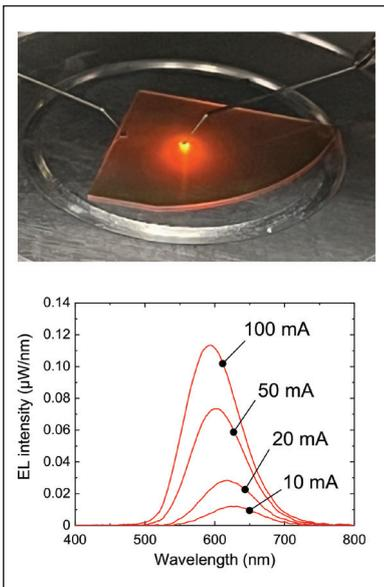
➤ Significant indium compositional fluctuations in the quantum well account for broad electroluminescence.
