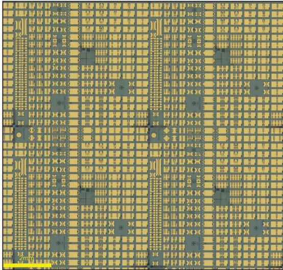
enables a true 'mix-and-match' of different devices, such as InP and GaN, in a single PLIC. This enables optimal architectures that are free from multi-chip modules. Finally, as the interposer is built on wafers with a diameter of at least 8 inches, they have at least four times the area of the 4-inch wafers used in typical III-V processes, leading to significant fab throughput and cost advantages.
