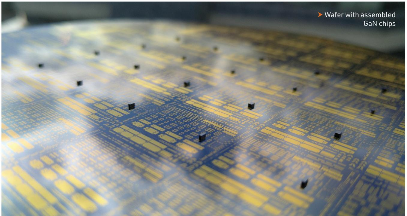
► Wafer with assembled GaN chips
