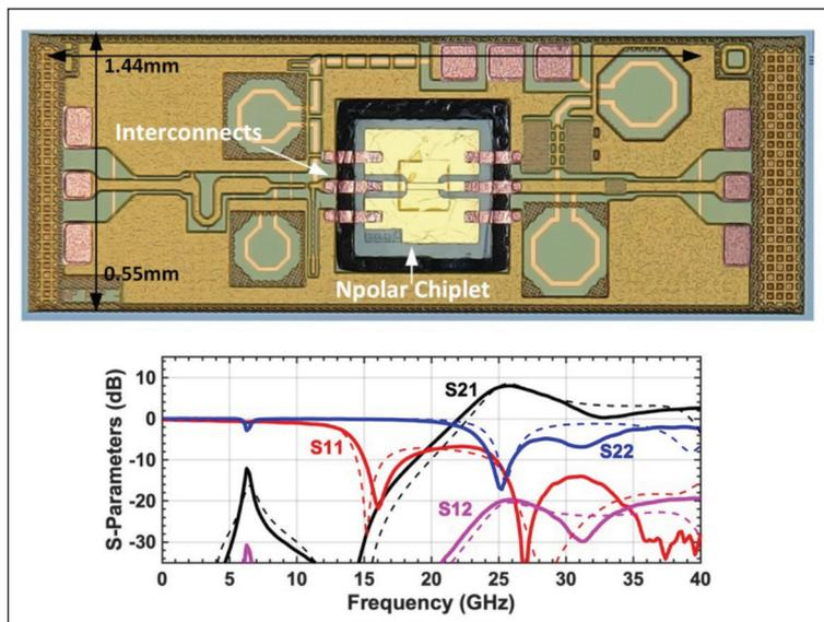
► Figure 6. (top) Chip microphotograph of the 26 GHz heterogeneously integrated amplifier illustrating the compact implementation of the input and output matching networks. For clarity, the HEMT chiplet and interconnect are highlighted. (bottom) Simulated (dashed) and measured (solid) S-parameters of the heterogeneously integrated amplifier. A peak gain of 8.0 dB occurs at 26 GHz.
