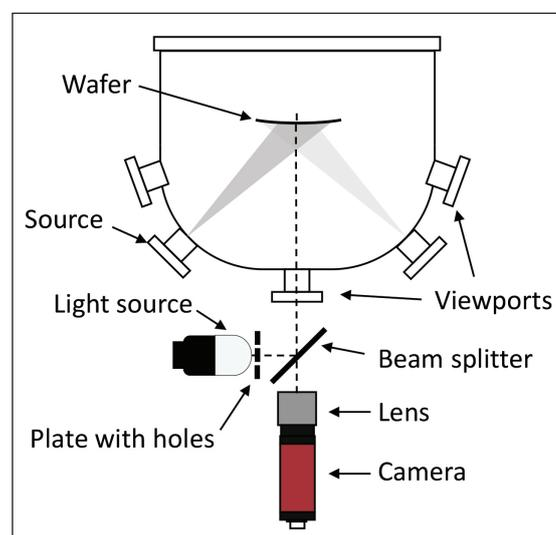
➤ Figure 1. The magnification inferred curvature principle.
