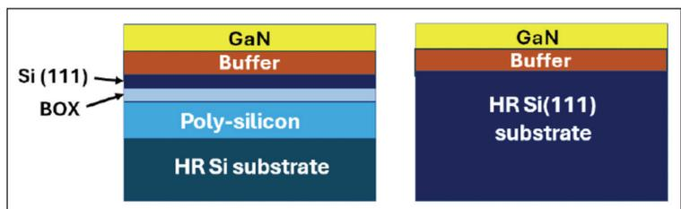
➤ Figure 2. (a) Intel has used 300 mm trap-rich SOI as a foundation for producing GaN MOSHEMTs on 300 mm silicon wafers. The thin silicon (111) layer serves as a crystalline template for GaN epigrowth. Beneath this is an underlying insulating buried oxide (BOX), and below that a trap-rich polysilicon layer that eliminates stray charges at the interface to the BOX, as well as a high-resistivity silicon substrate.
