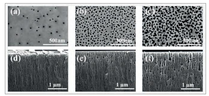
Figure 2. (a-c) Top-view and (d-f) cross-sectional scanning-electron microscopy images of nano-porous GaN with different porosity etched at different bias voltages. Reprinted with the permission of the American Society Chemistry.
