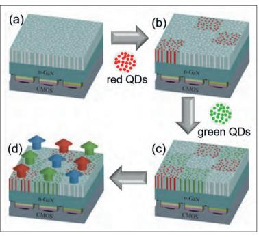
Figure 5. Saphlux's approach to making monolithic RGB microLEDs. (a) A vertical blue LED with exposed nano-porous GaN is bonded to a current-driver panel. (b) Red quantum dots are selectively loaded into red zones. (c) Green quantum dots are selectively loaded into green zones. (d) Red, green and blue light emitted from red quantum dot zones, green quantum dots zones, and zones without any quantum dots, respectively.
