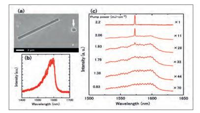
Figure 5. (a) Scanning electron microscopy image of a nanowire mechanically dispersed onto a gold-film-covered SiO<sub>2</sub>-on-silicon substrate. The white arrow indicates a removed indium particle. (b) Photoluminescence spectrum of a single nanowire under a pump laser power of 0.83 mJ cm<sup>-2</sup>. (c) Photoluminescence spectra of the nanowire with increasing pump power, revealing spectral narrowing.
