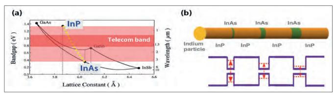
Figure 1. (a) Bandgap and lattice constant of III-V compound semiconductors. InP/InAs can cover a wide spectral range, including the telecom band. (b) Lattice-matching constraints are far less severe in InP/InAs heterostructure nanowires connected by a single indium particle, than in conventional heterostructures. In these nanowires, the quantum confinement effect along the axial direction allows the real bandgap of the InAs layer to be modulated by the thickness.
