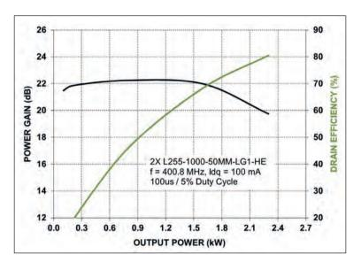
Figure 1. Measured RF power gain and drain efficiency versus output power at 145 V bias and 400.8 MHz. Quiescent current is 100 mA. 6  $\Omega$  series gate resistors help to stabilise the transistor with 20 dB gain at 2 dB compression and 2.3 kW saturated power. Drain efficiency peaks at 80 percent. In CW operation at 100 V bias, saturated power is 1.2 kW with the same 80 percent peak drain efficiency.
