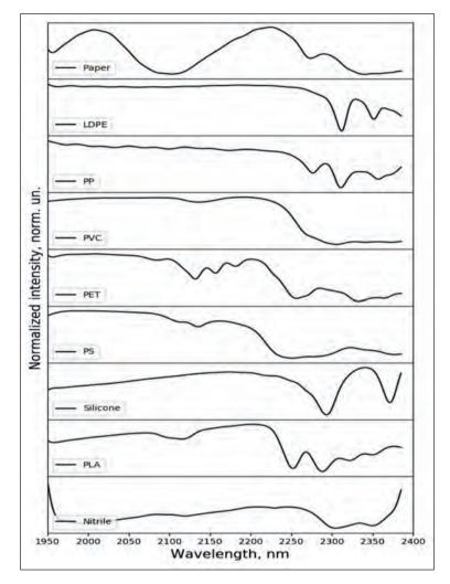
Figure 7. Sorting different types of plastic can draw on the transmission spectra of different materials.
