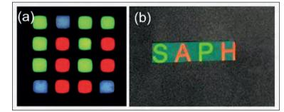
Figure 6. (a) Saphlux RGB monolithic microLEDs excited by a blue LED source from the backside. (b) A picture of the company logo "SAPHLUX" fabricated by red and green nano-porous quantum-dot microLEDs.
