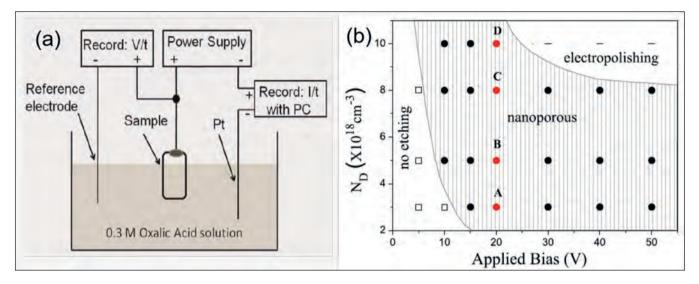
Figure 1. (a) An electrochemical etching process produces nano-porous GaN. (b) A phase diagram of the GaN electrochemical etching process shows how the etching characteristics are related to silicon doping in GaN and the applied bias.
