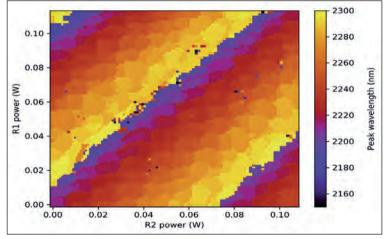
Figure 4. The peak wavelength of Brolis' single widely-swept laser, when both micro-rings are electrothermally tuned in a specific manner. Continuous spectral coverage is clearly visible.
