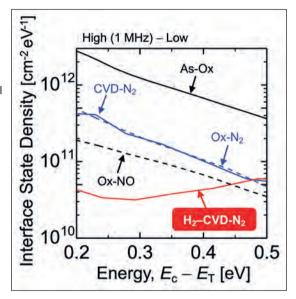
on *n*-type 4H-SiC (0001) epilayers. As part of this study, they investigated whether the benefits of the nitridation process were simply due to the high temperature employed – it takes place at 1400 °C – or resulted from the use of  $N_2$  gas. To test the latter, the team compared results with those associated with a similar process involving argon. The engineers also fabricated MOS capacitors by dry oxidation to aid comparison.
