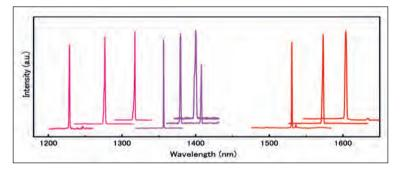
Figure 6. Nanowires allow a tuning of the laser wavelength range in the telecom band. Spectra are offset for clarity. The laser wavelength is modulated by the growth parameters, such as flow rates of the metal-organic sources. Thus a broad wavelength range is covered in the whole telecom band, including the two technologically important telecom-band windows centred around 1.3  $\mu$ m and 1.55  $\mu$ m.
