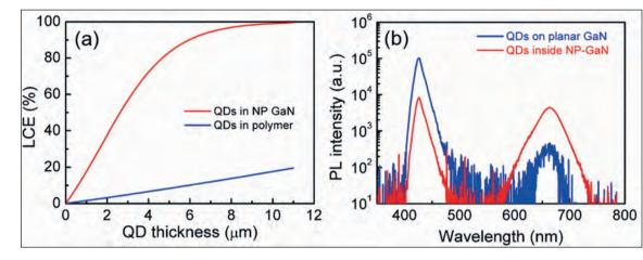
increase in device efficiency. For planar quantum dots in a polymer film, light-conversion efficiency increases linearly with increases in the thickness of the quantum dot layer to a maximum of only 20 percent – that's for a 10  $\mu$ m-thick quantum-dot layer (see Figure 3(a)). In stark contrast, when dots fill the nanopores, light-conversion efficiency exceeds 80 percent, for a film thickness of just 5  $\mu$ m.
