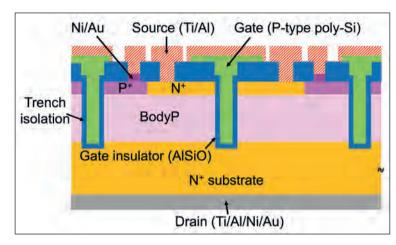
Engineers at Nagoya University, Japan, have increased the mobility of the channel in vertical GaN **MOSFETs** by turning to an in-situ nitrogen plasma treatment in an atomic layer deposition chamber.
