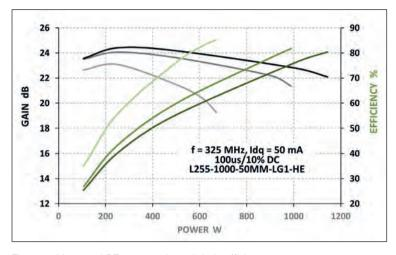
Figure 2. Measured RF power gain and drain efficiency versus output power for a 50 mm die with a signal of 100  $\mu s$  pulse width and 10 percent duty cycle at 325 MHz. The device is characterized at 100 V, 125 V and 145 V DC bias demonstrating a 3 dB power dynamic range. By reducing operating bias to 50 V a 6 dB dynamic range is achieved.
