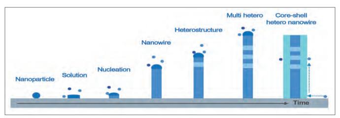
Figure 3. Schematic diagram of the vapour-liquid-solid growth mode. InAs and InP nanowires can be grown by the self-catalysed vapour-liquidsolid mode using indium particles.
