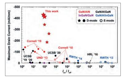
Figure 5. A partnership between engineers at Cornell and Intel has propelled the drain current for *p*-channel HEMTs to a new high. Success results from scaling device dimensions and trimming the contact resistance.
