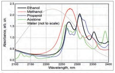
Figure 1. Infrared spectroscopy can identify ethanol, methanol, propanol and acetone by their unique absorbance spectra. The light grey line shows superimposed water transmission spectra.
