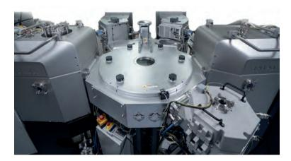
mainstream MOSFET's and IGBT benefit from the above merits enabled by advanced integrated ALD technology. Thanks to rapid advances in ALD equipment technology, throughput can now be scaled by using batch process i.e. 25 wafer batch as much as needed. Thermal batch ALD enables production-worthy throughputs (double digit) for thickness in the range of 10 to 100 nm. Beneq Transform<sup>™</sup> © All rights reserved.
