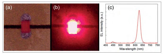
Figure 7. Photos of  $100 \times 150 \,\mu$ m<sup>2</sup> red nano-porous quantum dot miniLED mounted on a PCB board (a) and lit-up at an injection current of 1 mA (b). (c) Spectrum of a red nano-porous quantum dot LED shown in (b). Testing the reliability of the red nano-porous quantum-dot miniLED revealed acceptable results at 30 W cm<sup>2</sup>. This power density is more than sufficient for most microLED applications.
