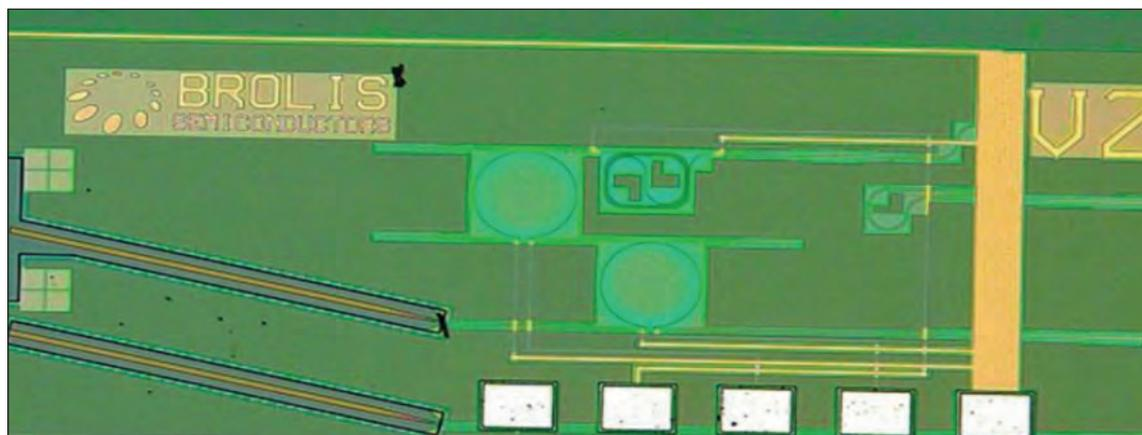
Figure 2. The SOI part of Brolis' widely-swept GaSb/SOI hybrid laser. Two coupled micro-rings are clearly visible.
