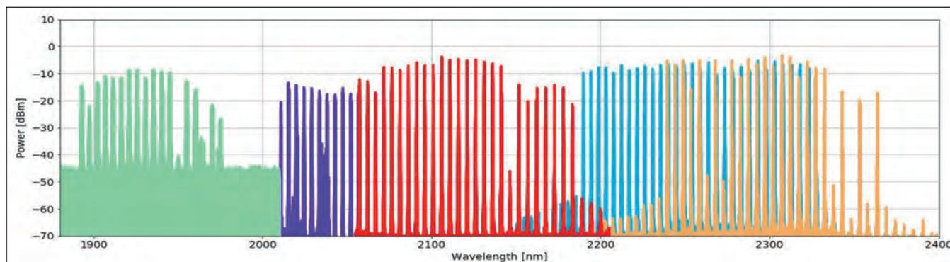
Figure 3. Superimposed spectra show that four widely-swept GaSb/SOI lasers can cover the spectral range from 1900 nm to 2400 nm. Devices exhibit continuous-wave lasing with output powers of around 1 mW. As tuning involved only tuning a single micro-ring, spectral separation is defined by the free spectral range of a ring (several nm).
