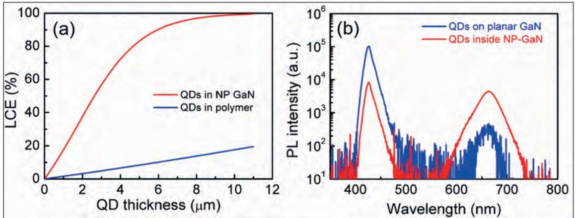
increase in device efficiency. For planar quantum dots in a polymer film, light-conversion efficiency increases linearly with increases in the thickness of the quantum dot layer to a maximum of only 20 percent – that’s for a 10 μm-thick quantum-dot layer (see Figure 3(a)). In stark contrast, when dots fill the nanopores, light-conversion efficiency exceeds 80 percent, for a film thickness of just 5 μm.
