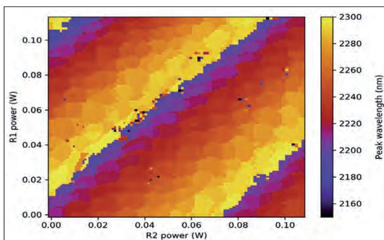
Figure 4. The peak wavelength of Brolis' single widely-swept laser, when both micro-rings are electrothermally tuned in a specific manner. Continuous spectral coverage is clearly visible.
