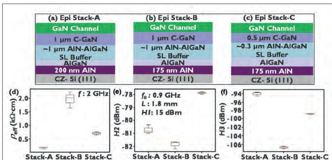
Figure 3. A team from imec considered how the changes to the epitaxial design of the GaN HEMT ((a) to (c)) impact effective resistivity (d) and second- and third-harmonic power ((e) and (f), respectively). The effective resistivity is determined from co-planar waveguides with a centre conductor width of 75 μm and a slot width of 50 μm. Values for the second (H2) and third (H3) harmonic power are measured at a fundamental frequency of 0.9 GHz, and a H1 of 15 dBm, for 1.8 mm-long lines.
