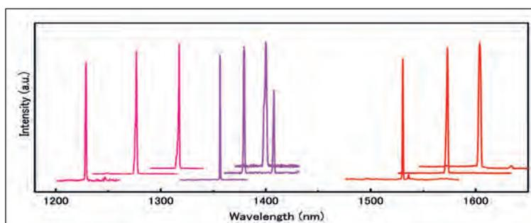
Figure 6. Nanowires allow a tuning of the laser wavelength range in the telecom band. Spectra are offset for clarity. The laser wavelength is modulated by the growth parameters, such as flow rates of the metal-organic sources. Thus a broad wavelength range is covered in the whole telecom band, including the two technologically important telecom-band windows centred around 1.3  $\mu\text{m}$  and 1.55  $\mu\text{m}$ .
