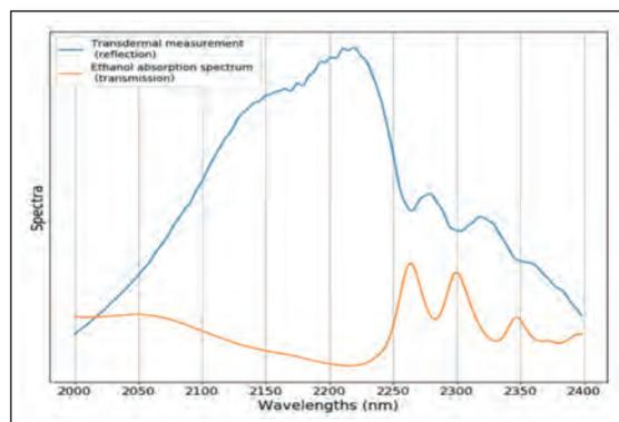
Figure 6. Transdermal optical signal of a tissue matrix containing ethanol, measured in reflection geometry (blue line) and ethanol absorption spectrum (orange). Characteristic ethanol absorption dips are clearly visible in the transdermal signal.
