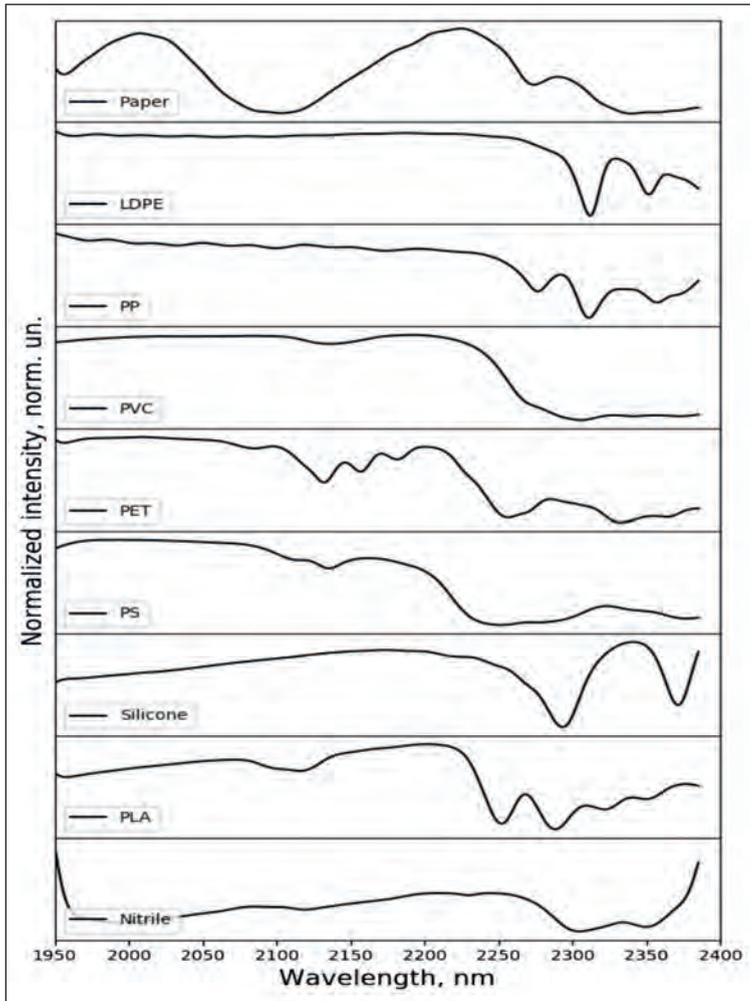
Figure 7. Sorting different types of plastic can draw on the transmission spectra of different materials.
