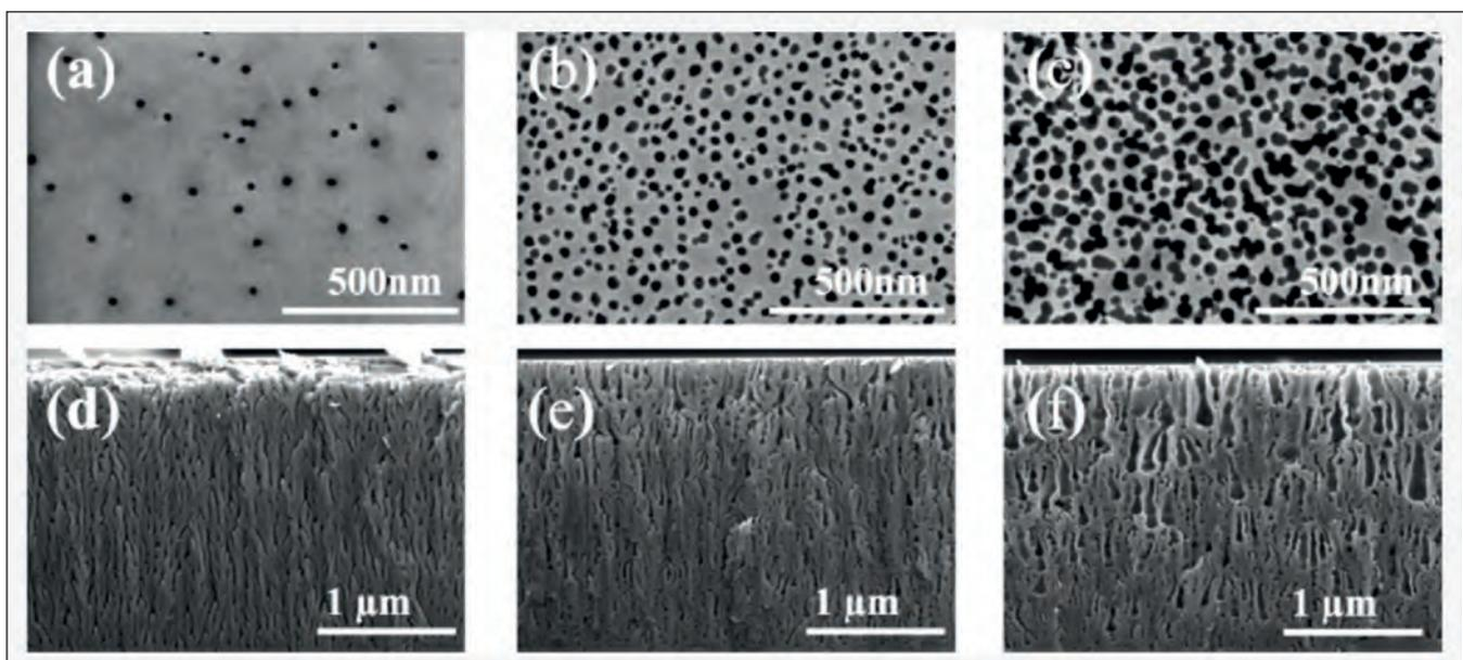
Figure 2. (a-c) Top-view and (d-f) cross-sectional scanning-electron microscopy images of nano-porous GaN with different porosity etched at different bias voltages. Reprinted with the permission of the American Society Chemistry.
