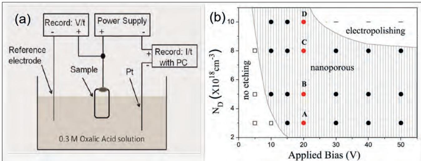
Figure 1. (a) An electrochemical etching process produces nano-porous GaN. (b) A phase diagram of the GaN electrochemical etching process shows how the etching characteristics are related to silicon doping in GaN and the applied bias.
