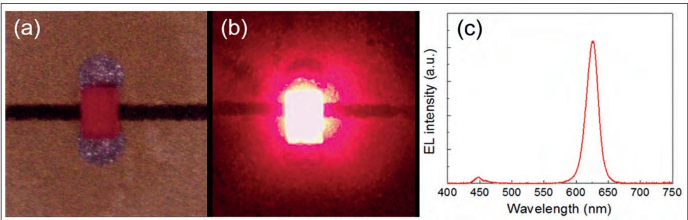
Figure 7. Photos of  $100 \times 150 \mu\text{m}^2$  red nano-porous quantum dot miniLED mounted on a PCB board (a) and lit-up at an injection current of 1 mA (b). (c) Spectrum of a red nano-porous quantum dot LED shown in (b). Testing the reliability of the red nano-porous quantum-dot miniLED revealed acceptable results at  $30 \text{ W cm}^{-2}$ . This power density is more than sufficient for most microLED applications.
