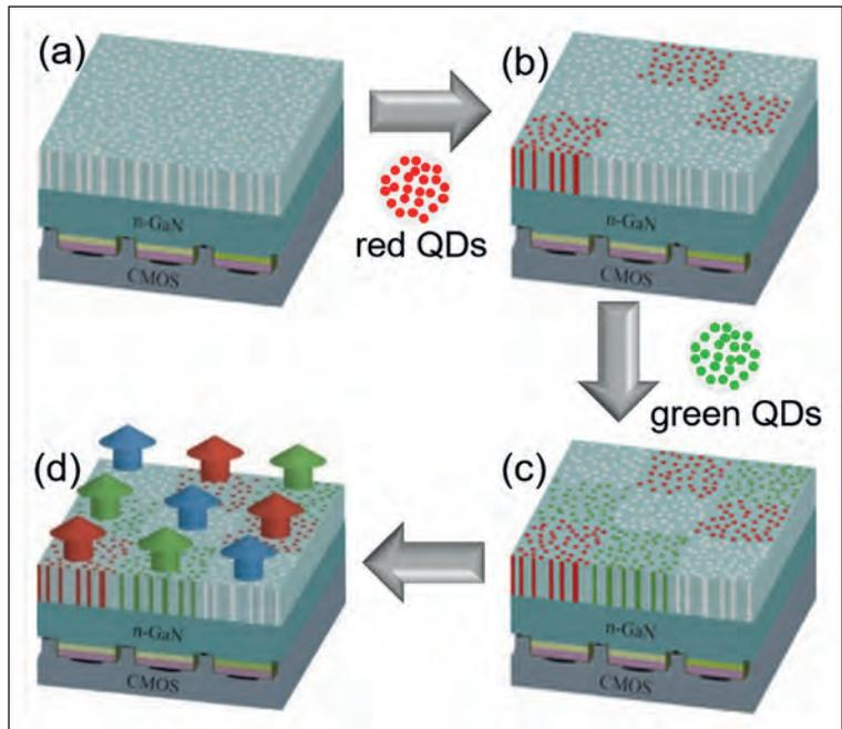
Figure 5. Saphlux's approach to making monolithic RGB microLEDs. (a) A vertical blue LED with exposed nano-porous GaN is bonded to a current-driver panel. (b) Red quantum dots are selectively loaded into red zones. (c) Green quantum dots are selectively loaded into green zones. (d) Red, green and blue light emitted from red quantum dot zones, green quantum dots zones, and zones without any quantum dots, respectively.
