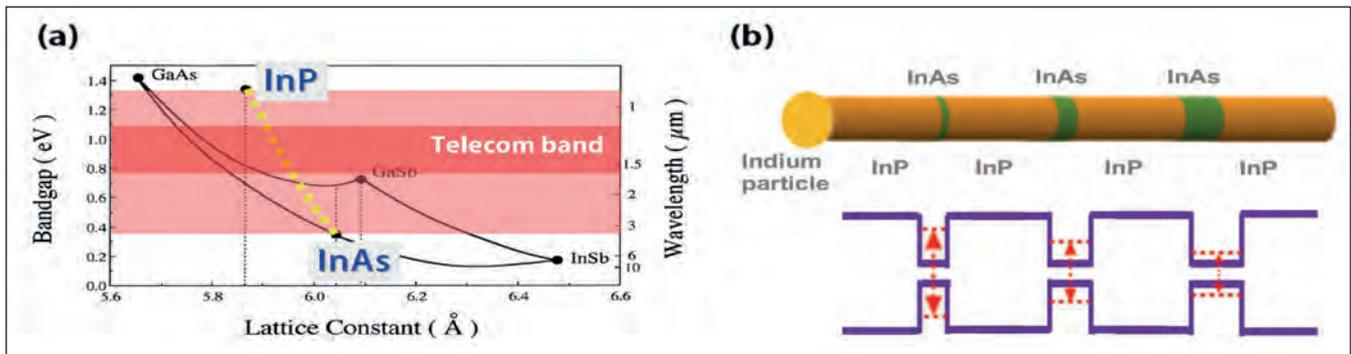
Figure 1. (a) Bandgap and lattice constant of III-V compound semiconductors. InP/InAs can cover a wide spectral range, including the telecom band. (b) Lattice-matching constraints are far less severe in InP/InAs heterostructure nanowires connected by a single indium particle, than in conventional heterostructures. In these nanowires, the quantum confinement effect along the axial direction allows the real bandgap of the InAs layer to be modulated by the thickness.
