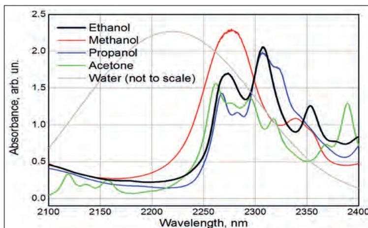
Figure 1. Infrared spectroscopy can identify ethanol, methanol, propanol and acetone by their unique absorbance spectra. The light grey line shows superimposed water transmission spectra.
