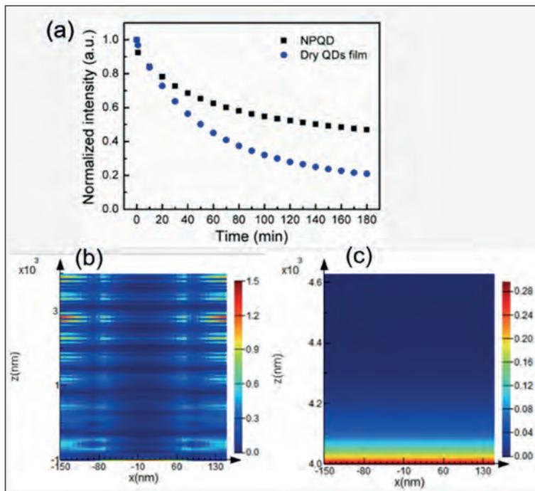
Figure 4. (a) Comparison of the normalized power intensity of red emission from a red nano-porous quantum-dot sample and a quantum-dot film on a GaN-on-sapphire wafer. Both samples were subjected to 3 hours of excitation with a 420 nm blue laser. (b) Simulated mapping results of blue light absorption by nano-porous GaN. (c) Simulated mapping results of blue light absorption by a nano-porous film.
