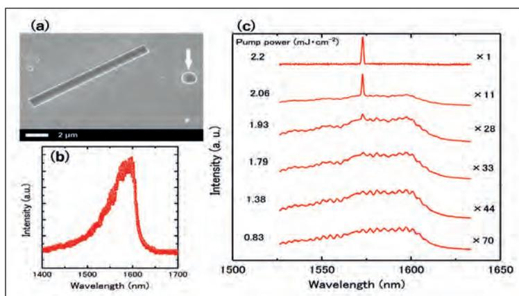
Figure 5. (a) Scanning electron microscopy image of a nanowire mechanically dispersed onto a gold-film-covered  $\text{SiO}_2$ -on-silicon substrate. The white arrow indicates a removed indium particle. (b) Photoluminescence spectrum of a single nanowire under a pump laser power of 0.83  $\text{mJ cm}^{-2}$ . (c) Photoluminescence spectra of the nanowire with increasing pump power, revealing spectral narrowing.
