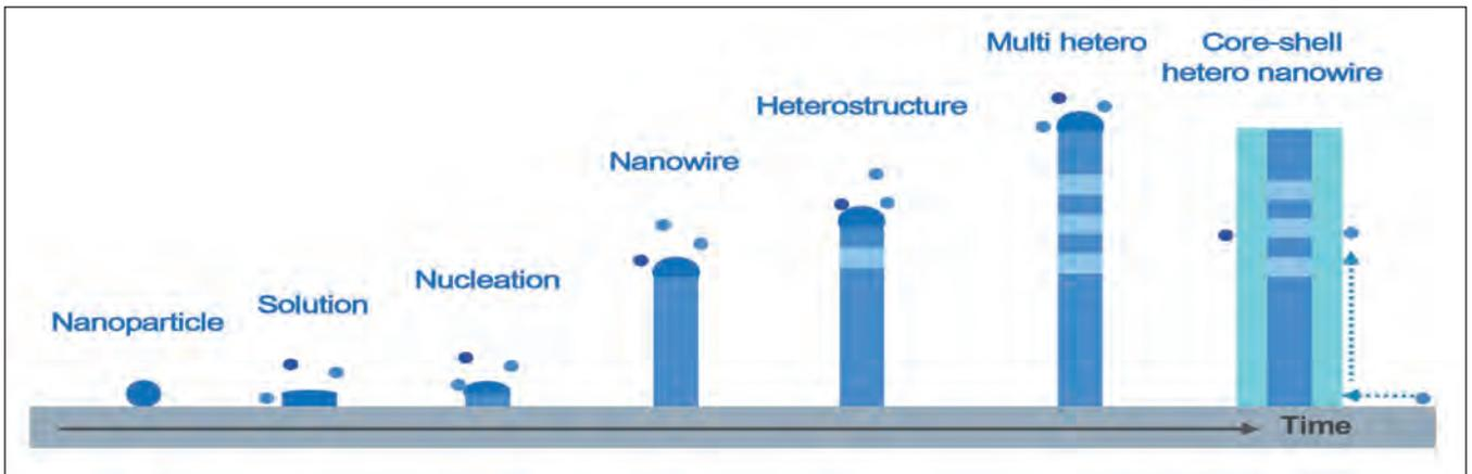
Figure 3. Schematic diagram of the vapour-liquid-solid growth mode. InAs and InP nanowires can be grown by the self-catalysed vapour-liquid-solid mode using indium particles.
