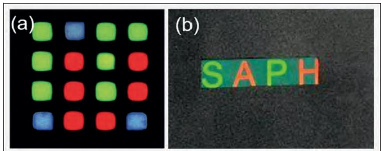
Figure 6. (a) Saphlux RGB monolithic microLEDs excited by a blue LED source from the backside. (b) A picture of the company logo "SAPHLUX" fabricated by red and green nano-porous quantum-dot microLEDs.
