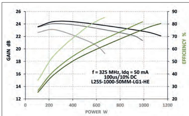
Figure 2. Measured RF power gain and drain efficiency versus output power for a 50 mm die with a signal of 100  $\mu$ s pulse width and 10 percent duty cycle at 325 MHz. The device is characterized at 100 V, 125 V and 145 V DC bias demonstrating a 3 dB power dynamic range. By reducing operating bias to 50 V a 6 dB dynamic range is achieved.
