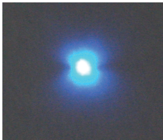
Light emission from an experimental homojunction ZnO LED. The central most luminous region appears white due to over-exposure.
