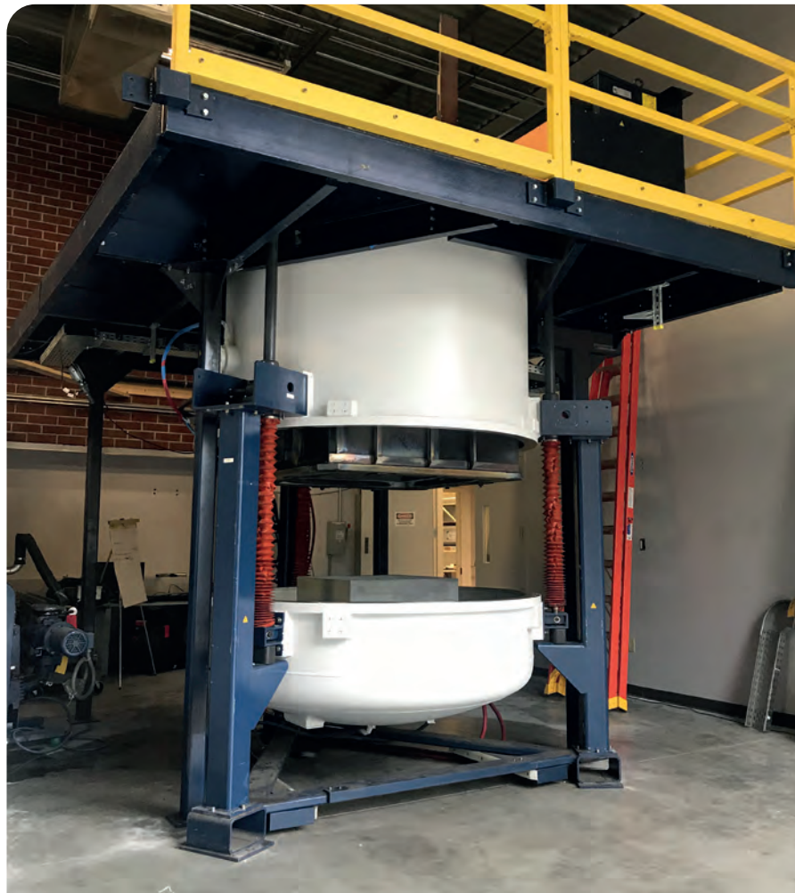
► Figure 1: Photograph of one of Antora's prototype thermal storage systems. With a capacity of 500 kWh, this system has been used to demonstrate the core functionality of the technology.
