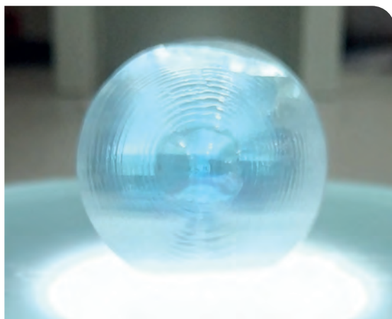
► A view, from the bottom, of a crystal of (\text{Al}_x\text{Ga}_{1-x})_2\text{O}_3 produced by the Czochralski method.
