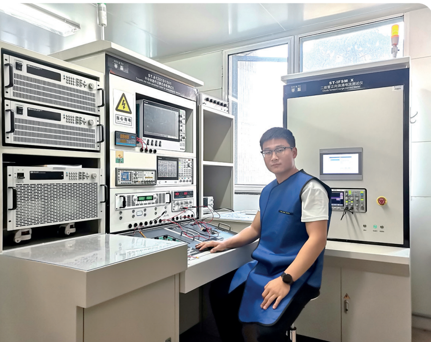
► Figure 4. The team led by Hai Lu at Nanjing University has developed a high-speed, high-reliability dynamic test system to characterize the dynamic performance of power devices based on wide-bandgap semiconductors.
