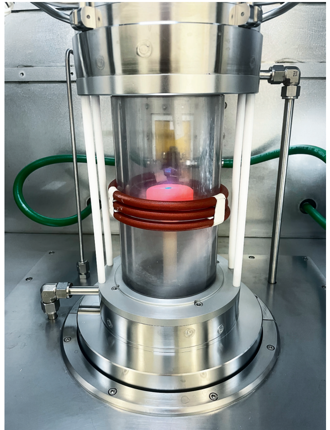
► Figure 5. The Agnitrion Agilis 100 and Mini MOCVD systems offer maximum flexibility with their ability to feature both remote injection and close injection showerhead flanges, enabling users to quickly and easily switch between the two options to optimise their processes. Furthermore, the close injection showerhead flanges are designed with multiple preset distances from the wafer to increase experiment flexibility. The blue light is for optical reflectometer for in-situ monitoring of the films growth rate.
