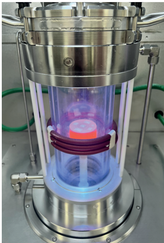
► Figure 5. The Agnitrion Agilis 100 and Mini MOCVD systems offer maximum flexibility with their ability to feature both remote injection and close injection showerhead flanges, enabling users to quickly and easily switch between the two options to optimise their processes. Furthermore, the close injection showerhead flanges are designed with multiple preset distances from the wafer to increase experiment flexibility. The blue light is for optical reflectometer for in-situ monitoring of the films growth rate.
