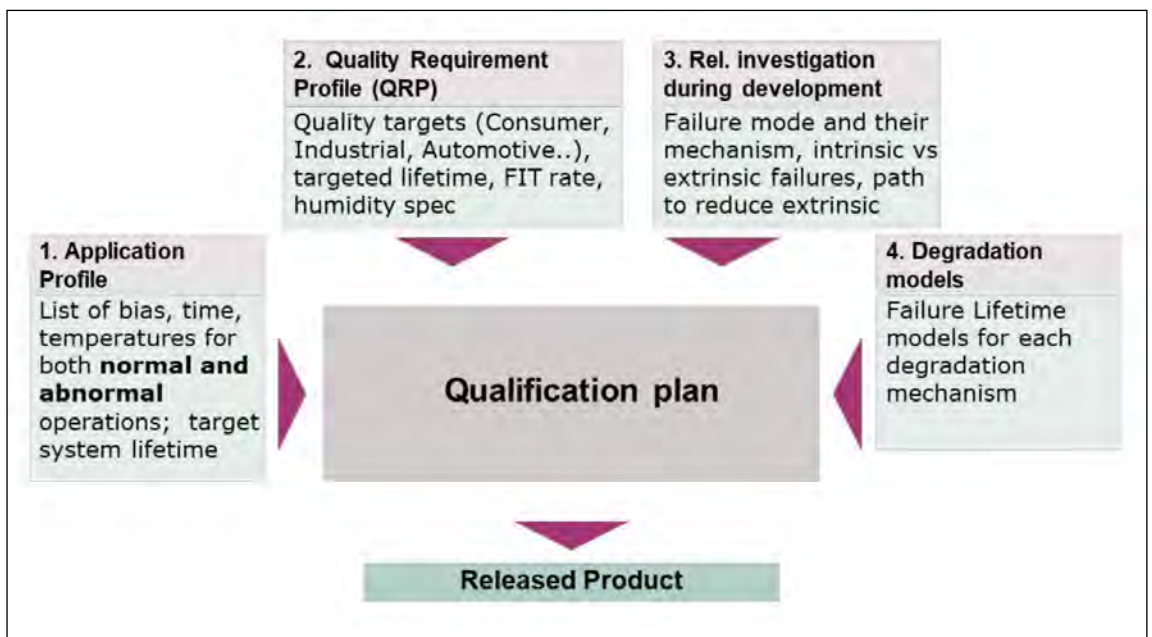
➤ Figure 5. Qualification methodology depicting the main four inputs that drive product release at Infineon Technologies.
