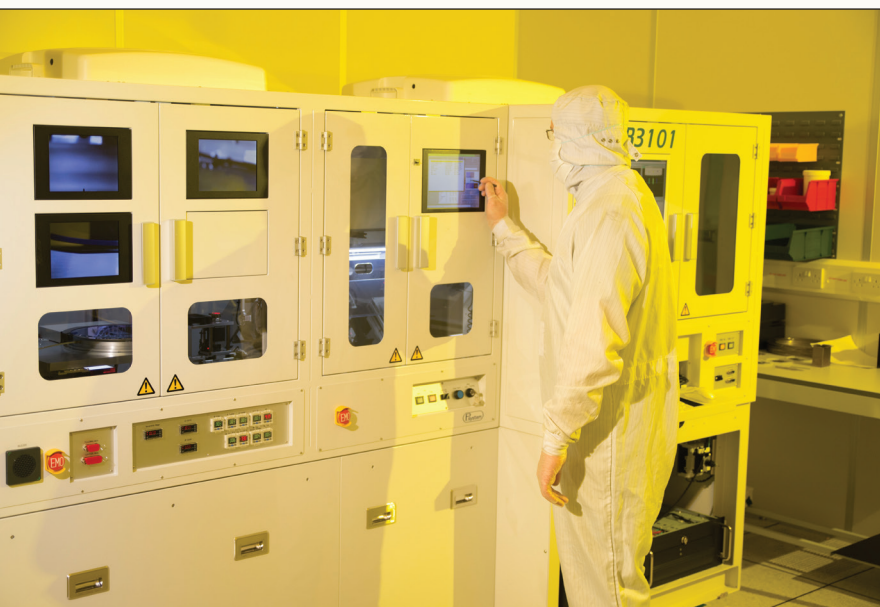
A dedicated tool for bar stacking is helping to increase the throughput at CST Global.
