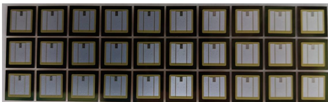
➤ Figure 4. 10kV die ready for packaging.
