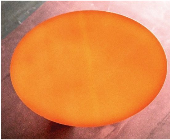
➤ Figure 5. 200 mm silicon wafer heated above 800°C in less than 10 s using less than 20 kW.
