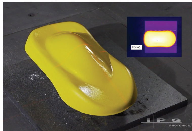
► Figure 4. Lasers cure or dry paint ten times faster than conventional ovens because they selectively heat coatings with high energy fluence governed by agile closed-loop temperature control.
