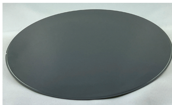
➤ Figure 3. Example of a 200 µm (ø196 mm) n -type 4H-SiC (4° offcut) CS-PVT layer on a 200 mm seed wafer.
