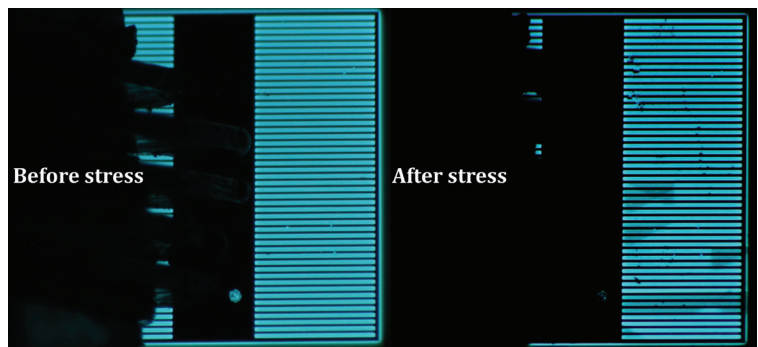
► Figure 5. Electroluminescence images for diodes before (left) and after (right) electrical stress tests without high-energy ion implantation. After electrical stress tests, triangle and bar shape dark regions appear.
