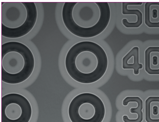
► Figure 4. Microscope image showing oxidation calibration mesas after oxidation, with the central dark spot identifying the aperture (unoxidised region).
