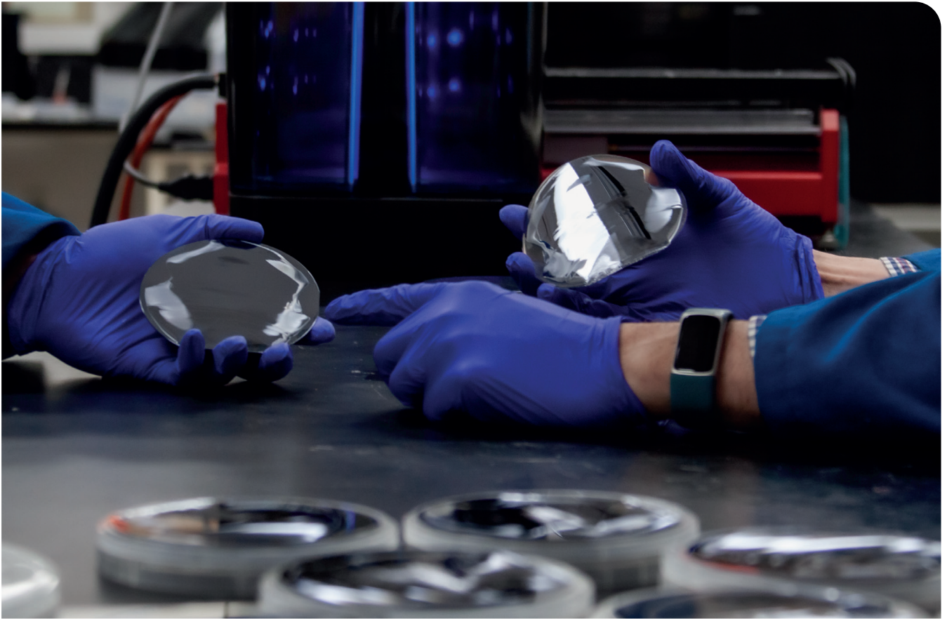
➤ Figure 2. 4-inch GaAs wafers split by Sonic Lift-off, at Crystal Sonic laboratories in Phoenix, Arizona.
