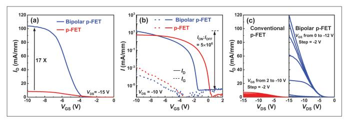
> Figure 3. (a) Linear-scale transfer, (b) log-scale transfer and gate leakage current, and (c) output characteristics of BiPFETs compared with conventional p-FETs.
