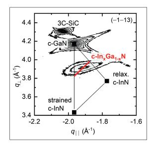
> Figure 2. X-ray diffraction of the asymmetric  $(\overline{1}\overline{1}3)$  reflection of c-GaN. The reciprocal space map reveals a pure cubic phase and a single, partially strained  $c-In_{0.47}Ga_{0.53}N$ layer.
