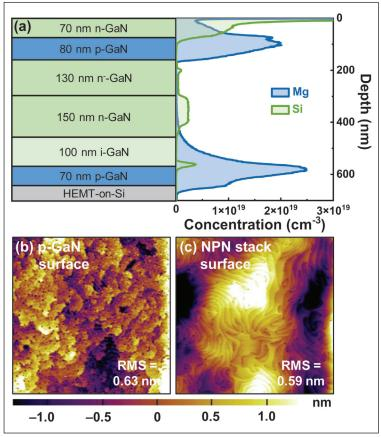
Figure 2. (a) An n-p-n epi-structure on the conventional p-GaN HEMT platform and a secondary ion mass spectrometry depth profile of magnesium and silicon dopants. Atomic force microscopy images of the (b) initial p-GaN surface and (c) GaN surface after n-p-n stack growth on the E-mode GaN HEMT platform.
