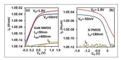
> Figure 6. The current-voltage (I-V) characteristics of (a) GaN transistor, and a (b) silicon PMOS transistor produced by the DrGaN process.
