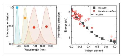
> Figure 3. Normalised low-temperature photoluminescence spectra of c-In $_x$ Ga $_{1-x}$ N with values for x ranging from 0.1 to 0.5. The spectrally integrated intensity is shown as dots (left). Peak emission energy versus indium content, where black squares denote data points of this work and red symbols refer to the emission energies of bulk c-In $_x$ Ga $_{1-x}$ N (right).
