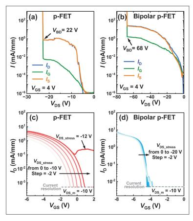
Figure 4. (a) Off-state leakage current and breakdown characteristics of (a) the conventional p-FET and (b) bipolar p-FET. Plots of pulsed drain current as a function of gate-source voltage ( $I_D$ - $V_{GS}$ ) of (c) the p-FET and (d) the BiPFET measured with various drain-source stress voltages ( $V_{DS \ stress}$ ).
