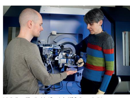
➤ In the X-ray diffraction lab at Fraunhofer IAF, Freiburg, scientists Mario Prescher and Nadine Brückner meticulously analyse the crystallographic structure of AlYN layers, providing essential data for optimising material quality and understanding its relationship with underlying GaN layers.
