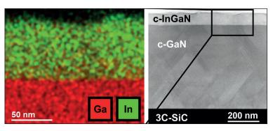
➤ Figure 4. Characteristic energy-dispersive X-ray spectrometry (left) and scanning transmission electron microscopy (right) of a c-In<sub>0.47</sub>Ga<sub>0.53</sub>N sample. The cross section of energy-dispersive X-ray spectrometry shows a very homogeneous distribution of the elements gallium (red) and indium (green). This is a noteworthy finding, as a sample with this indium content lies at the heart of the often literature-perceived miscibility gap.
