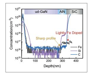
> Figure 2. Secondary ion mass spectrometry provides profiles of the iron, silicon and carbon elements in GaN/AlN/ SiC heterostructures.
