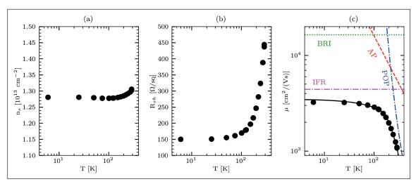
> Figure 1. Temperature-dependent Hall measurement of the  $Al_{1-x}Y_xN/GaN$  heterostructure with a value for x of 0.082. (a) Electron density ( $n_s$ ), (b) sheet resistance ( $R_{sh}$ ) and (c) mobility ( $\mu$ ). Calculated background residual impurity scattering (BRI), interface roughness scattering (IFR), acoustic phonon scattering (AP) and polar optical phonon scattering (POP) limited mobilities are indicated.
