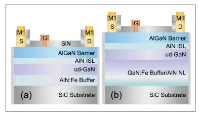
> Figure 1. Improvements in RF performance are realised by introducing an iron-doped AlN buffer (a). This design is superior to the conventional iron-doped GaN heterostructure (b). Note that these illustrations are not to scale.
