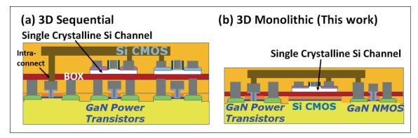
Figure 4. (a) Intel's prior work involved the three-dimensional sequential monolithic integration of GaN and silicon CMOS by a layer transfer process, with silicon PMOS/NMOS transistors fabricated after completing fabrication of the GaN transistors. (b) For Intel's latest work, DrGaN technology, GaN and silicon PMOS/NMOS transistors are fabricated in such a way that the high-temperature activation steps are completed before the deposition of the gate dielectric of the GaN transistors.
