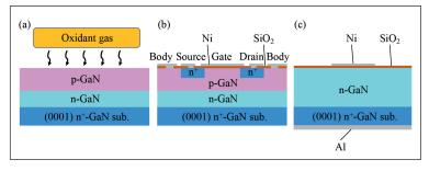
> The researchers from Mirise **Technologies** and Kochi University of Technology produced: (a), an epitaxial layer for oxidation evaluation; (b), a lateral MOSFET for determining channel mobility; and (c), an *n*-type MOS capacitor for finding the density of interface states.
