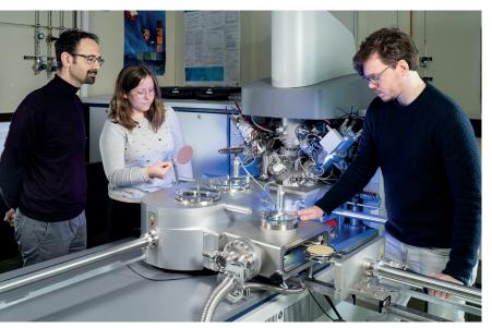
➤ The time-of-flight secondary ion mass spectrometry tool operated by Patrik Straňák provides invaluable insights into the composition of AlYN layers, allowing analysis of interfaces and the detection of impurities.
