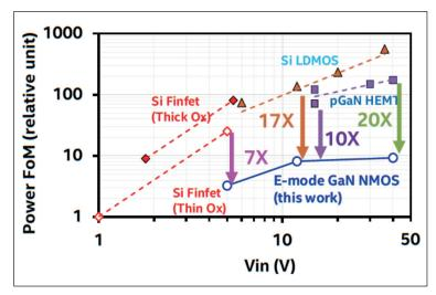
ightharpoonup Figure 2. Benchmarking the power figure-of-merit ( $R_{\rm ON} x Q_{\rm GG}$ ) of the GaN transistor of this work shows: a performance that's around a 20-fold better than the  $p{\rm GaN}$  HEMT and around a 30-fold better than silicon LDMOS at 40 V; a 10-17-fold better performance than silicon LDMOS and a  $p{\rm GaN}$  HEMT at 12-15 V, and 7-fold better performance than a silicon finFET at 5 V.
