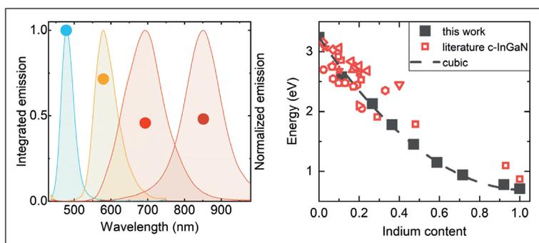
► Figure 3. Normalised low-temperature photoluminescence spectra of  $\text{c-In}_x\text{Ga}_{1-x}\text{N}$  with values for  $x$  ranging from 0.1 to 0.5. The spectrally integrated intensity is shown as dots (left). Peak emission energy versus indium content, where black squares denote data points of this work and red symbols refer to the emission energies of bulk  $\text{c-In}_x\text{Ga}_{1-x}\text{N}$  (right).
