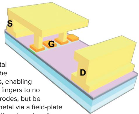
➤ Fabrication of radiation-hard HEMTs involves removal of the *p*-GaN layer in the non-gate region and source-connected buried metal region, followed by deposition of a Ti/Al/TiN metal stack in the patterned source and drain region, as well as the source-connected buried metal region.
