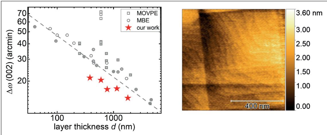
► Figure 1. The quality of material can be evaluated by considering values provided by  $\omega$ -scans, produced by X-ray diffraction. The general trend is a decreasing value for  $\Delta\omega$  with increasing layer thicknesses. Grey squares and circles refer to other c-GaN layers grown by MOCVD and MBE on comparable 3C-SiC substrates (left). An atomic force microscopy image offers insight into surface morphology, uncovering mono-atomic steps across the smooth surface of c-GaN (right).
