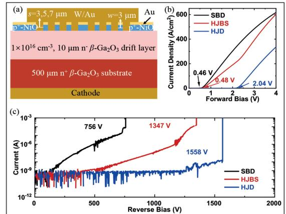
➤ Heterojunction barrier Schottky diodes almost match Schottky diodes for turn-on characteristics, while providing the highest breakdown voltages.
