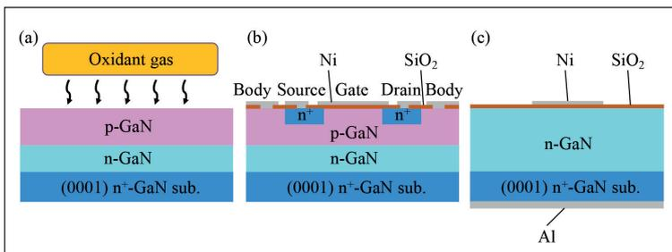
► The researchers from Mirise Technologies and Kochi University of Technology produced: (a), an epitaxial layer for oxidation evaluation; (b), a lateral MOSFET for determining channel mobility; and (c), an *n*-type MOS capacitor for finding the density of interface states.
