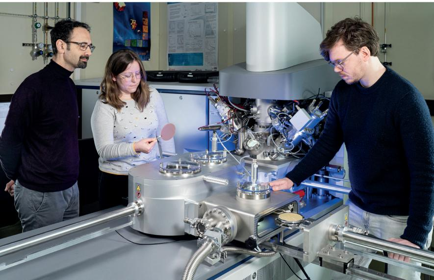
► The time-of-flight secondary ion mass spectrometry tool operated by Patrik Straňák provides invaluable insights into the composition of AlYN layers, allowing analysis of interfaces and the detection of impurities.
