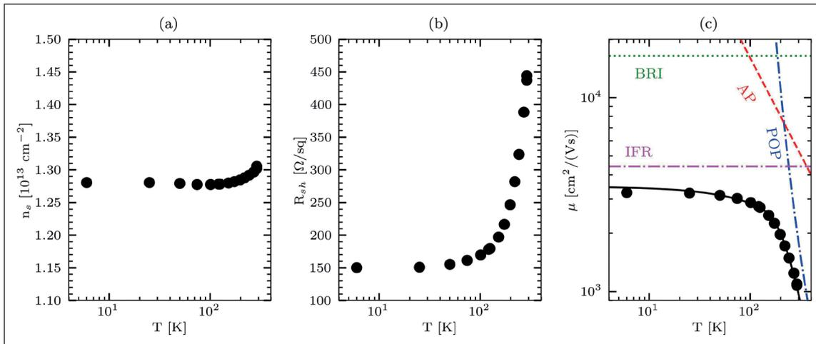
► Figure 1. Temperature-dependent Hall measurement of the  $\text{Al}_{1-x}\text{Y}_x\text{N}/\text{GaN}$  heterostructure with a value for  $x$  of 0.082. (a) Electron density ( $n_s$ ), (b) sheet resistance ( $R_{sh}$ ) and (c) mobility ( $\mu$ ). Calculated background residual impurity scattering (BRI), interface roughness scattering (IFR), acoustic phonon scattering (AP) and polar optical phonon scattering (POP) limited mobilities are indicated.
