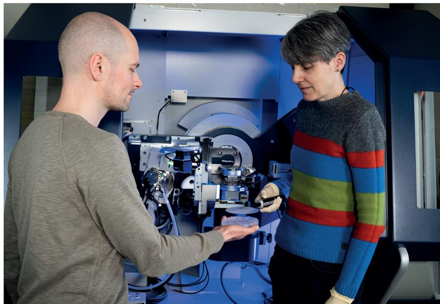
► In the X-ray diffraction lab at Fraunhofer IAF, Freiburg, scientists Mario Prescher and Nadine Brückner meticulously analyse the crystallographic structure of AlYN layers, providing essential data for optimising material quality and understanding its relationship with underlying GaN layers.
