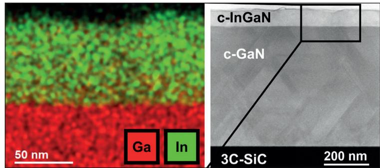
► Figure 4. Characteristic energy-dispersive X-ray spectrometry (left) and scanning transmission electron microscopy (right) of a  $\text{c-In}_{0.47}\text{Ga}_{0.53}\text{N}$  sample. The cross section of energy-dispersive X-ray spectrometry shows a very homogeneous distribution of the elements gallium (red) and indium (green). This is a noteworthy finding, as a sample with this indium content lies at the heart of the often literature-perceived miscibility gap.
