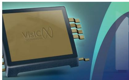
The adoption of the silver sintering process by Pink enhances the thermal and electrical conductivity of the module. Silver sintering is a low-temperature bonding process that creates robust and reliable connections between components, improving the module's overall durability and efficiency. This process is said to be critical for the high reliability required in EV powertrains, where consistent performance is non-negotiable.
