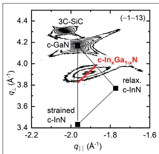
► Figure 2. X-ray diffraction of the asymmetric  $(\bar{1}\bar{1}3)$  reflection of c-GaN. The reciprocal space map reveals a pure cubic phase and a single, partially strained c-In<sub>0.47</sub>Ga<sub>0.53</sub>N layer.
