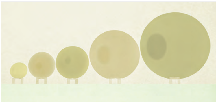
► Figure 4. GTAT's progress in crystal growth from 50 mm to 200 mm.
