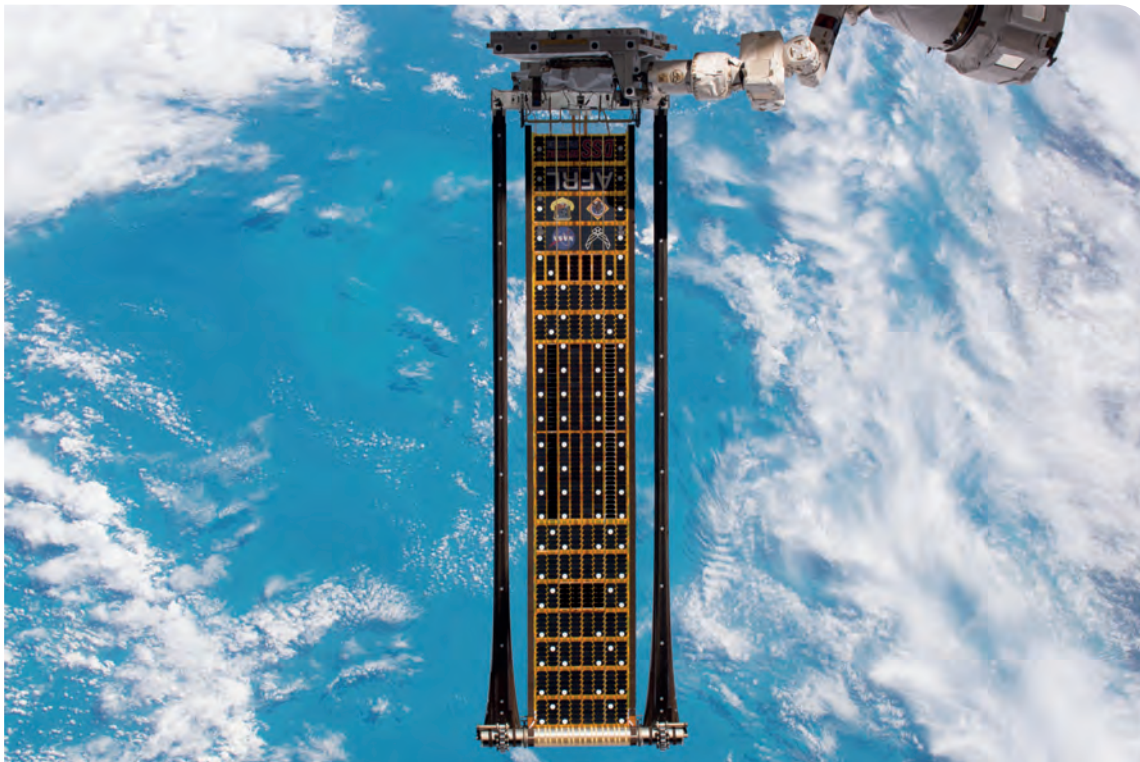
► Flexible solar cells are needed on the ROSA (Roll Out Solar Array) held by the robotic arms at the International Space Station.
