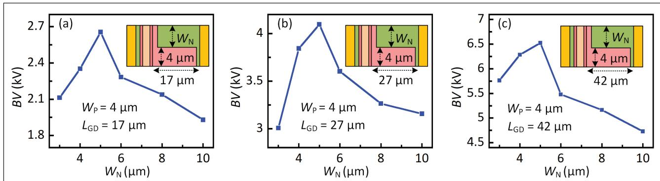
► Figure 2. The measured relationship for the blocking voltage ( $BV$ ) and  $n$ -pillar width ( $W_N$ ) of superjunction HEMTs with different source-to-drain lengths ( $L_{GD}$ ) when the  $p$ -pillar width is fixed at 4  $\mu\text{m}$ . For all source-to-drain lengths, the highest blocking voltage is obtained at  $W_N/W_p = 5/4 \mu\text{m}$ , which is the charge balance point.
