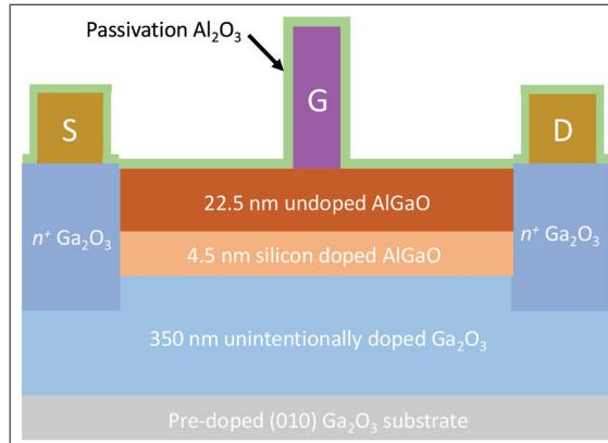
► A relatively thick layer of  $\text{Al}_2\text{O}_3$  passivates the traps in  $\beta\text{-Ga}_2\text{O}_3$  RF devices
