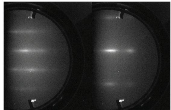
► Figure 10. Reflection high-energy electron diffraction patterns taken in two orientations from the 2D AlScN film with 29 percent scandium.
