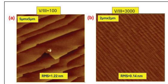
► Figure 2. Atomic force microscopy images of undoped AlN films that are around 1  $\mu\text{m}$ -thick and grown on AlN substrates using RIS MOCVD. TMAI provides the aluminium source, and V/III ratios are (a) 100 and (b) 3000.
