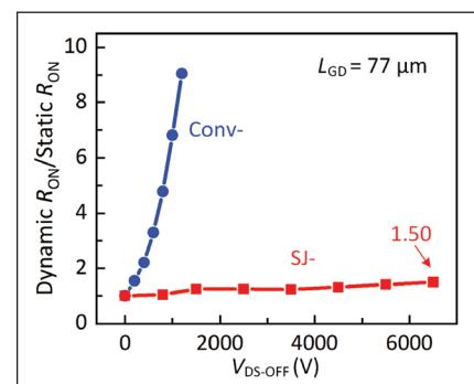
► Figure 4. An ultra-low dynamic on-resistance/static on-resistance ratio of 1.5 is obtained in superjunction HEMT after a 6.5 kV drain stress.
