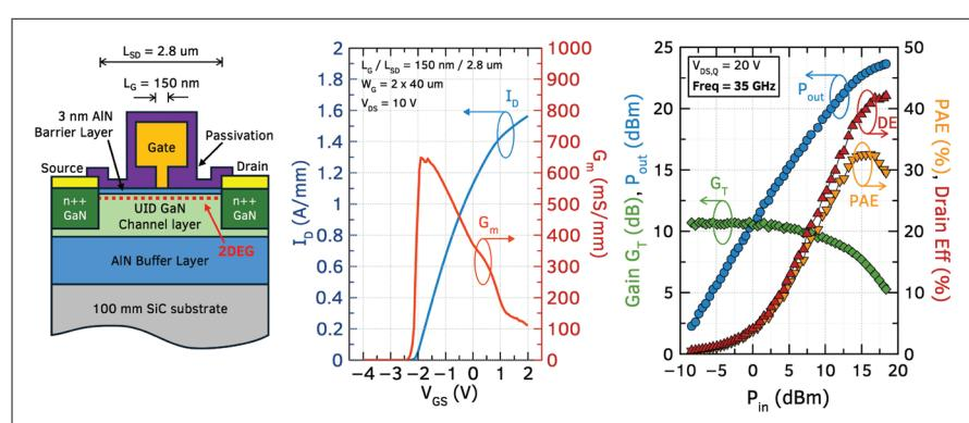
► The Soctera-Qorvo collaboration has evaluated drain currents, transconductance, gain, output power and drain and power-added efficiency of AlN/GaN HEMTs.
