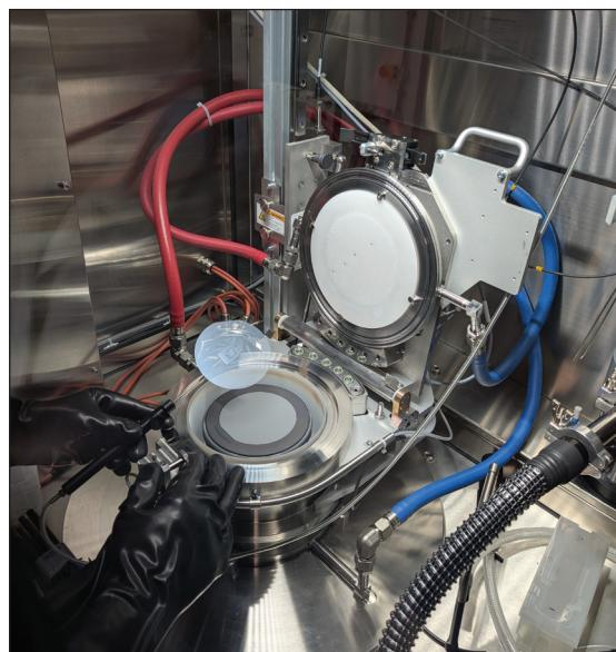
► Recently CISM installed an MOCVD reactor capable of the growth of gallium oxide epilayers on 4-inch substrates.
