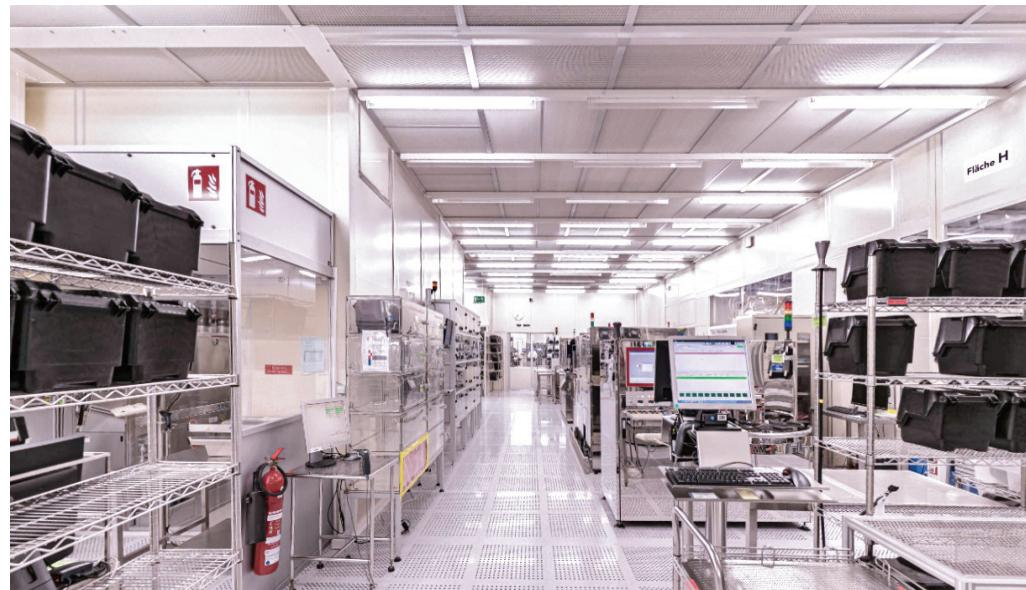
► The 200 mm line at the Dresden Foundry has focused in producing devices using 350 nm CMOS technology, but will soon also provide the production of GaN-based D- and E-mode HEMTs and Schottky barrier diodes.
