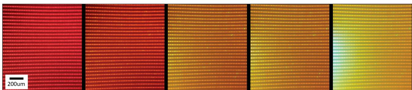
► Prototype panel demonstration of Q-Pixel's proprietary transfer process, using 10 µm tuneable polychromatic microLEDs to produce a display with a pixel density of over 500 pixels per inch. There are no missing pixels, and yield is more than 99.9995 percent.
