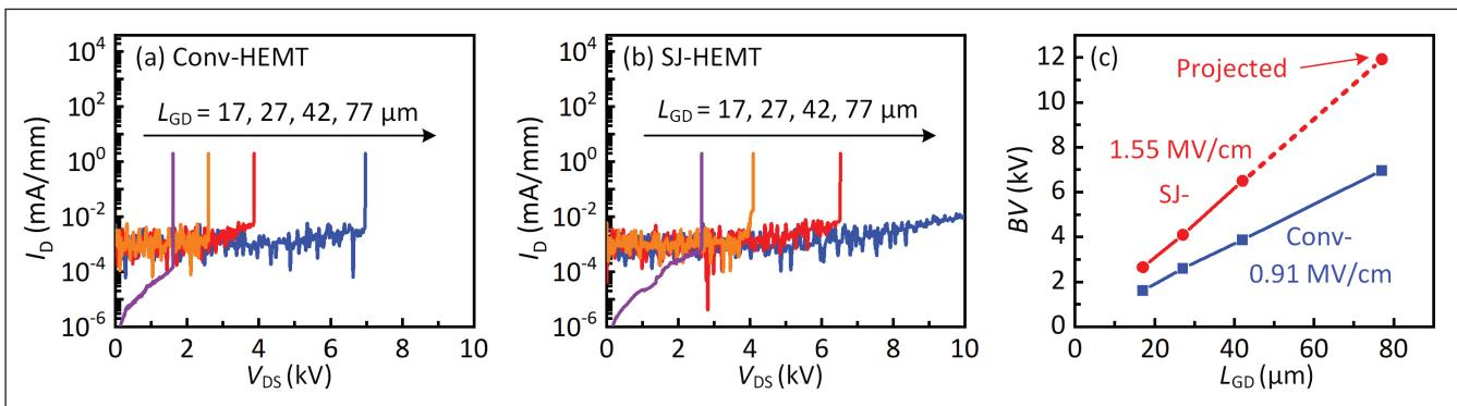
► Figure 3. Off-state current-voltage curves of (a) conventional  $p$ -GaN gate HEMT and (b) superjunction-HEMT with widths of the  $n$ - and  $p$ -pillars ( $W_N/W_P$ ) of 5 μm and 4 μm, respectively. (c) The relationship between blocking voltage ( $BV$ ) and gate-to-drain distance ( $L_{GD}$ ). For the superjunction HEMT with a gate-to-drain distance of 77 μm, the blocking voltage exceeds 10 kV (the measurement limit), and is projected to be 11,935 V by linear extrapolation.
