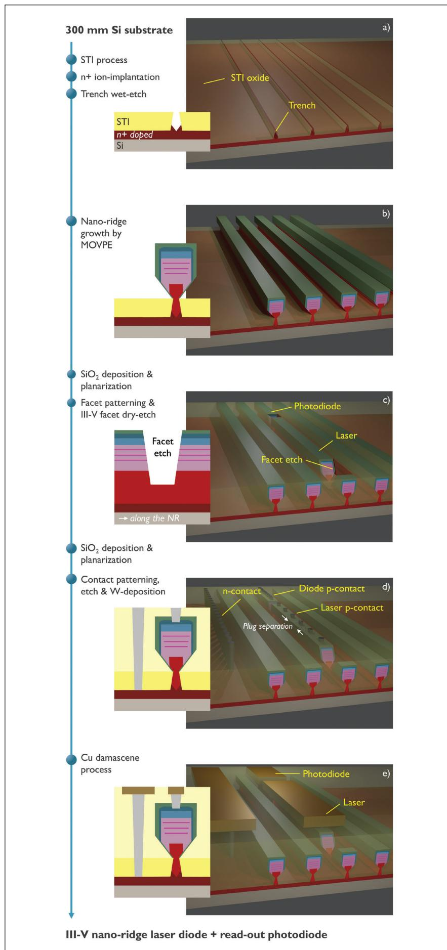
► Figure 2. Simplified schematic of the 300 mm process flow executed in imec's CMOS prototyping line (W: tungsten; Cu: copper). For more details see Y. D. Konick et al. *Nature* **637** 63 (2025)
