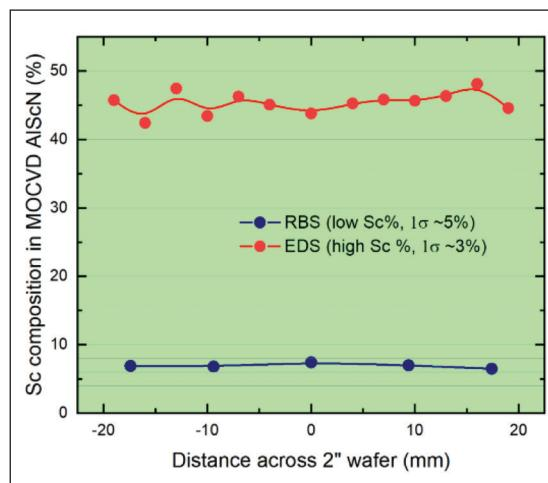
► Figure 7. Scandium composition in MOCVD-grown AlScN. Two representative samples are shown: one with a low scandium content of around 7 percent, measured with Rutherford backscattering spectrometry; and another with a high scandium content of around 45 percent, measured by energy dispersive X-ray spectroscopy. Both samples have a scandium composition variability of less than 5 percent over the diameter of the wafer, demonstrating effective control over scandium incorporation during growth.
