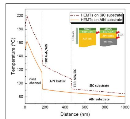
Compared with a SiC substrate, that made from AlN leads to a significant reduction in device temperature.
