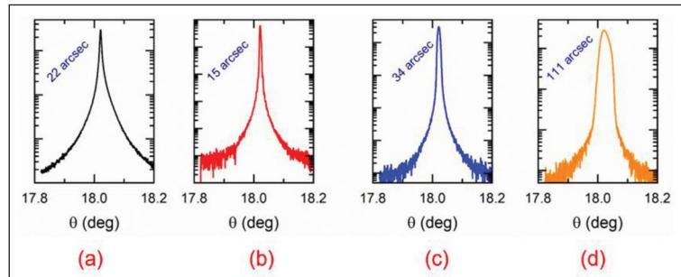
► Figure 3. High-resolution X-ray diffraction rocking curves for the (0002) reflection of AlN films grown on native substrates using the RIS reactor. The layers were grown under varying growth conditions: (a) unintentionally doped AlN layer grown using a V/III ratio of 100, (b) a doped AlN layer grown using a V/III ratio of 100, (c) a doped AlN layer grown using a V/III ratio of 3000, and (d) a doped AlN layer grown using a V/III ratio of 1500.
