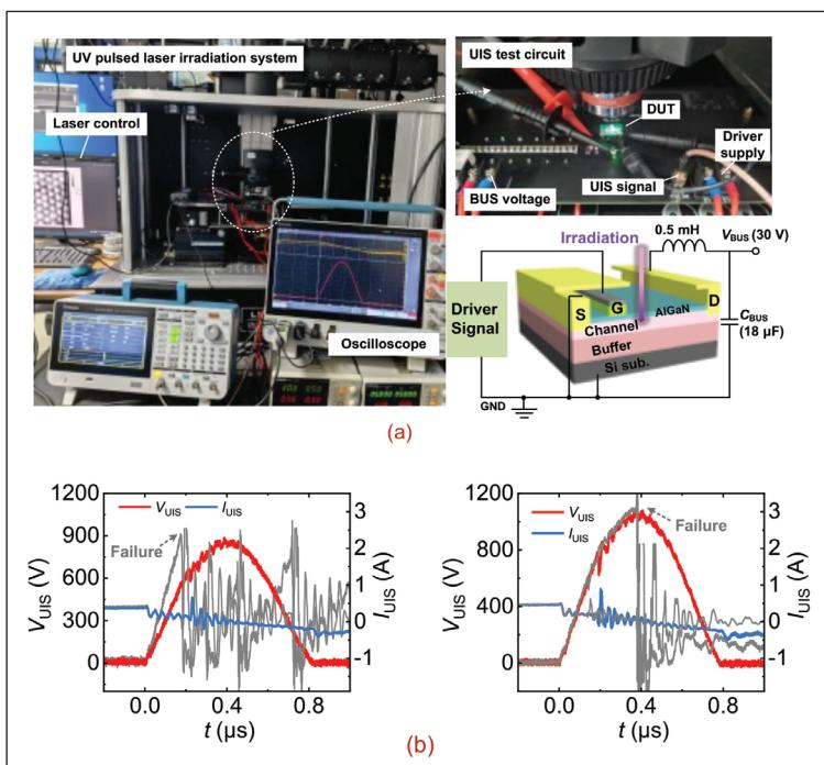
► Figure 4. (a) Un-clamped inductive switching circuit setup in a UV pulse laser irradiation experimental system. (b) Critical un-clamped inductive switching and failure waveforms.
