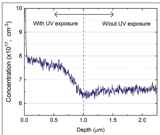
► Figure 6. SIMS depth profiles showing silicon concentration in AlN layers grown using the RIS reactor with and without UV exposure. UV illumination during growth resulted in approximately a 19 percent increase in silicon incorporation compared to the non-UV-exposed region.
