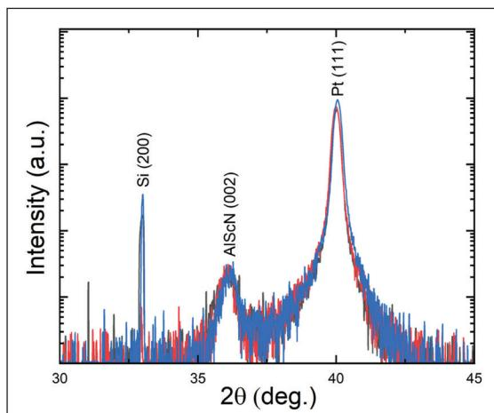
► Figure 9. X-ray diffraction scan ( $2\theta-\omega$ ) of AlScN/Pt/Si. Phase pure wurtzite structure is observed for all three samples.
