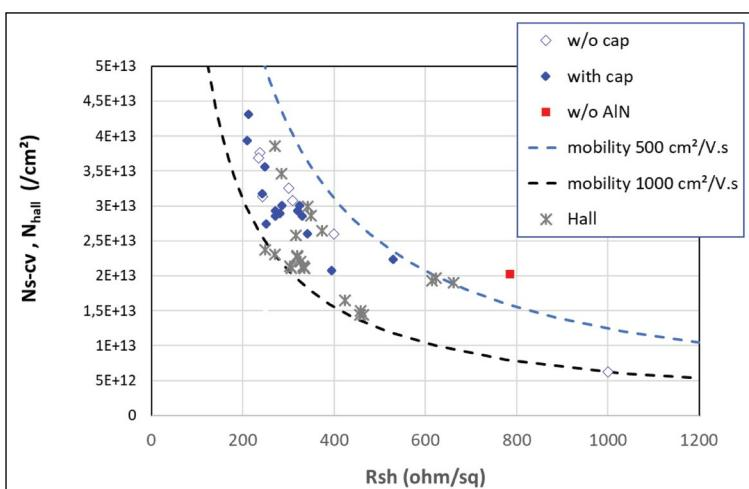
► Figure 4. Transport properties of the 2DEG in a ScAlN-based HEMT grown by ammonia MBE.
