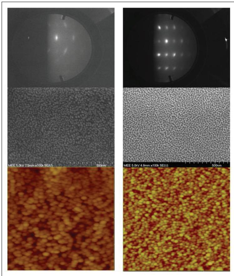
► Figure 8. A reflection high-energy electron diffraction pattern (top), scanning electron microscopy (middle), and atomic force microscopy (bottom) images of AlScN films grown on platinum/TiO<sub>x</sub>/silicon (left) and conductive silicon (right) substrates.
