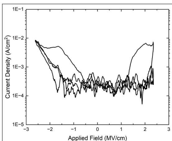
► Figure 12. Current density versus applied electric field for a 75  $\mu\text{m}$ -diameter capacitor of  $\text{AlScN}/\text{Pt}/\text{Si}$ . Ferroelectric looping is observed at each end of the curve.
