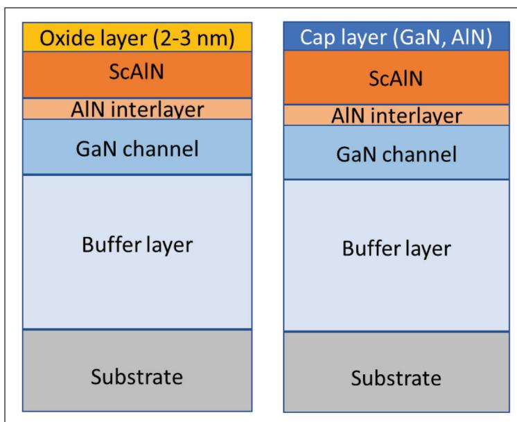
► Figure 1. Schematic cross-section of the first (left) and second (right) generation HEMTs studied at CRHEA.
