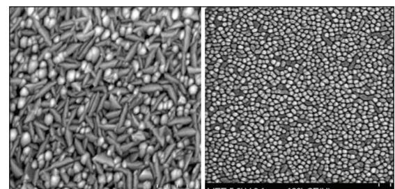
► Figure 11. High-resolution scanning electron microscopy images of AlScN on Pt/Si, displaying growth of a blend of oriented and misoriented grains (a) and fully oriented grains (b).
